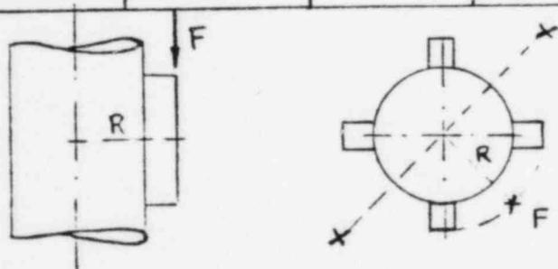
XX - NEUTRAL AXIS OF BENDING DUE TO THE FORCE F.
