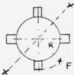
XX - NEUTRAL AXIS OF BENDING DUE TO THE FORCE F.
