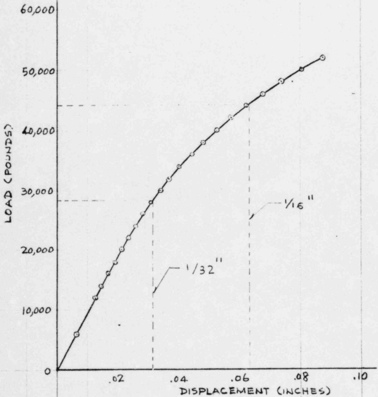
Fig. 11 LOAD-DISPLACEMENT CURVE OF GRID POINT 148
