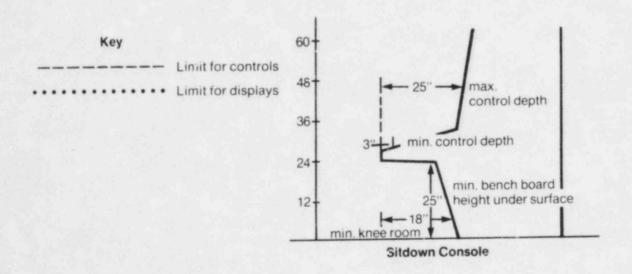
Figure AS-1. Anthropometric Criteria For Benchboards, Vertical Boards, and Sitdown Consoles
