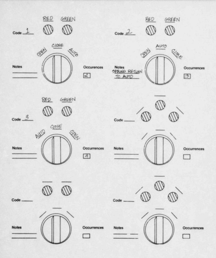
Figure DCS-4. Sample/Design Convention Worksheet For Three-Position Rotary Selections
