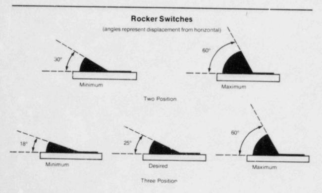
Figure G-1. (Illustrating Item G-15) Switch Displacements
