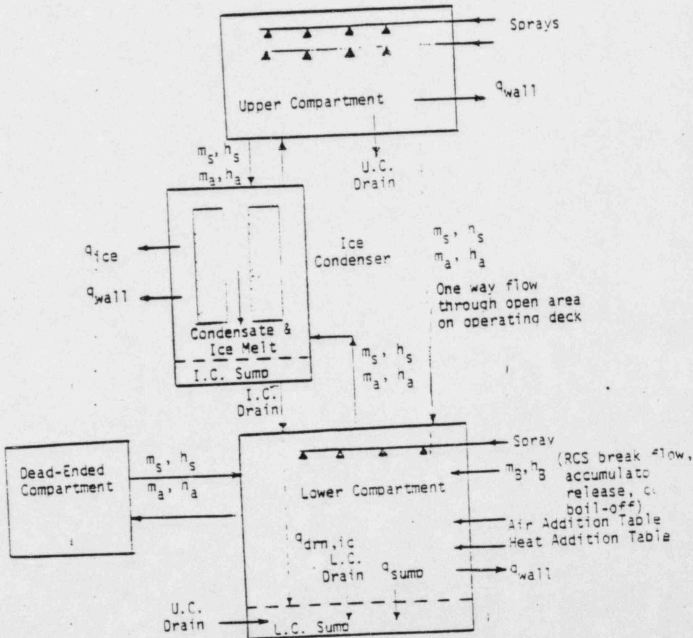
FIGURE 3.3 MASS AND ENERGY FLOW DIAGRAM FOR THE COMPARTMENTS
