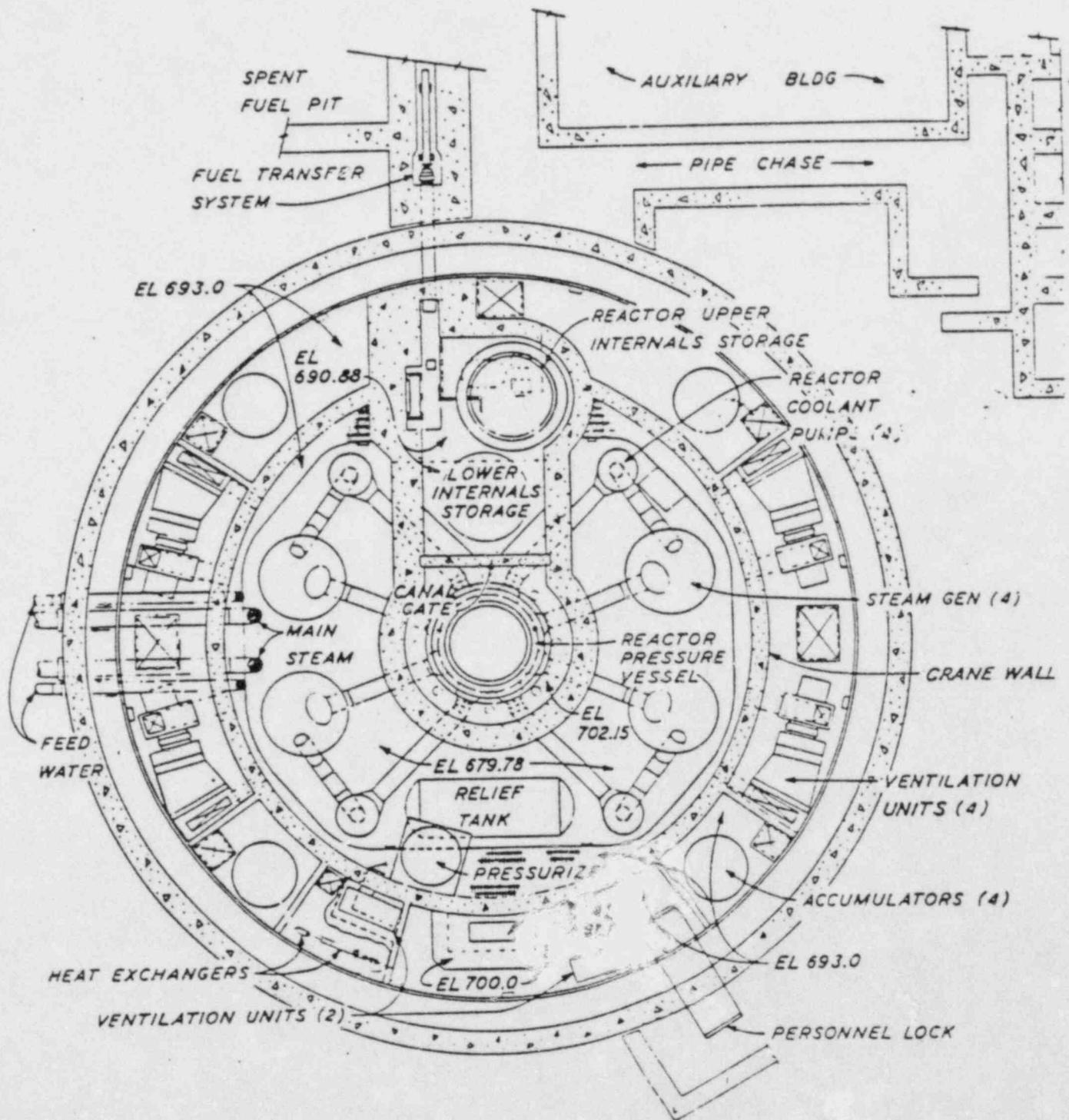
Figure 3.8.3-7 Plan-Lower Compartment
