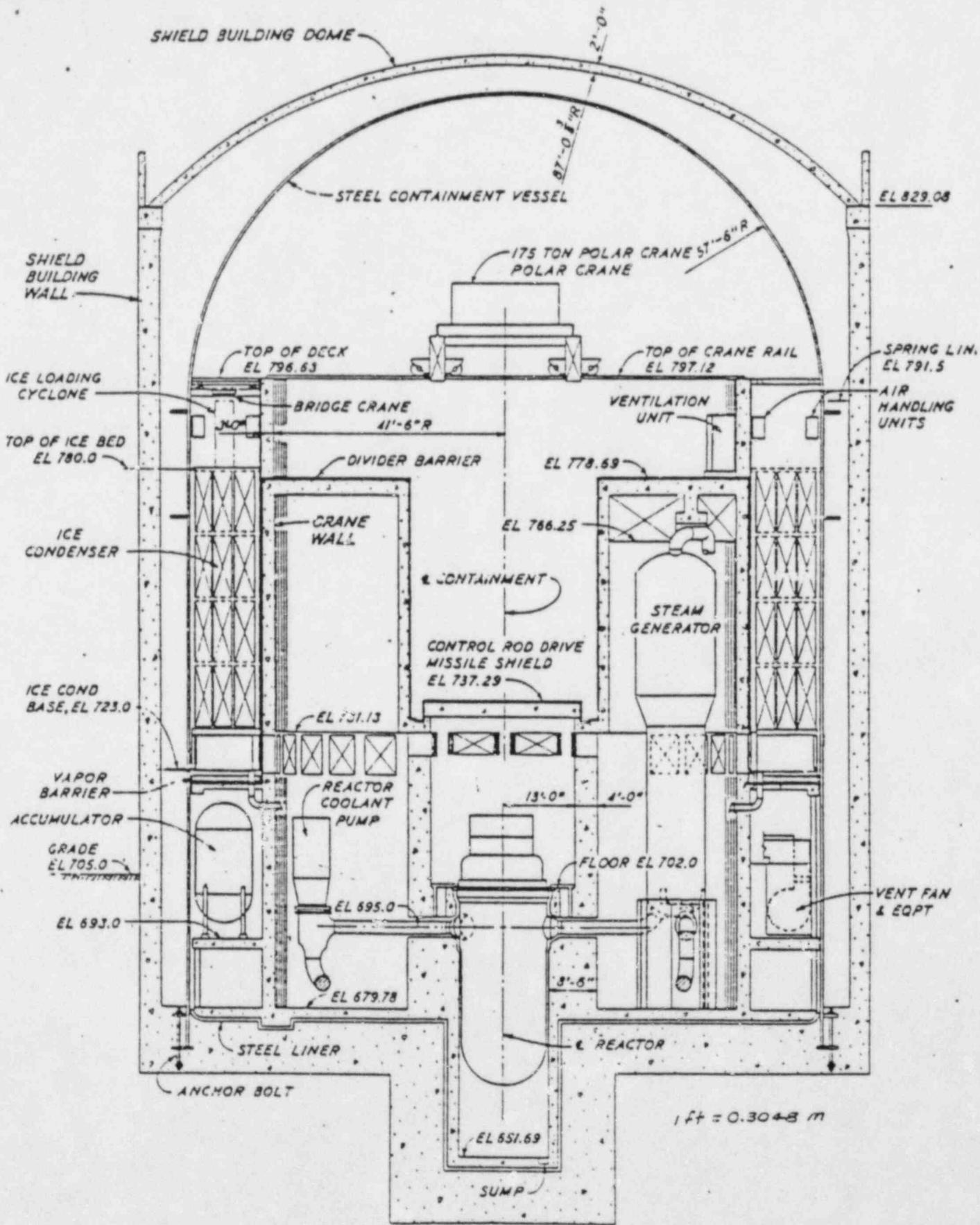
Reactor Building Elevation
