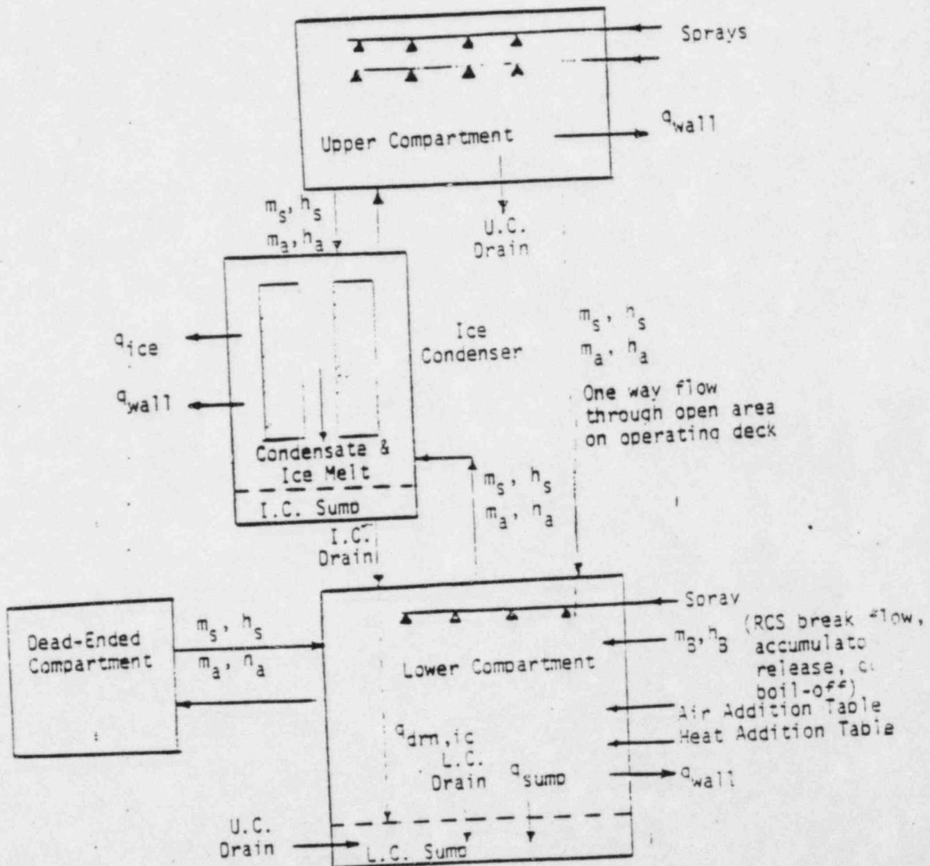
FIGURE 3.3 MASS AND ENERGY FLOW DIAGRAM FOR THE COMPARTMENTS
