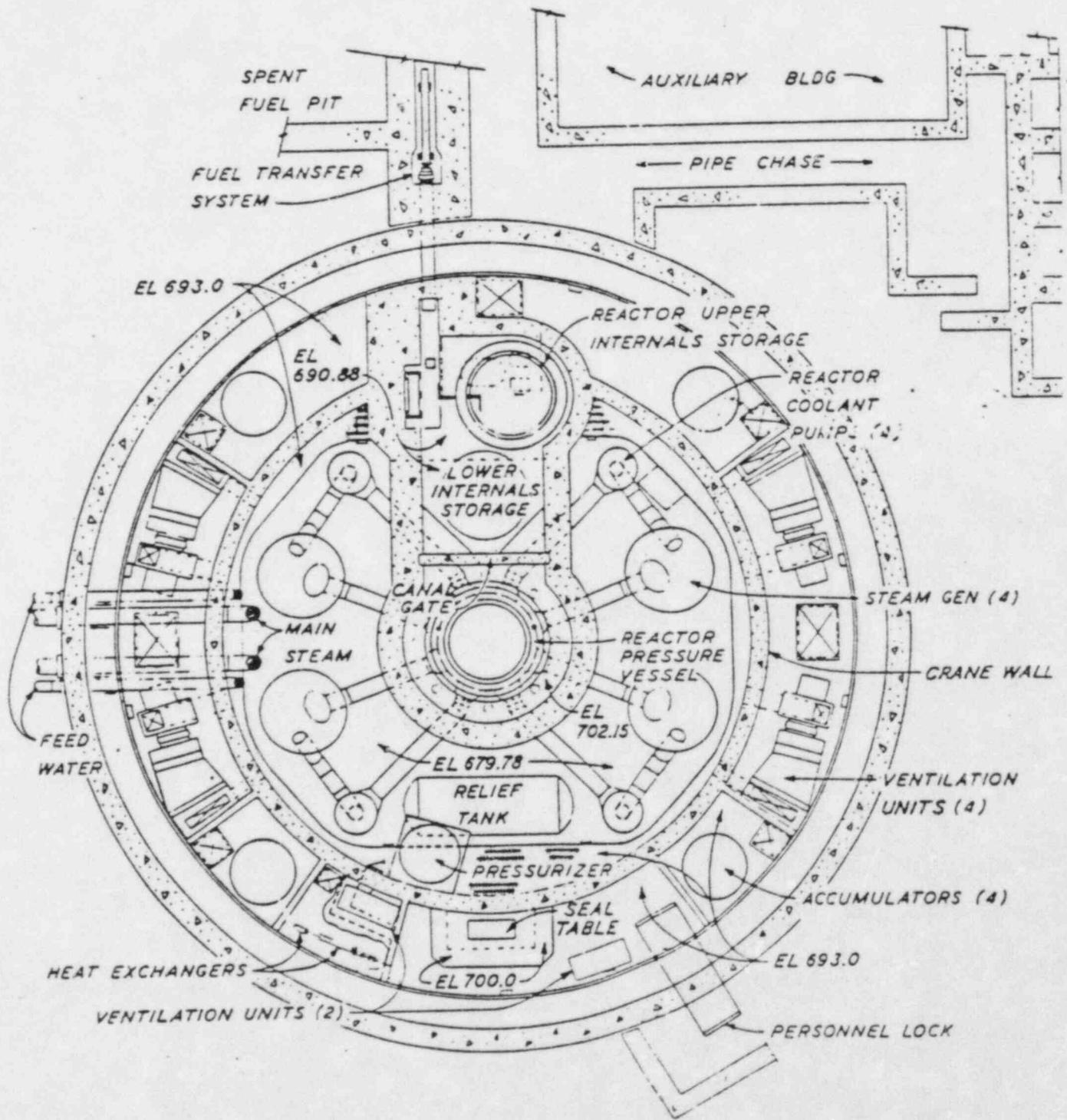
Figure 3.8.3-7 Plan-Lower Compartment
