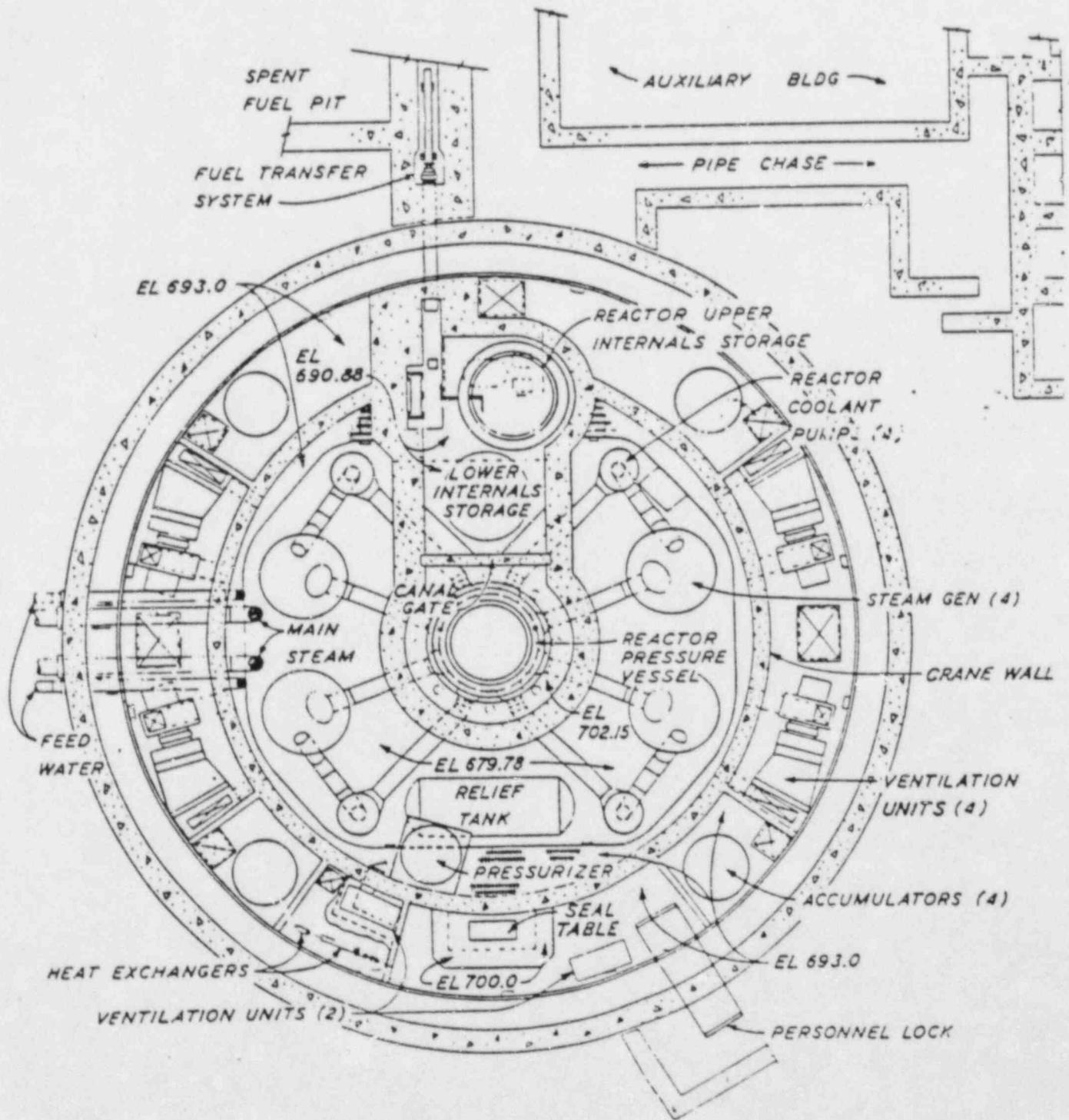
Figure 3.8.3-7 Plan-Lower Compartment
