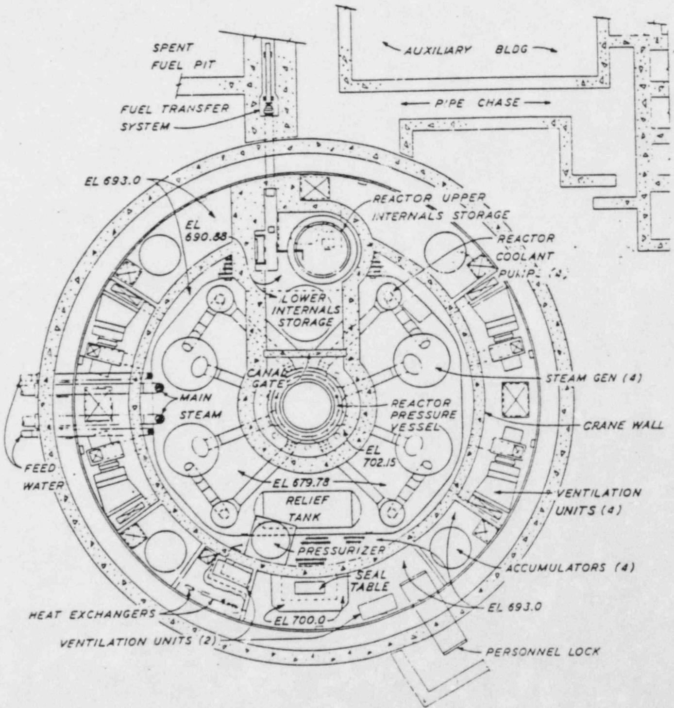
Figure 3.8.3-7 Plan-Lower Compartment
