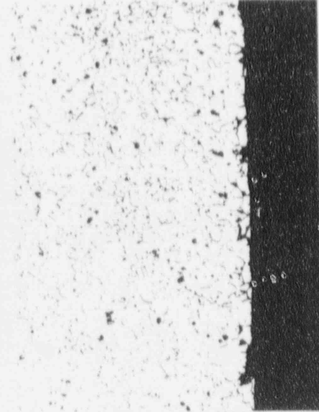
Figure 5-14. Transverse View of 'C'R29C70 TSP #3 Cracking.
