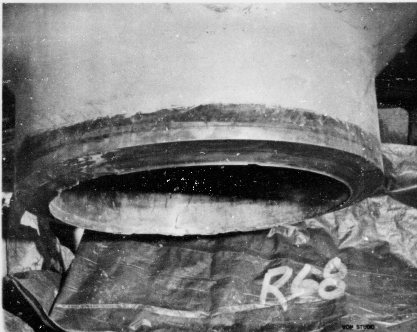
FIGURE 14. CLOSE-UP VIEW OF OUTLET NOZZLE ILLUSTRATING VISIBLE PHYSICAL DAMAGE TO LIP OF WELD PREPARATION - VIEW 1.
