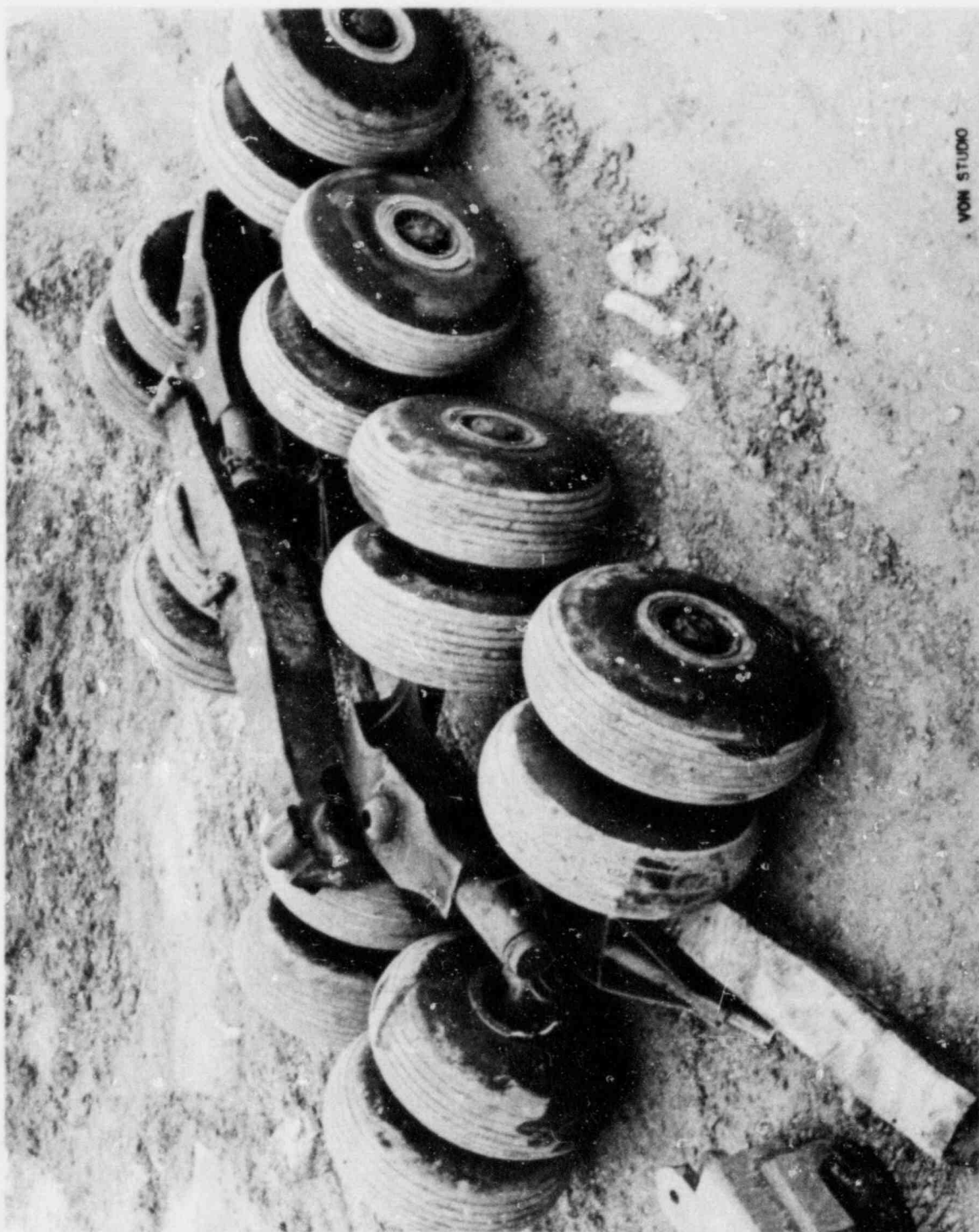
FIGURE 19. VIEW SHOWING THE WOODEN BLOCK USED TO BLOCK THE REAR TANDEM OF THE RIGHT TANDEM DOLLY.
