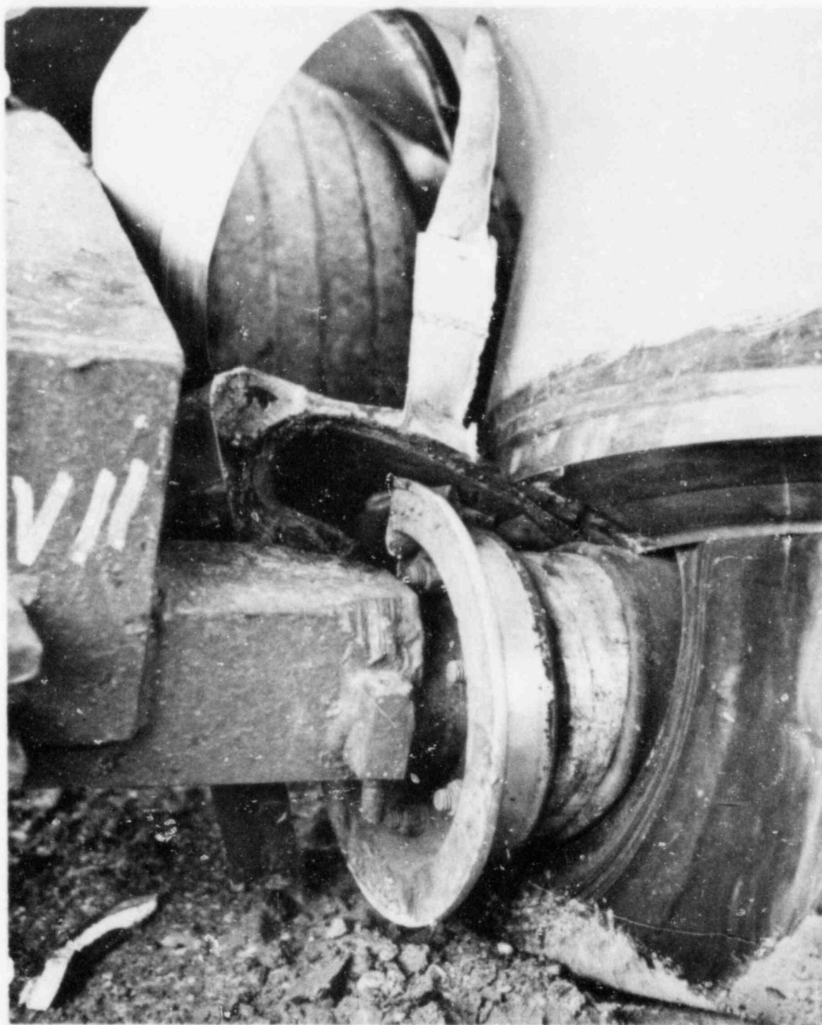
FIGURE 8. OUTLET NOZZLE RESTING ON DOLLY WHEEL RIM WITH TIRES AND AXLE EXTENDING INTO NOZZLE BORE - VIEW 1.
