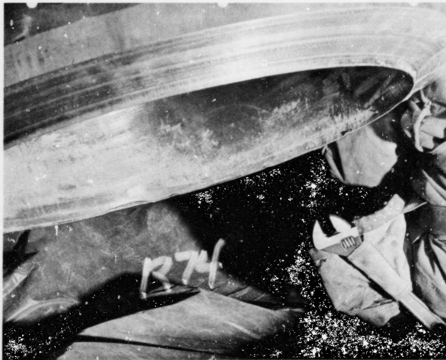
FIGURE 13. CLOSE-UP VIEW OF INLET NOZZLE ILLUSTRATING VISIBLE PHYSICAL DAMAGE TO LIP OF WELD PREPARATION - VIEW 2.
