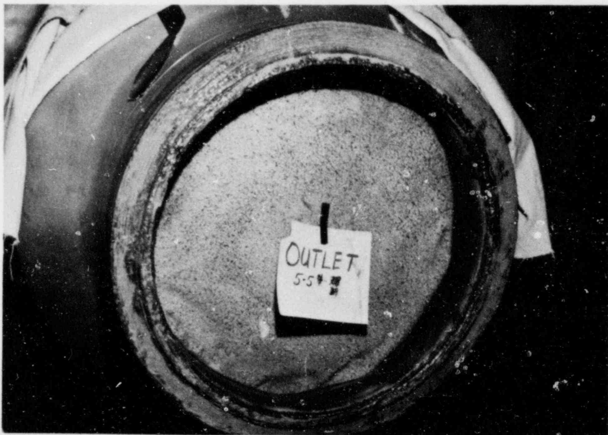
FIGURE 23. OUTLET NOZZLE AFTER COMPLETION OF WELDING THE ENTIRE WELD EDGE PREPARATION.
