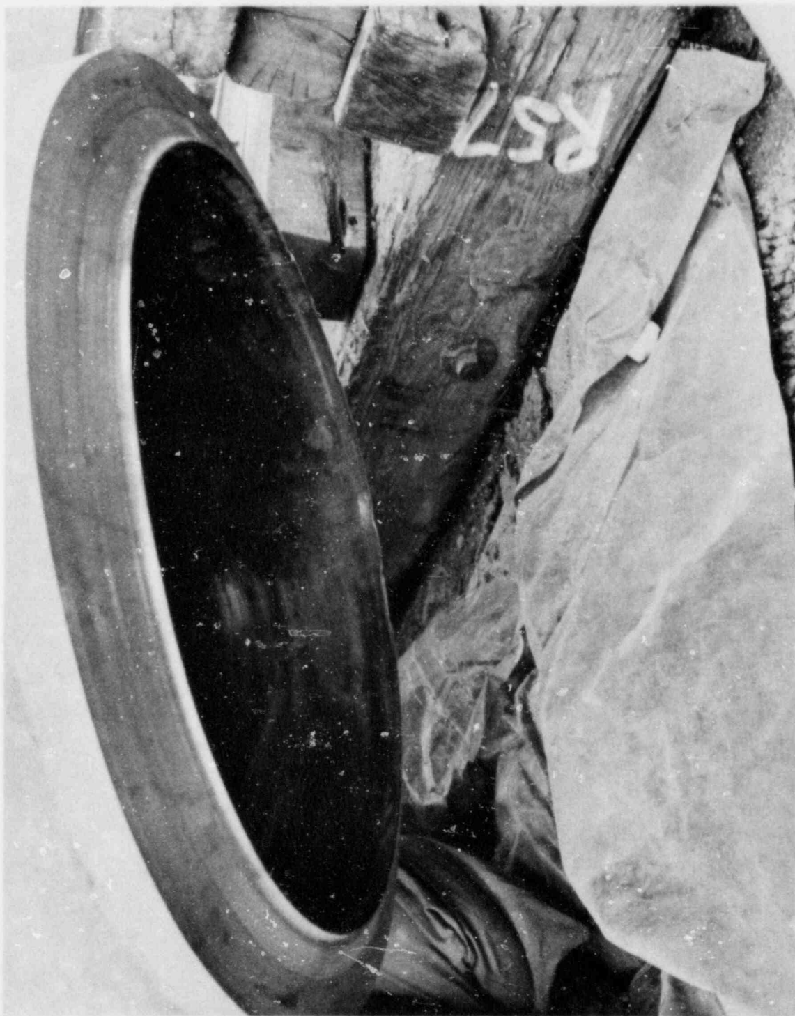
FIGURE 12. CLOSE-UP VIEW OF INLET NOZZLE ILLUSTRATING VISIBLE PHYSICAL DAMAGE TO LIP OF WELD PREPARATION - VIEW 1.
