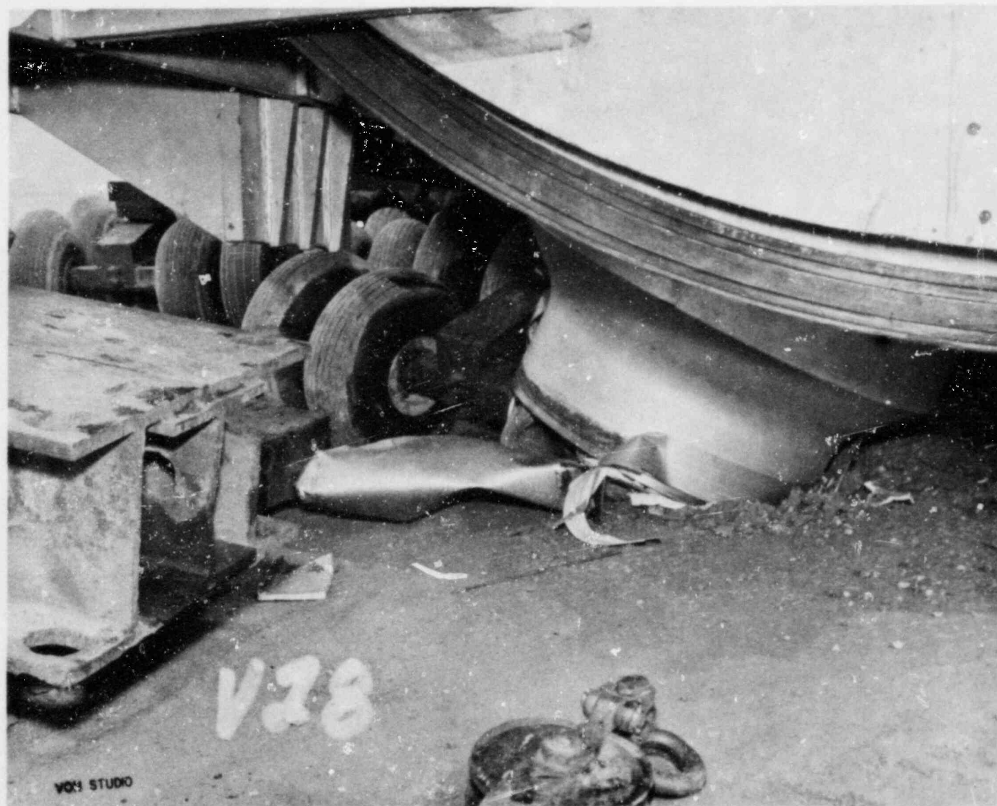
FIGURE 9. OUTLET NOZZLE RESTING ON DOLLY WHEEL RIM WITH TIRES AND AXLE EXTENDING INTO NOZZLE BORE - VIEW 2. Note penetration of nozzle into ground.
