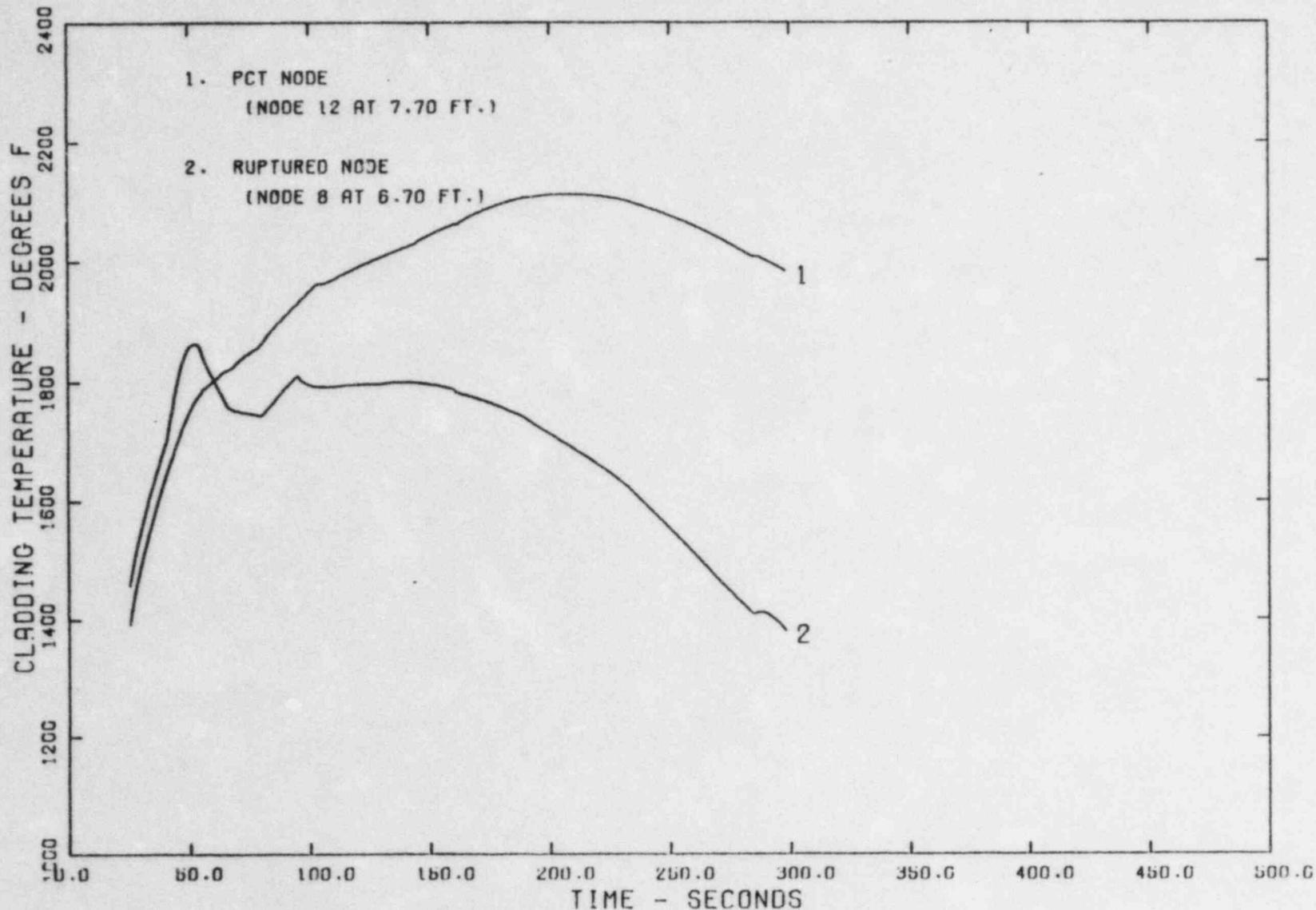
Figure 3.42 Cladding Temperature at PCT and Rupture Locations,
