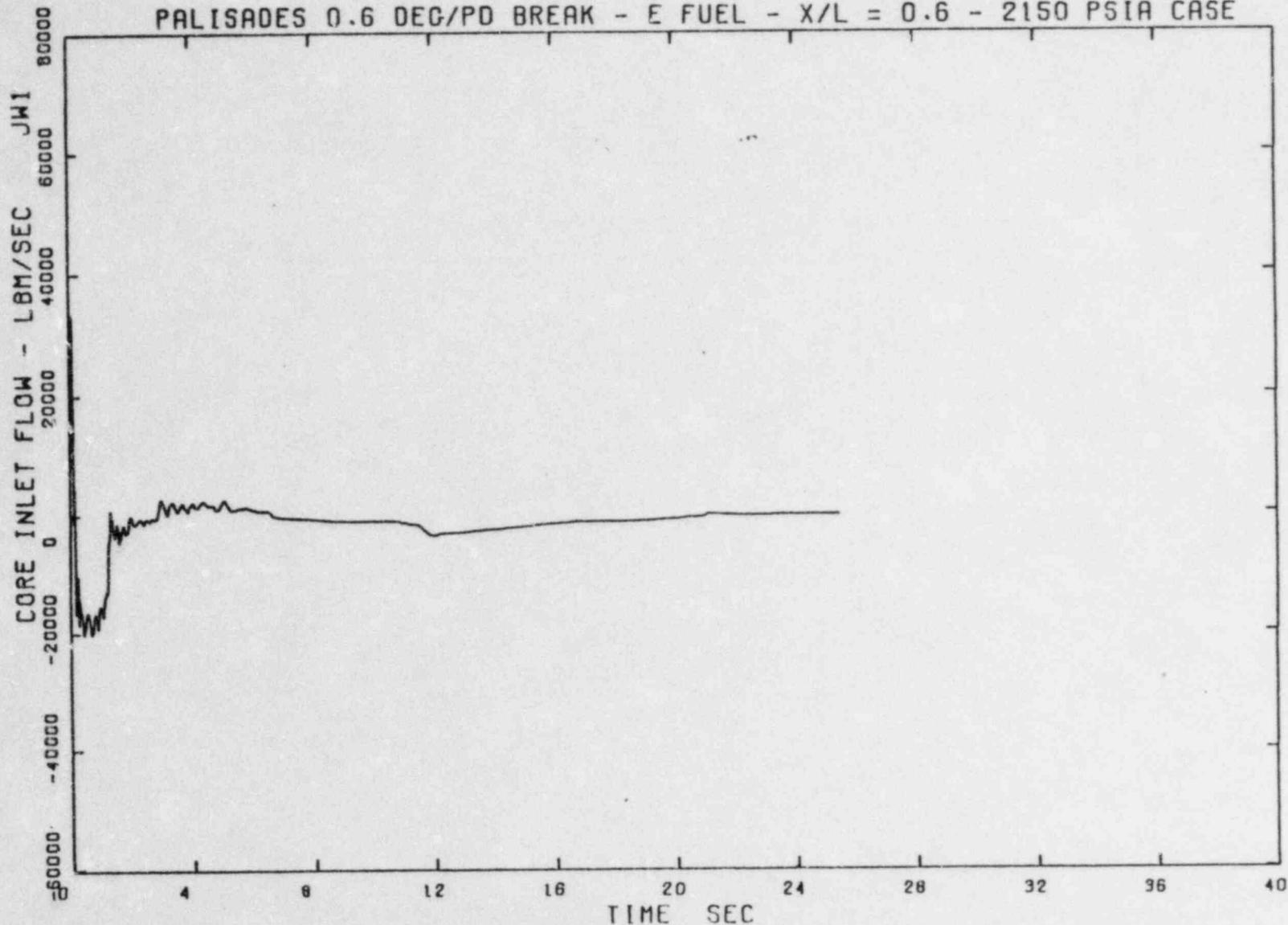
Figure 3.29 Average Core Inlet Flow During Blowdown,
