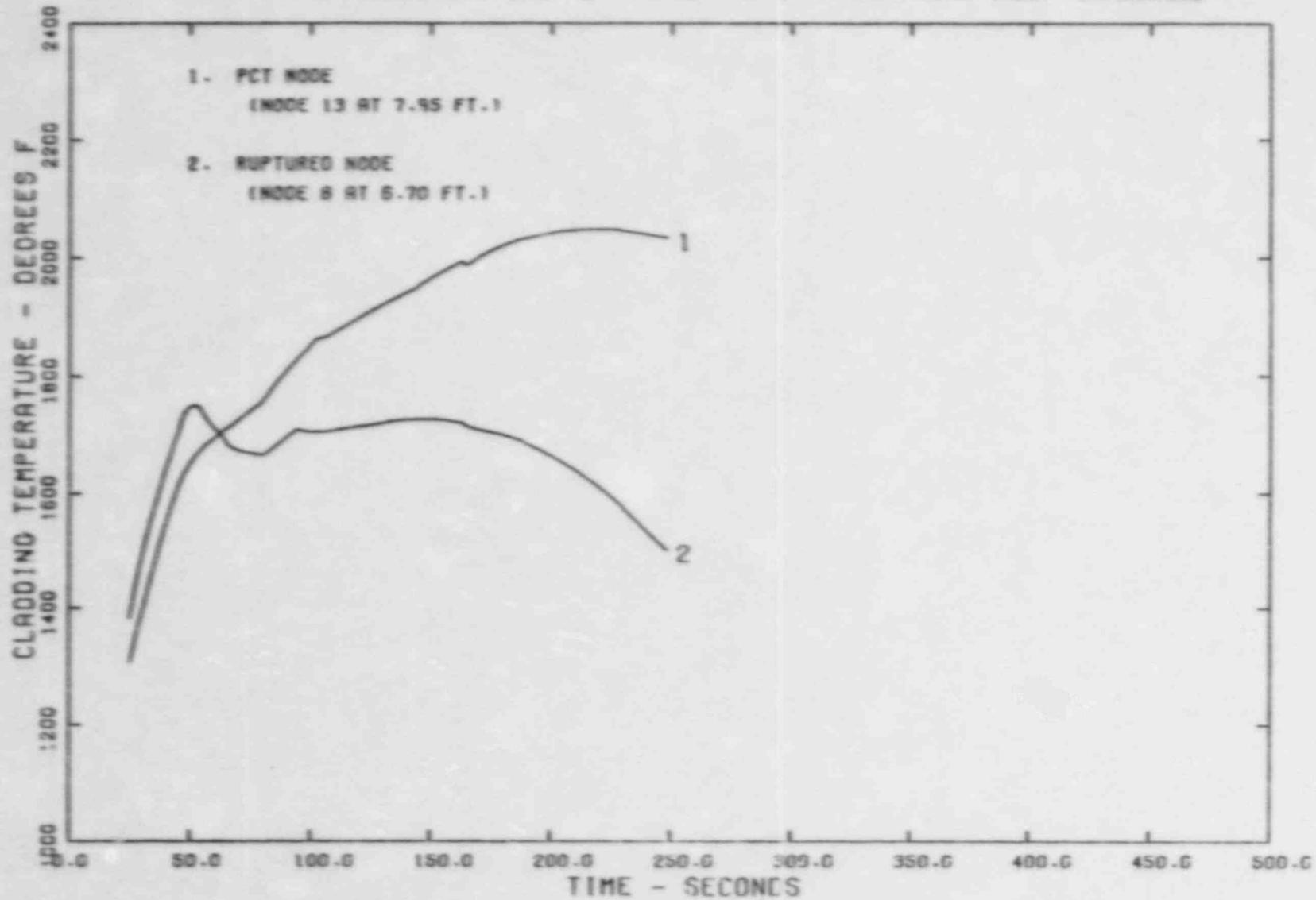
Figure 3.23 Cladding Temperatures at PCT and Rupture Locations, 545°F Core Inlet Temperature Case
