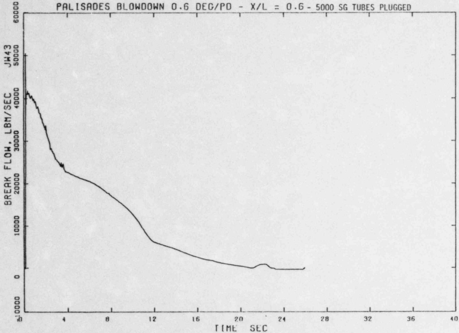
Figure 3.44 Pump Side Break Flow During Blowdown,
