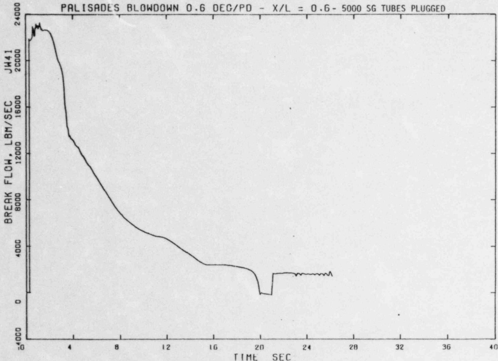
Figure 3.46 Vessel Side Break Flow During Blowdown, 5000 Tubes Plugged Case
