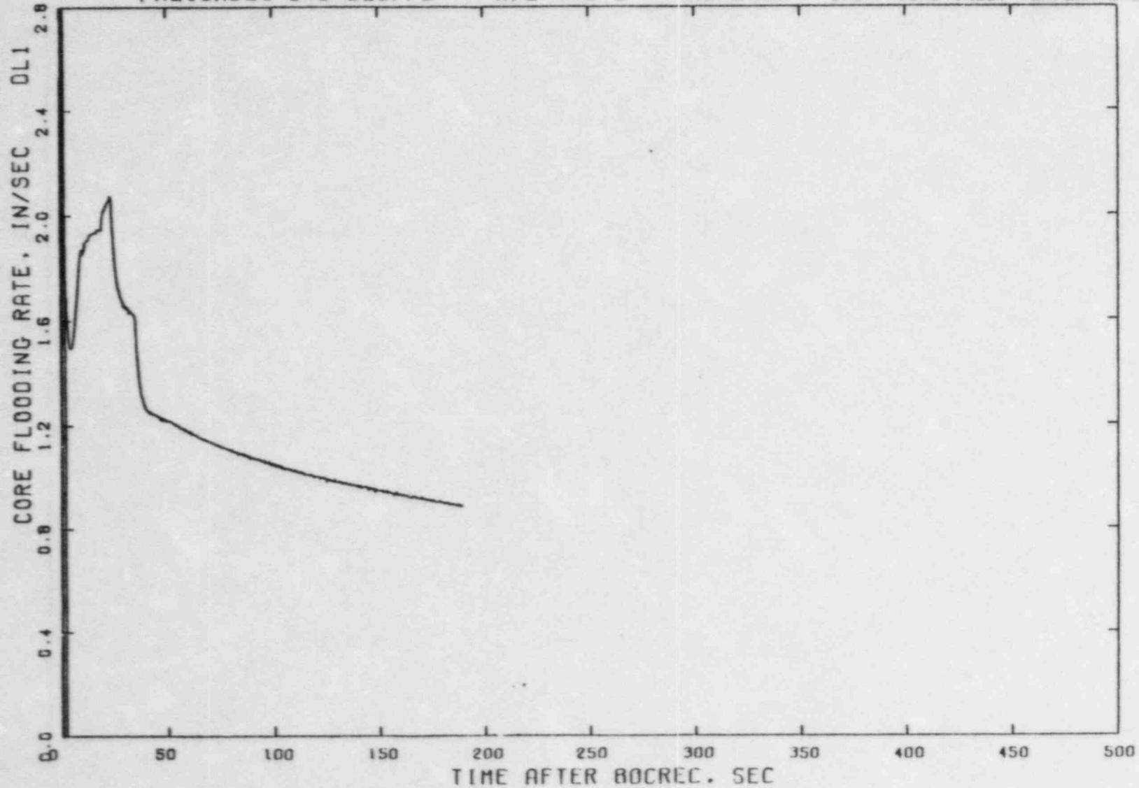
Figure 3.20 Core Reflood Rate During Reflood, 545°F Core Inlet Temperature Case
