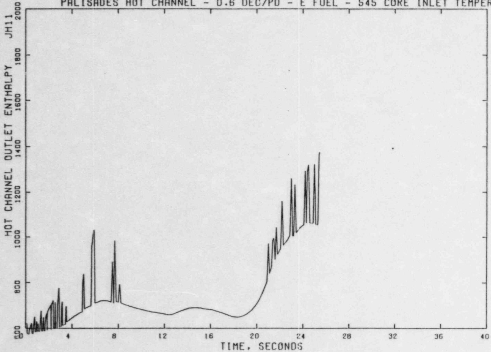
Figure 3.17 Hot Assembly Outlet Enthalpy During Blowdown,
