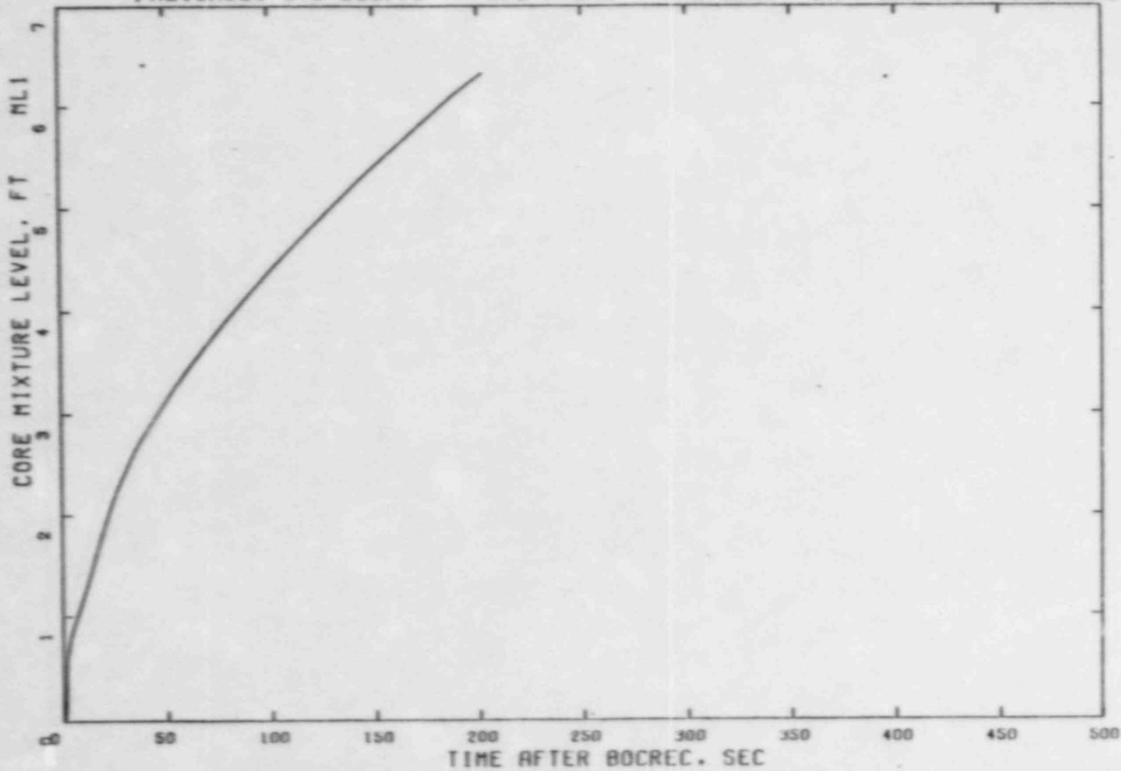
Figure 3.22 Collapsed Liquid Level in Core During Reflood, 545°F Core Inlet Temperature Case
