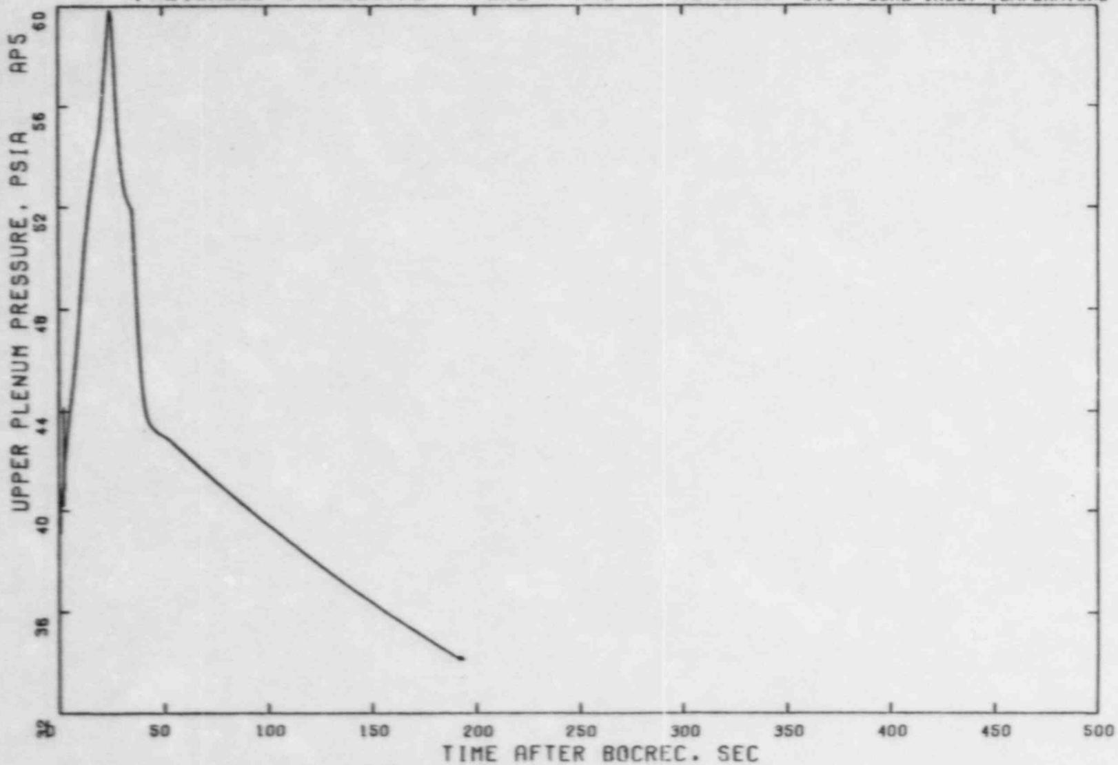
Figure 3.21 Upper Plenum Pressure During Reflood, 545°F Core Inlet Temperature Case
