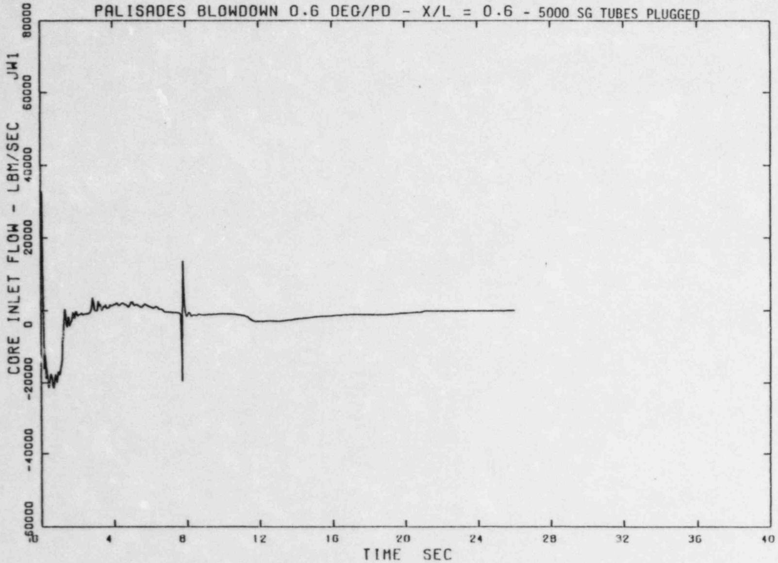
Figure 3.48 Average Core Inlet Flow During Blowdown,
