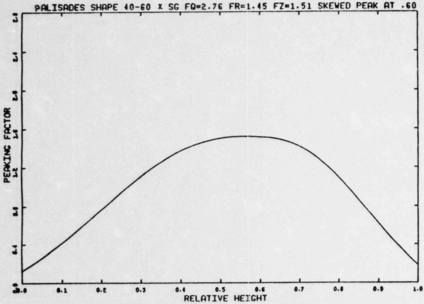
Figure 3.2 Axial Power Profile With Peak at X/L=0.6 and with Skewing Factor of 1.0
