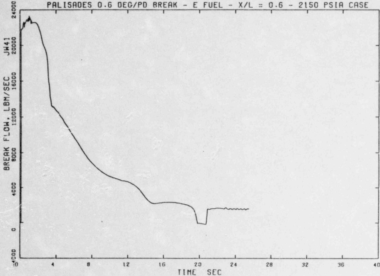
Figure 3.25 Pump Side Break Flow During Blowdown, 2150 psia Pressurizer Pressure Case
