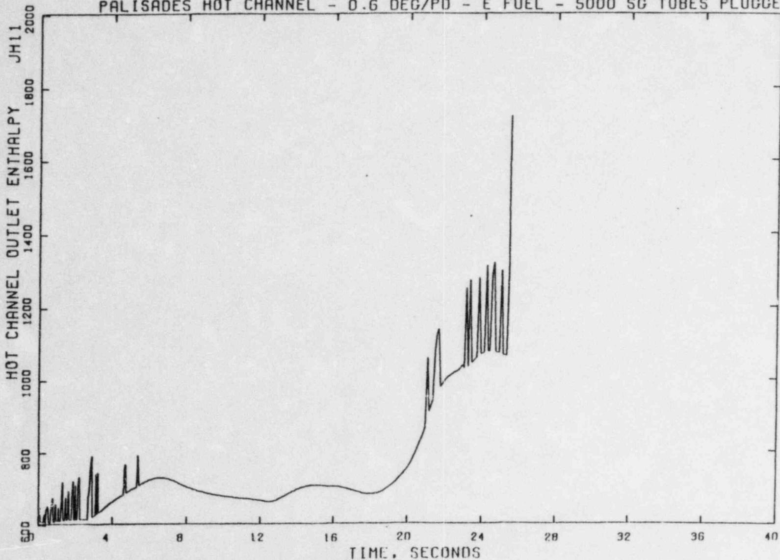
Figure 3.55 Hot Assembly Outlet Enthalpy During Blowdown,
