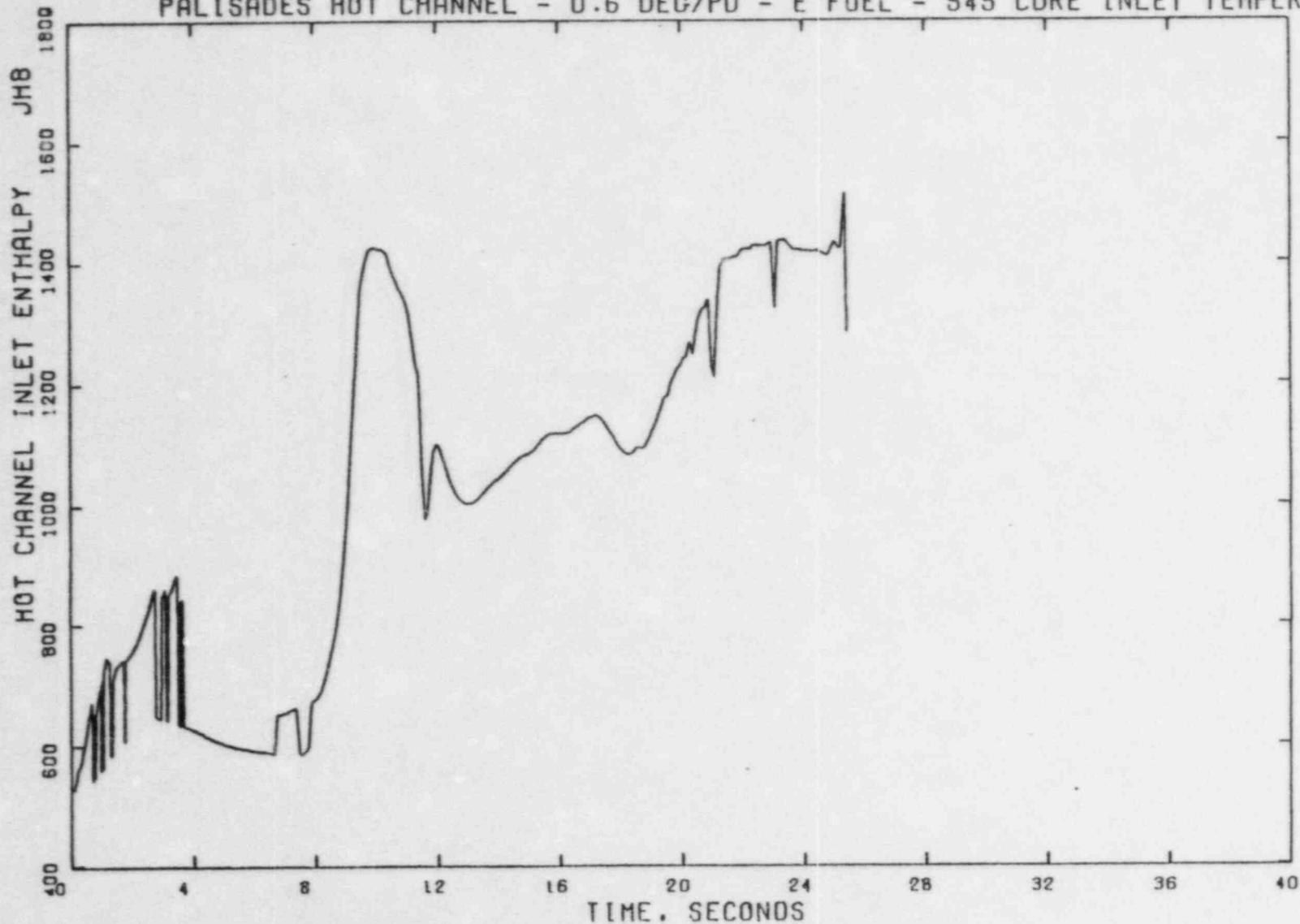
Figure 3.15 Hot Assembly Inlet Enthalpy During Blowdown,
