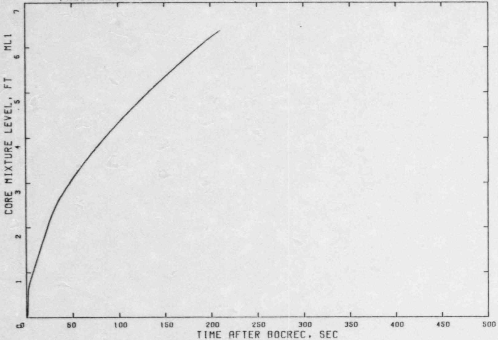
Figure 3.60 Collapsed Liquid Level in Core During Reflood, 5000 Tubes Plugged Case
