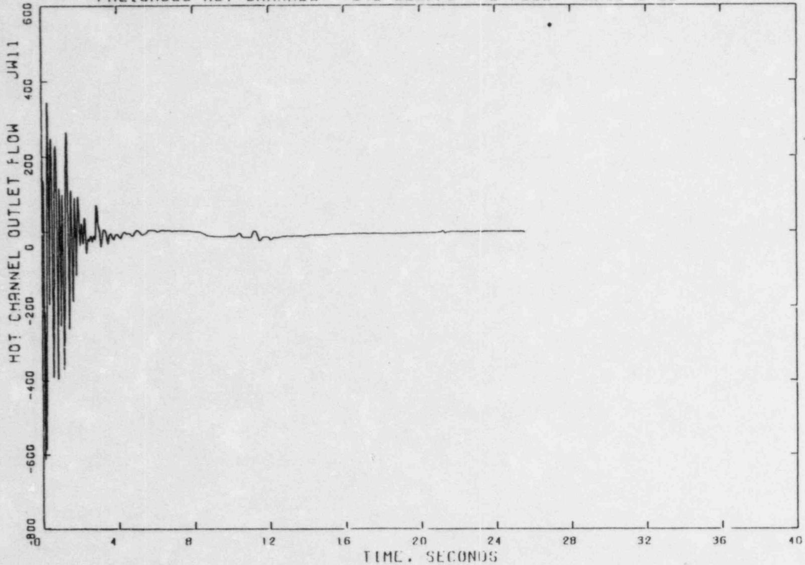
Figure 3.5 Hot Assembly Outlet Flow During Blowdown,
