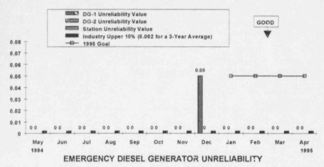
The purpose of this indicator is to monitor the likelihood that emergency AC power generators will respond to off-normal events or accidents. It also provides an indication of the effectiveness of maintenance, operation and test practices in controlling generator unreliability.
