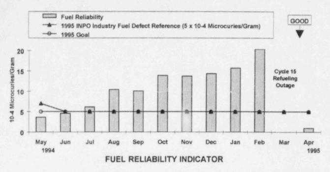
The FUEL RELIABILITY INDICATOR (FRI) for **April 1995** was **0.9556 X 10-4** microcuries/gram. The purpose of the FRI is to monitor industry progress in achieving and maintaining a high level of fuel integrity. The April FRI value, is less than the zero defect threshold value, however this does not necessarily confirm a defect free core, as discussed below.
