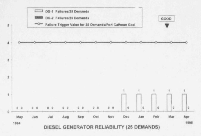
This indicator shows the number of failures experienced by each emergency diesel generator during the last 25 start demands and the last 25 load-run demands. A trigger value of 4 failures within the last 25 demands is also shown. This trigger value of 4 failures within 25 demands is the Fort Calhoun goal for 1995.
