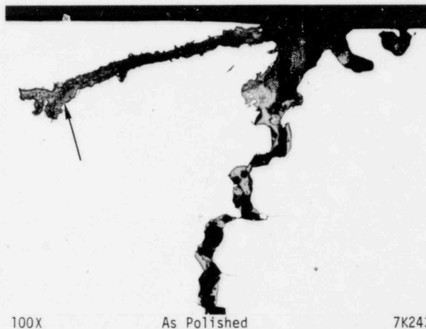
FIGURE 13. CROSS SECTION OF FLAW NO. 1 IN SECTION 1-S-S The arrow identifies the corrosion products in Flaw No. 1 (Area 3 in Table 4) that were subjected to EDAX analyses.
