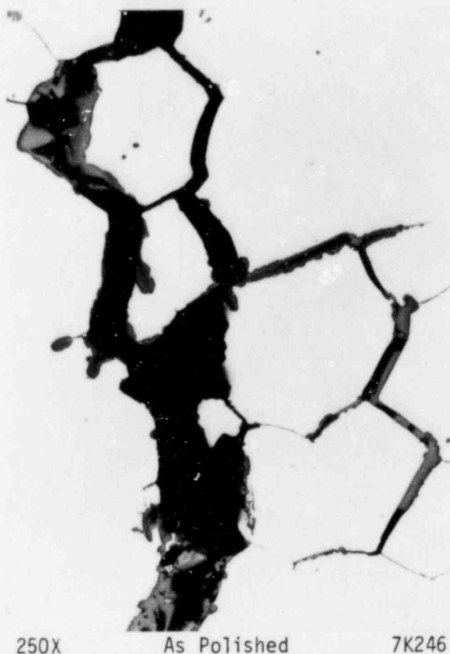
FIGURE 7. TYPICAL REGION OF THE INTERGRANULAR CRACK THAT WAS LOCATED WITHIN CIRCLED AREA 3 IN FIGURE 5a
