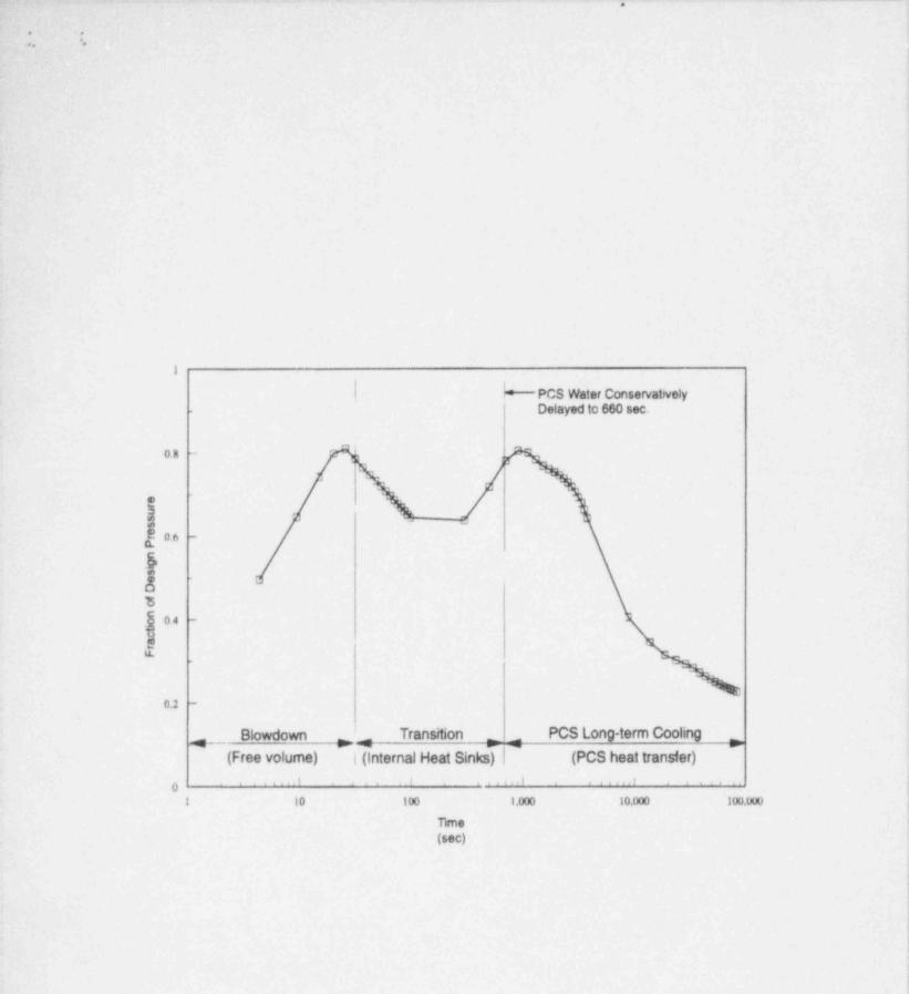
Figure 2-1 AP600 PCS LOCA Design Basis Analysis Pressure Transient (from Reference 3)
