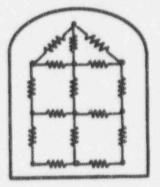
WGOTHIC Distributed Parameter \* (Finite Difference, Large Mesh)
