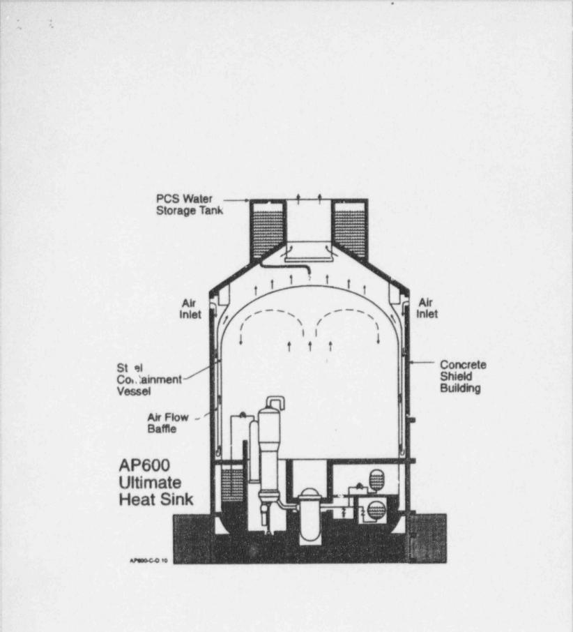
Figure 3-1 AP600 Passive Containment Cooling System Arrangement
