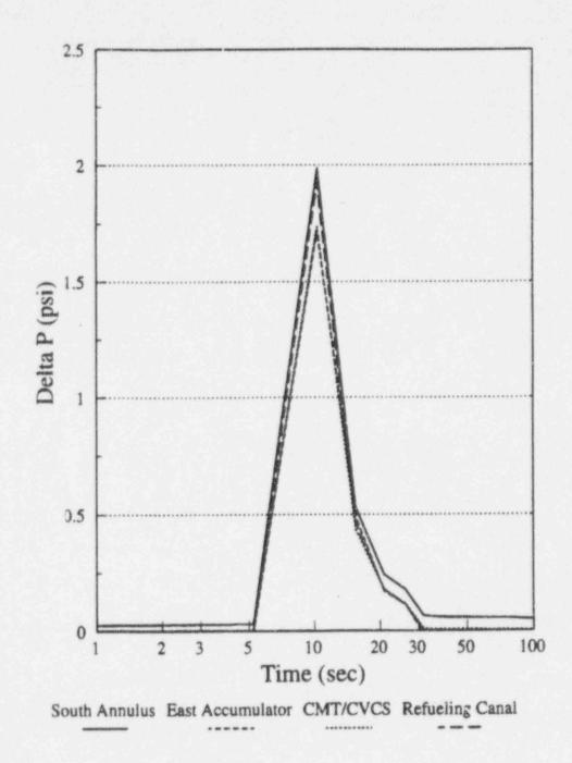
Figure 3-2 AP600 LOCA Break (Steam Generator) Compartment Relative Pressurization
