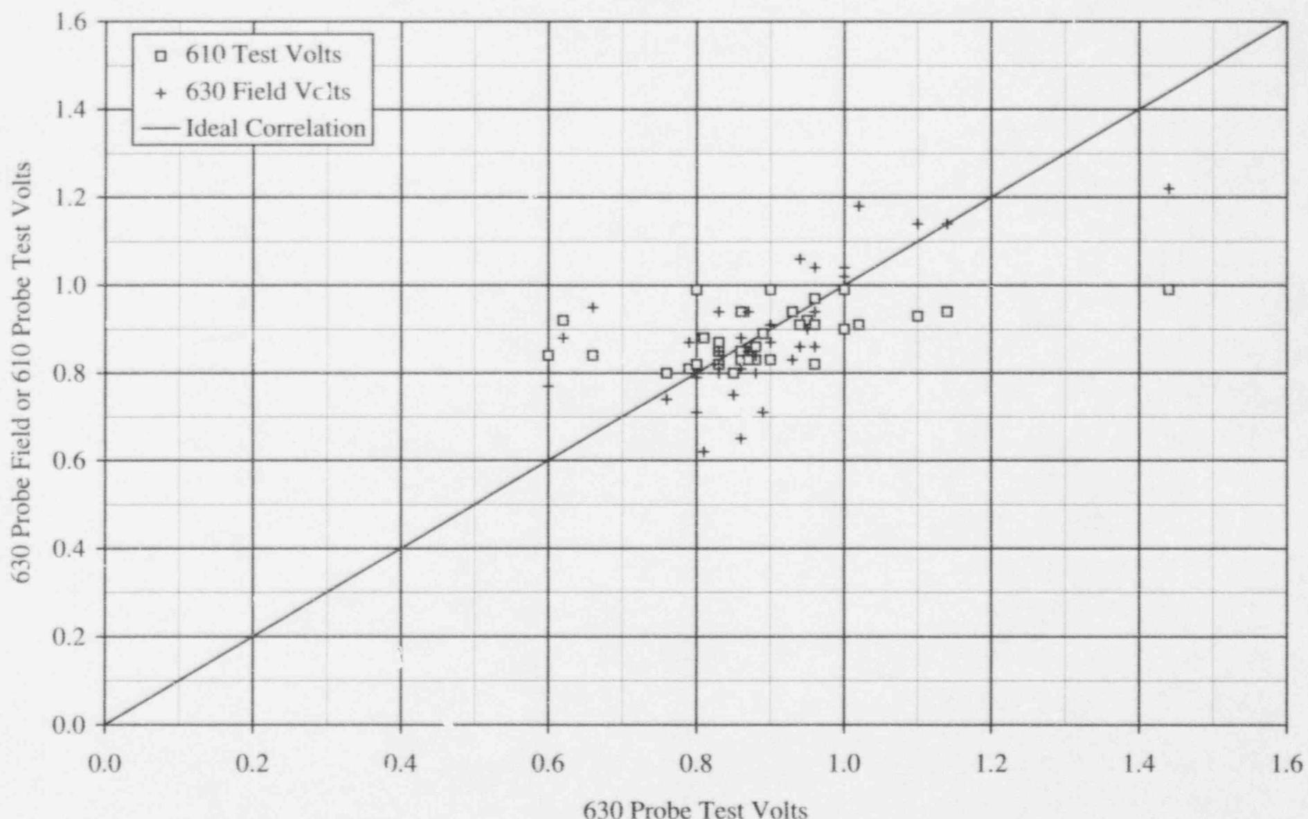
**Comparison of Bin 2 630 to 610 Probe Volts**
