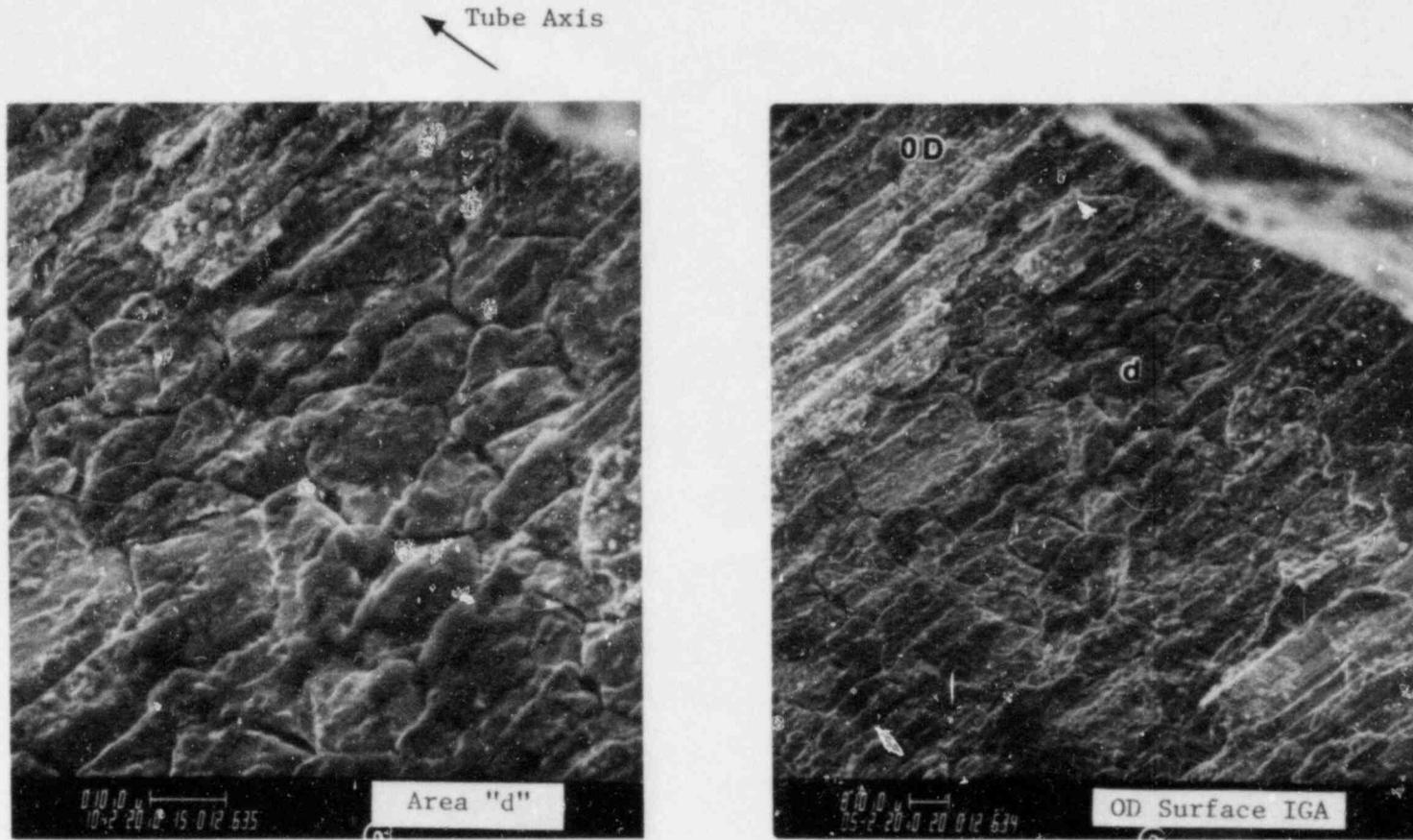
Figure 2-31. SEM Micrographs of Tube B73-8 Area 9 (After Cleaning)
