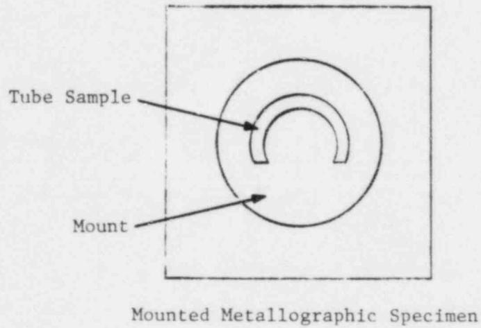
Figure 2-39. Longitudinal Metallographic Examination Technique
