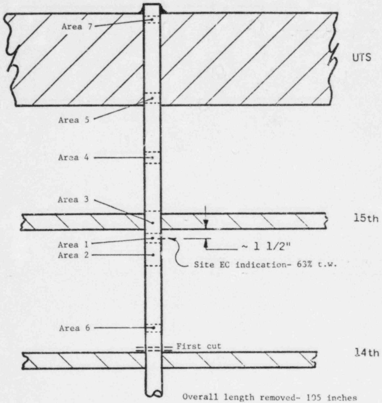
Figure 2-2. Tube B112-19 Schematic
