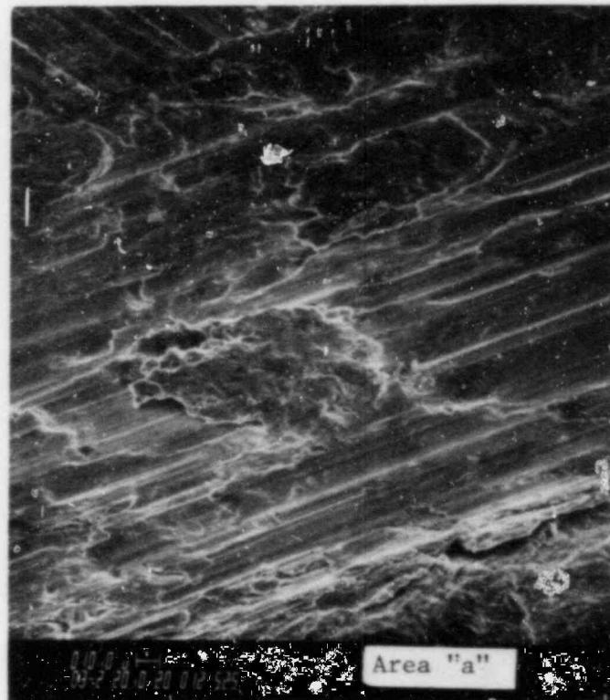
Figure 2-26. SEM Micrographs of Tube B112-19 Area 1 (After Cleaning)
