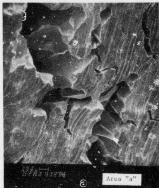
Figure 2-29. SEM Micrographs of Tube B112-19 Area 1 (After Bending)
