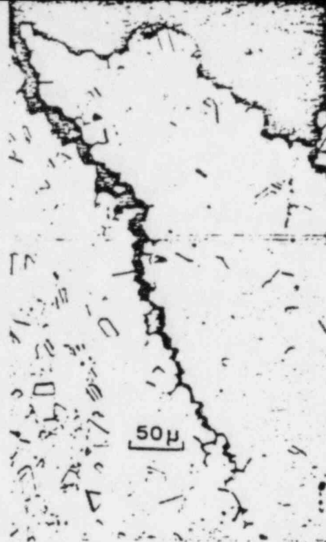
FIGURE 22 — Tensile specimen ( \alpha = 2/3 E_{0.2} 300 C) after 2,000 hours in 350 C deoxygenated water. Intergranular nature of the crack.
