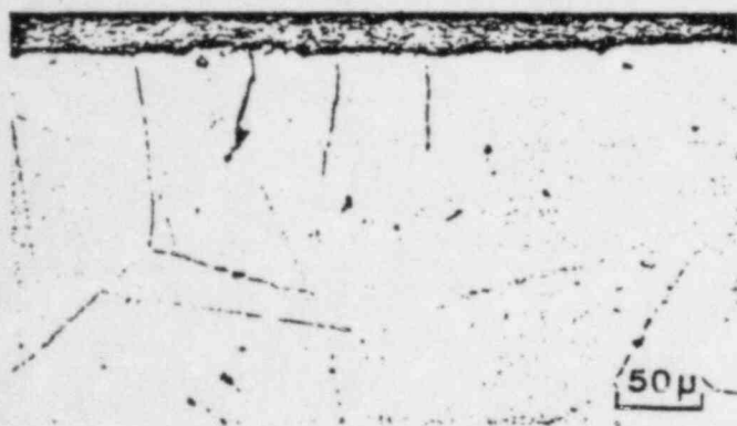
FIGURE 21 — Example of intragranular cracks.
