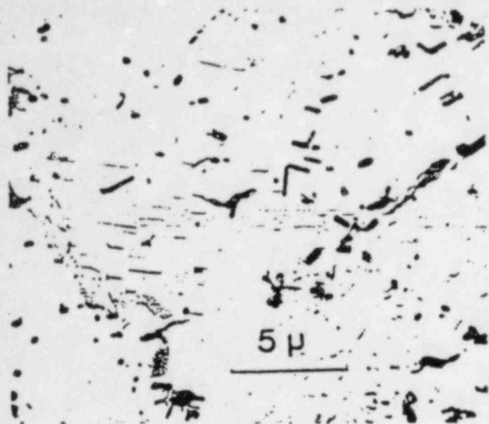
FIGURE 13 — Alloy A (Inconel 600) electron microscopic examinations. A3 = Sensitized condition (one hour at 700 C).
