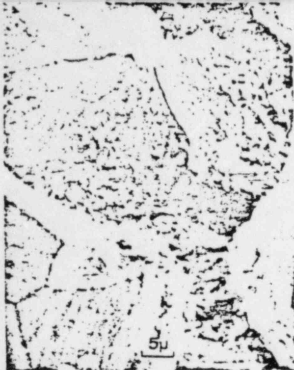
FIGURE 27 — Precipitates at grain surfaces on flanks of the crack (Inconel X 750).
