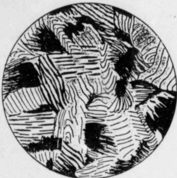
Fig. 3-5. Here is how the pearlite grains arrange themselves in a eutectoid mixture.
