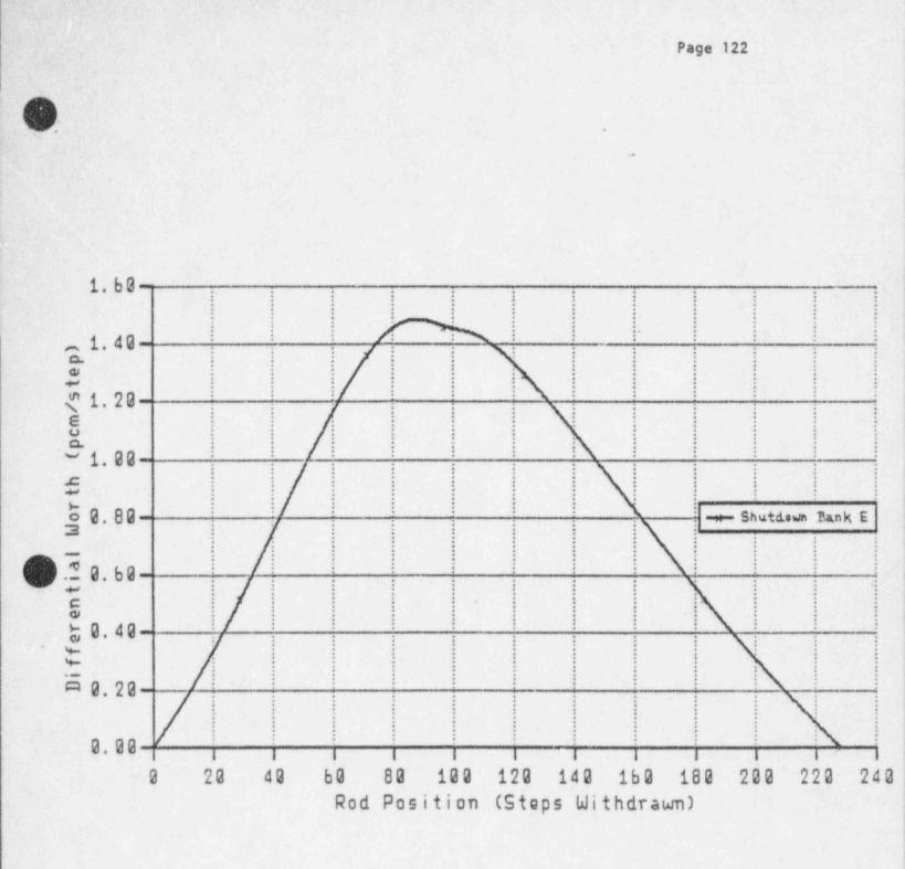
Millstone Nuclear Power Station Unit No. 3 DIFFERENTIAL CONTROL ROD WORTH SHUTDOWN BANK E 7.5-19
