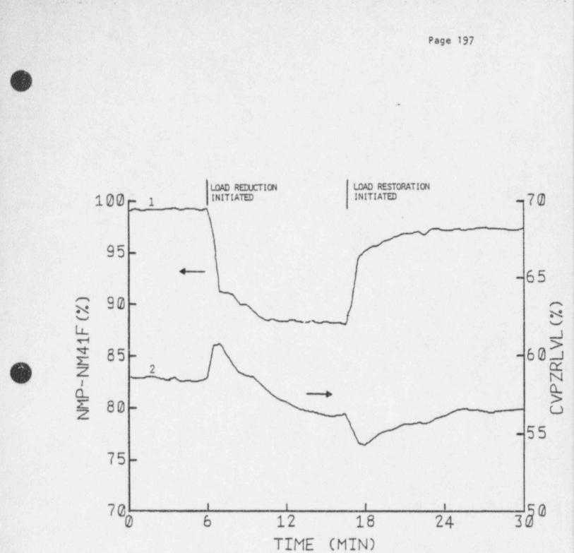
FLOT 1 - REACTOR POWER-POWER RANGE DETECTOR CHANNEL 41 FLOT 2 - PRESSURIZER LEVEL
