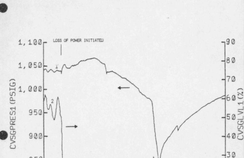
PLOT 1 - STEAM GENERATOR 1 PRESSURE PLOT 2 - STEAM GENERATOR 1 NARROW RANGE LEVEL
