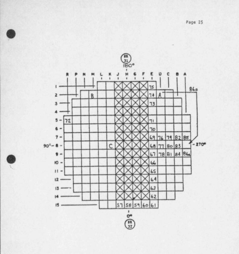
Millstone Nuclear Power Station Unit No. 3 INITIAL CORE LOADING SEQUENCE STEPS 57 TO 86B
