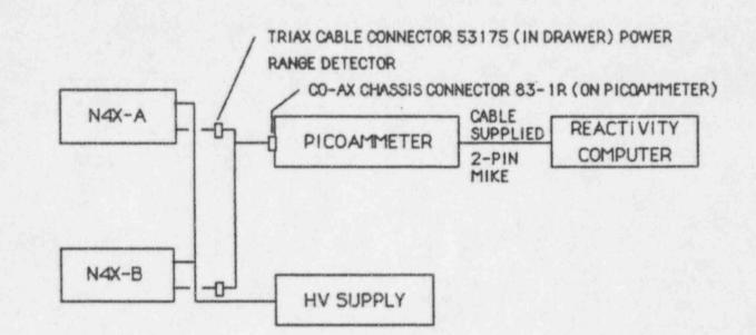
NOTES: The Nuclear Instrumentation Detector cables are Triax cables terminated with Amphenol 43175 connectors. The Keithley picoammeter and power supply inputs are 83-1R Co-ax connectors. Triax connector 53175 mates with Amphenol 52975 for cableto-cable connection or Amphenol 34475 for cable-to-chassis termination. Chassis Co-ax connector 83-1R mates with cable connector 83-1SP.
