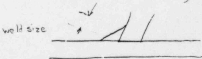
~~It is clear that~~ To "measure" by the Palo Verde method to a given size (e.g.  $\frac{5}{16}$  inch on a  $120^\circ$  weld) will result in an undersize weld by the Code definition (in this case by  $\frac{3}{64}$  inch)
