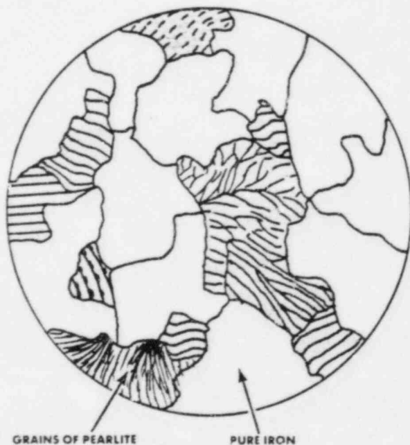
Fig. 3-6. An example of hypoeutectoid grain structure.
