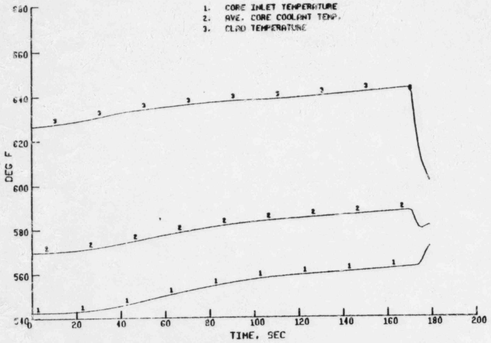
Figure 4.14 Core Inlet, Core Coolant, and Clad Temperature -
