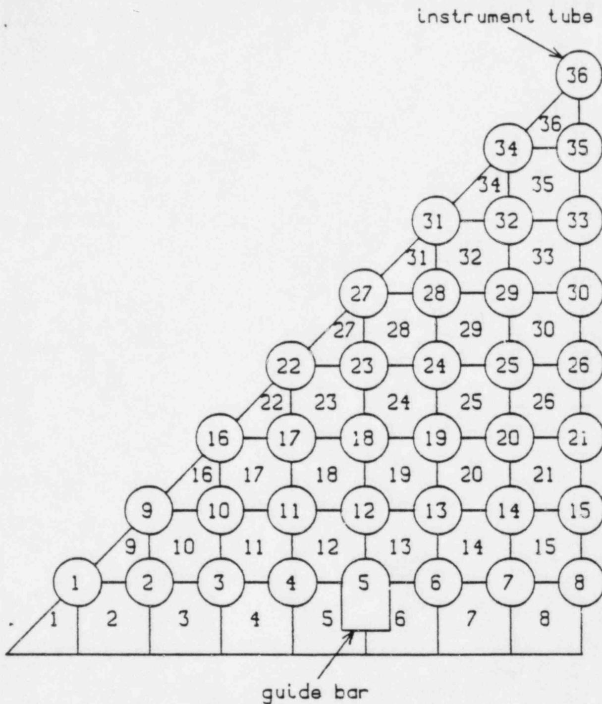
Figure 3.4 Rod and Channel Number Index.
