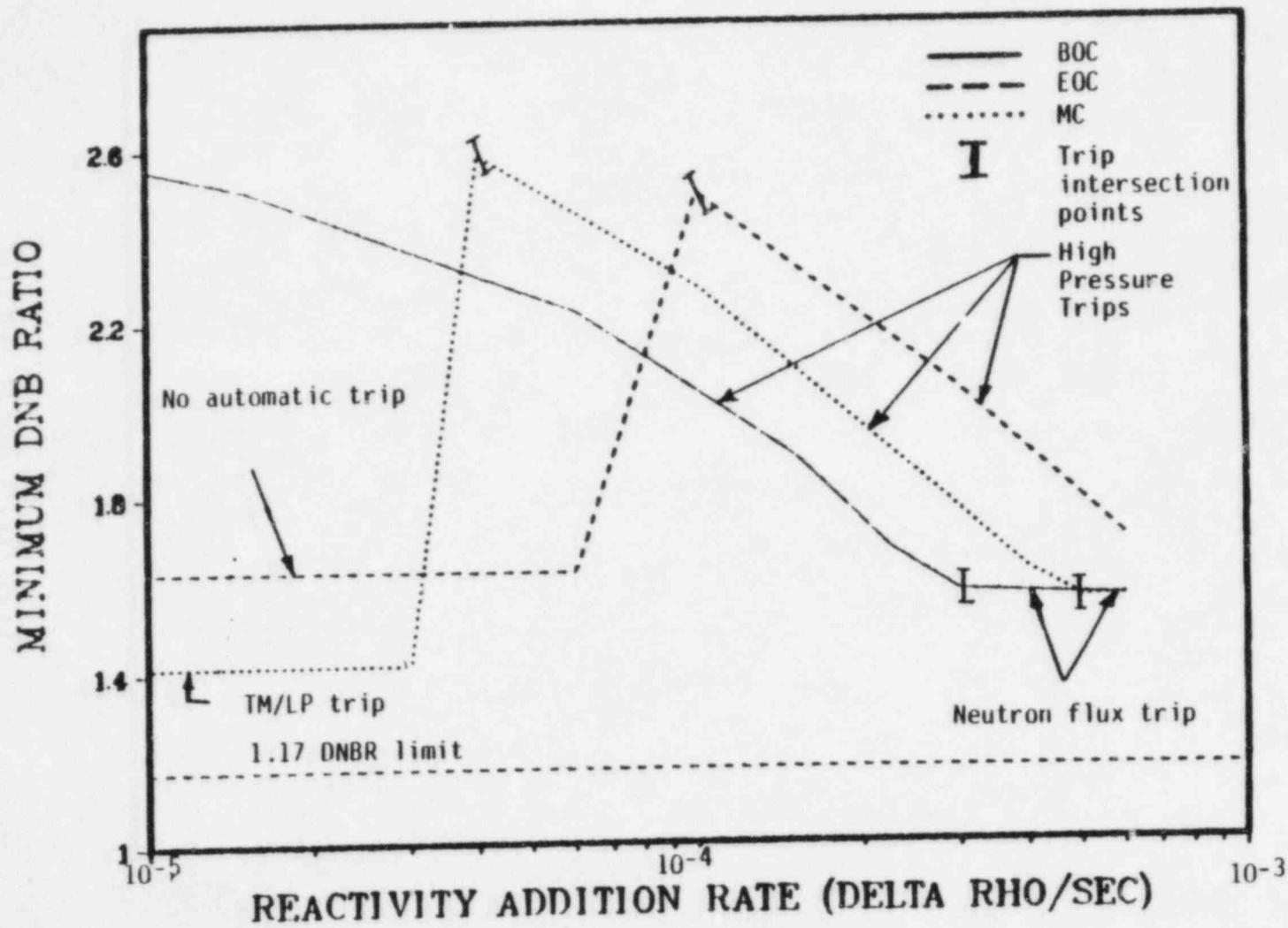
Figure 2.1 MDNBR Values for Rod Withdrawal Transients Initiated from 52% of Rated Power
