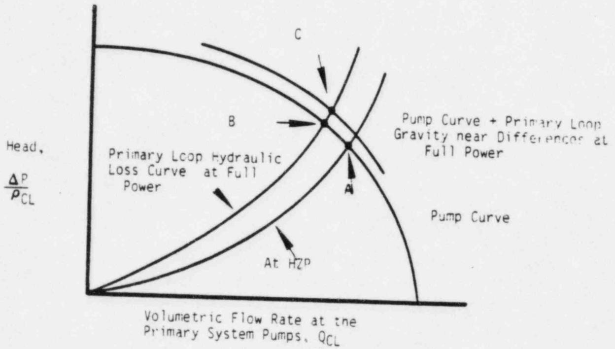
Figure A.1 Pump Curve, Gravity head, and Hydraulic Loss Curve Schematic Utilized in Development of Coolant Flow Upgrade
