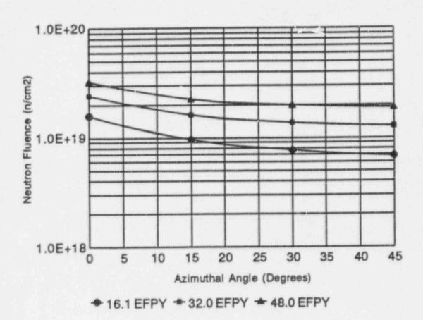
FAST NEUTRON FLUENCE (E > 0.1 MeV) AS A FUNCTION OF AZIMUTHAL ANGLE AT THE INNER RADIUS OF THE BELTLINE CIRCUMFERENTIAL WELD
