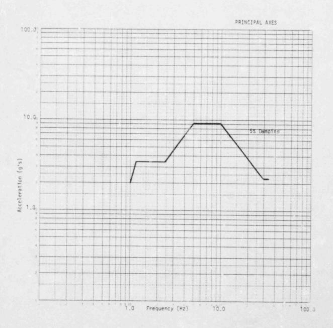
Figure 3: Required Response Spectrum (RRS) for Safe Shutdown Earthquake (SSE)
