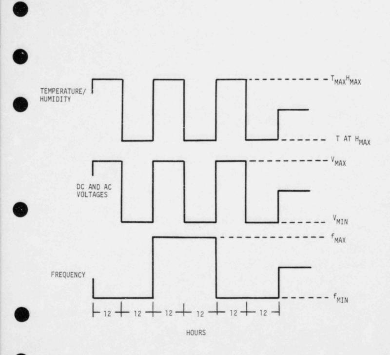
Figure 2 Verification Test Profile
