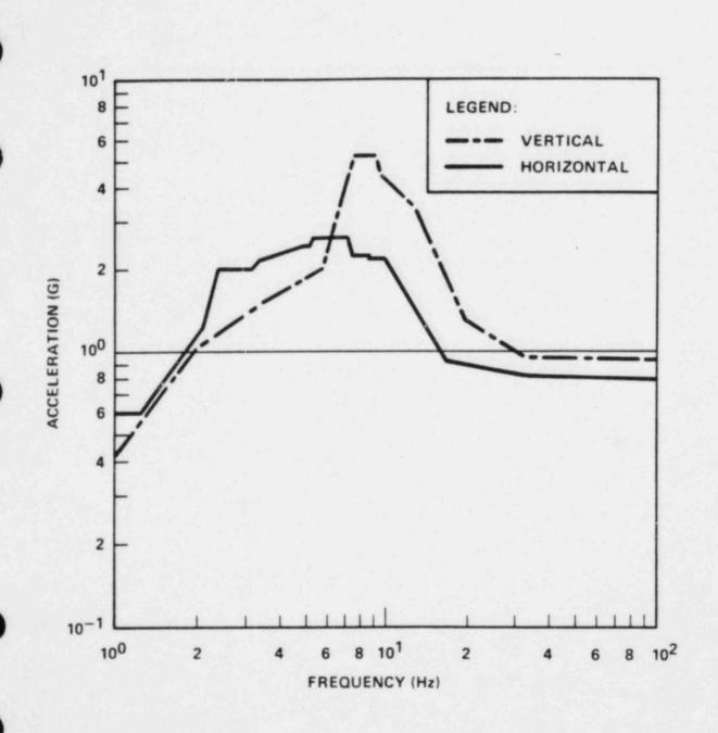
Figure 3 SSE Required Response Spectra for the Generic Auxiliary Safeguards Cabinet
