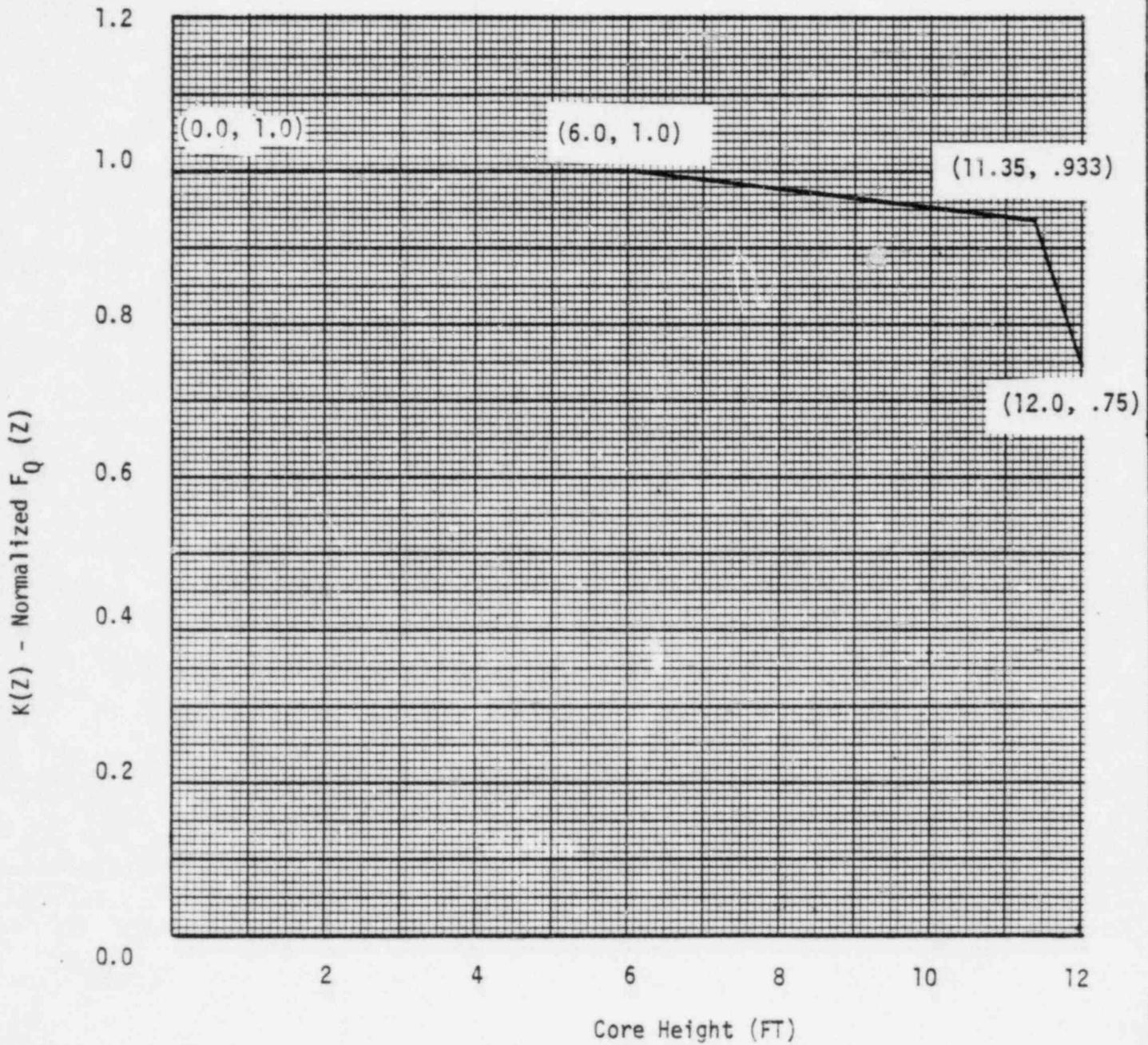
Figure 3.2-3  $K(Z)$  - Normalized  $F_Q(Z)$  As A Function of Core Height For Westinghouse Fuel
