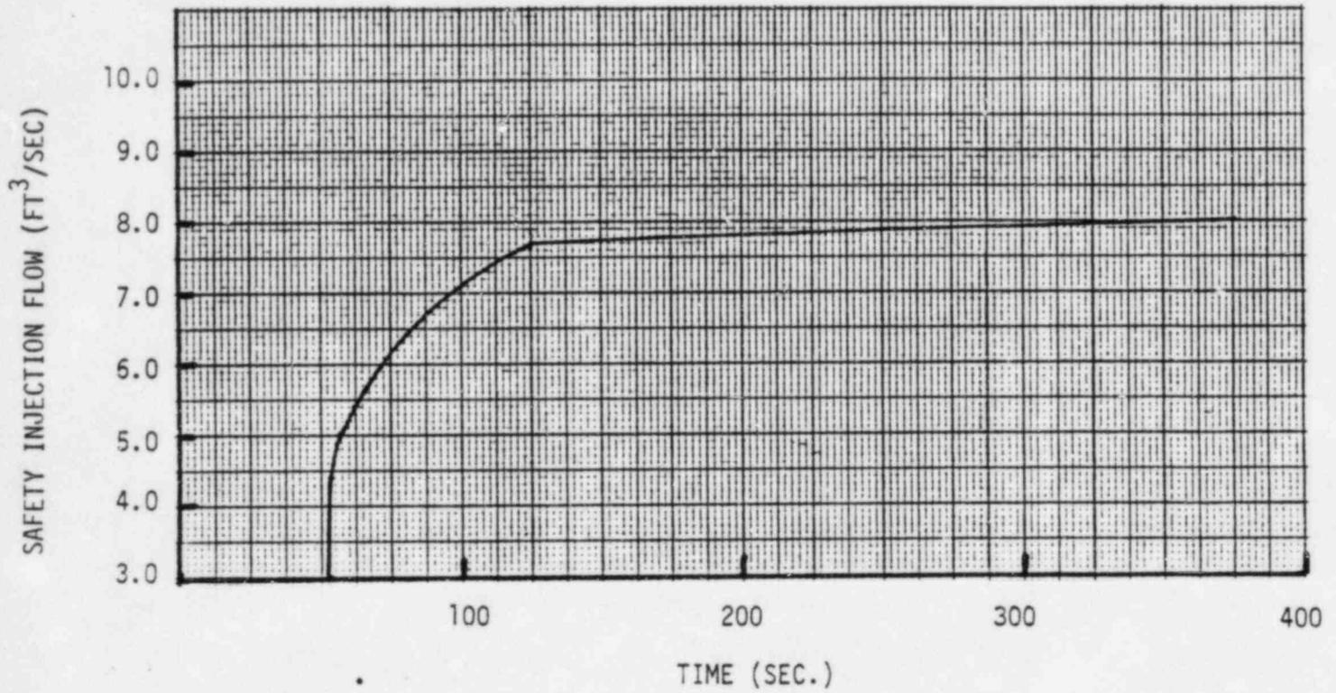
FIGURE 14.3.1-47 PUMPED ECCS FLOW (REFLOOD) DECLG(CD = 0.4)
