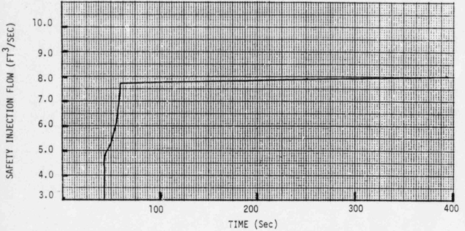
FIGURE 14.3.1-45 PUMPED ECCS FLOW (REFLOOD)
