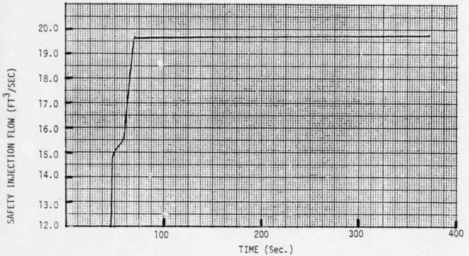
FIGURE 14.3.1-48 PUMPED ECCS FLOW (REFLOOD - DECLG (CD - 0.4)
