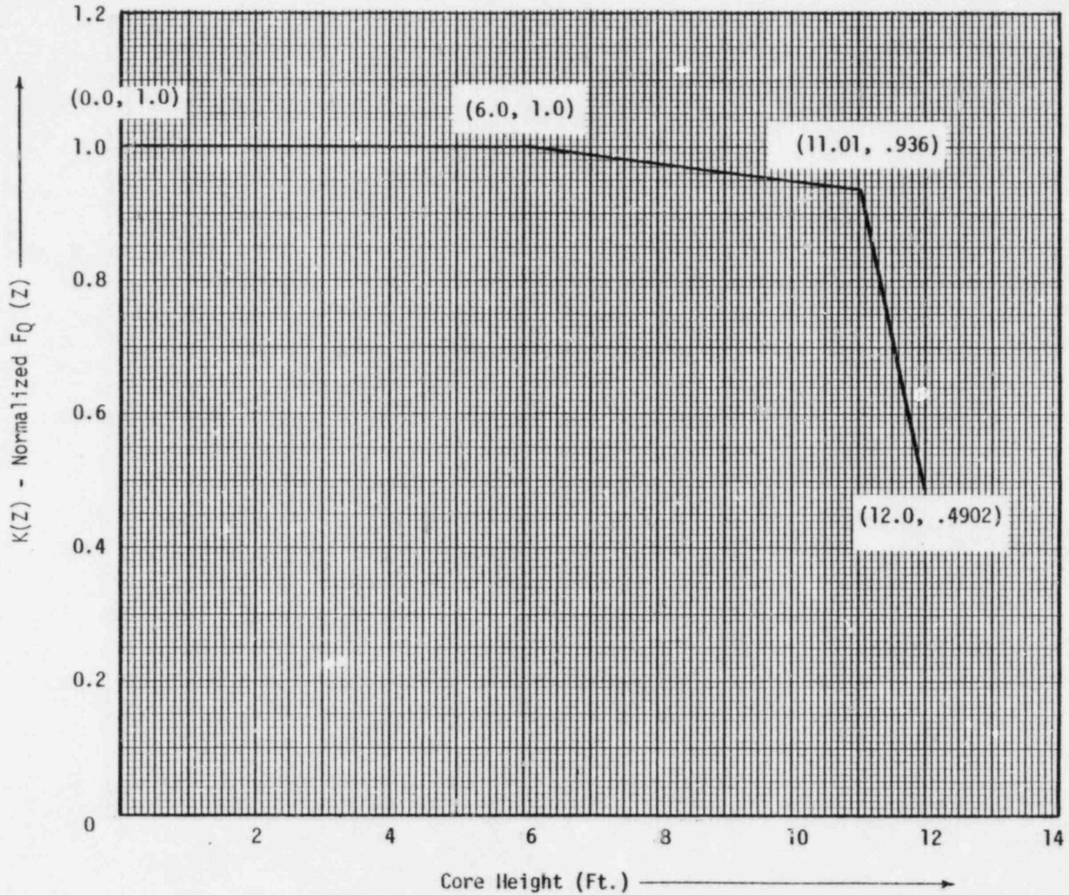
Figure 3.2-2  $K(Z)$  - Normalized  $F_0(Z)$  As A Function of Core Height for Exxon Nuclear Company Fuel
