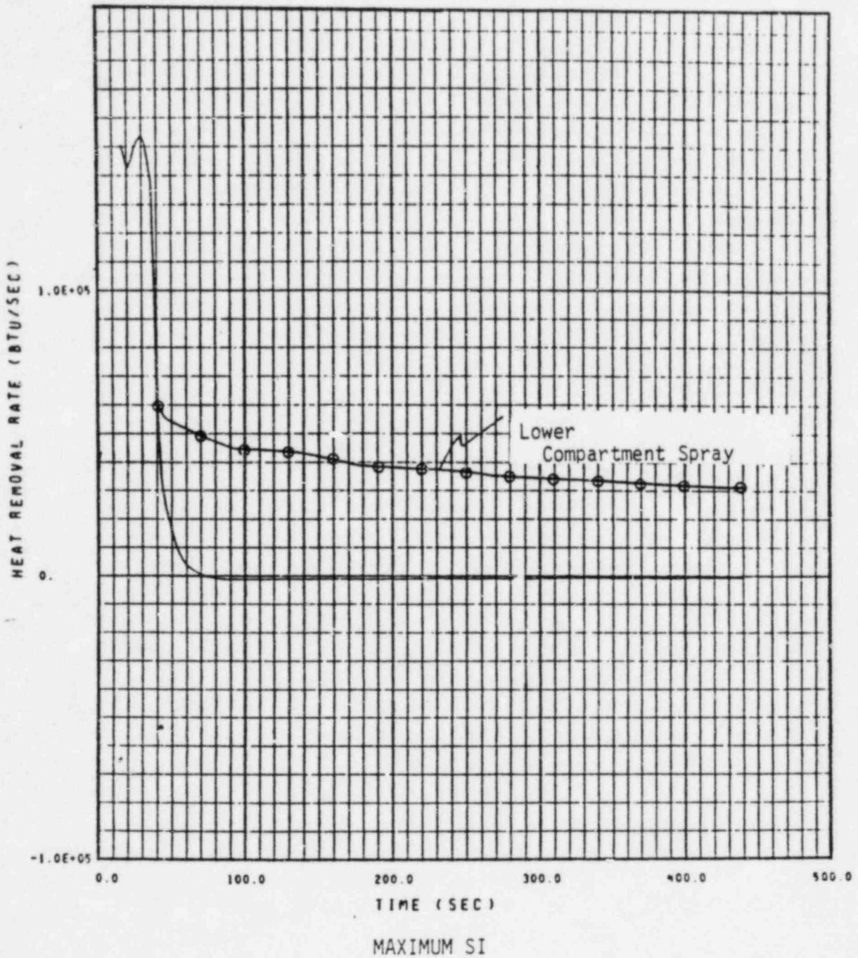
FIGURE 14.3.1-60 HEAT REMOVAL BY SUMP AND LC SPRAY
