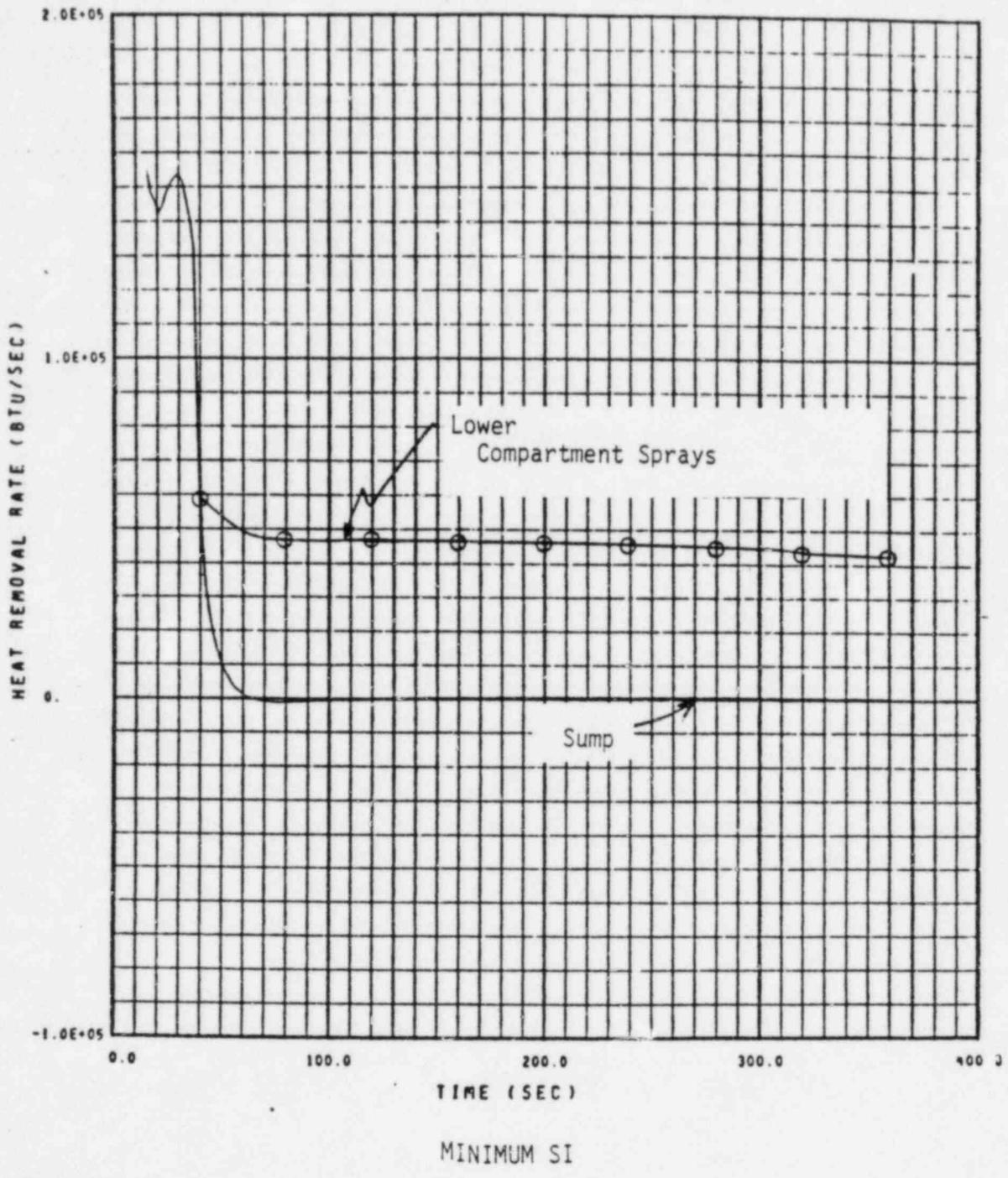
FIGURE 14.3.1-59 HEAT REMOVAL BY SUMP AND LC SPRAYS
