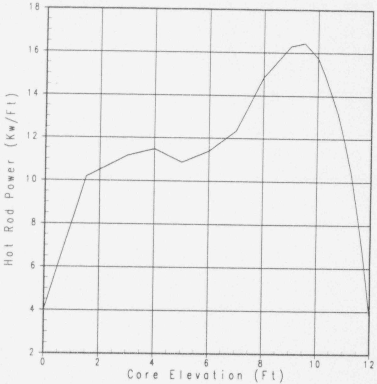
Figure 12 - 4 Loop Plant Power Shape (Kw/Ft)
