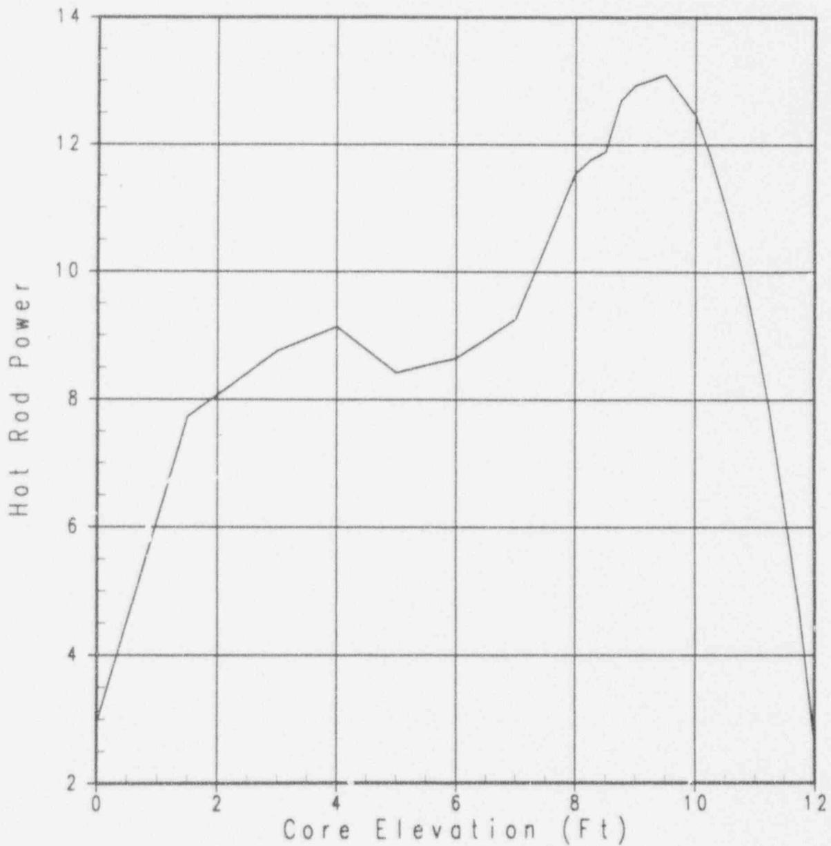
Figure 2 - 3 Loop Plant Power Shape (Kw/Ft)
