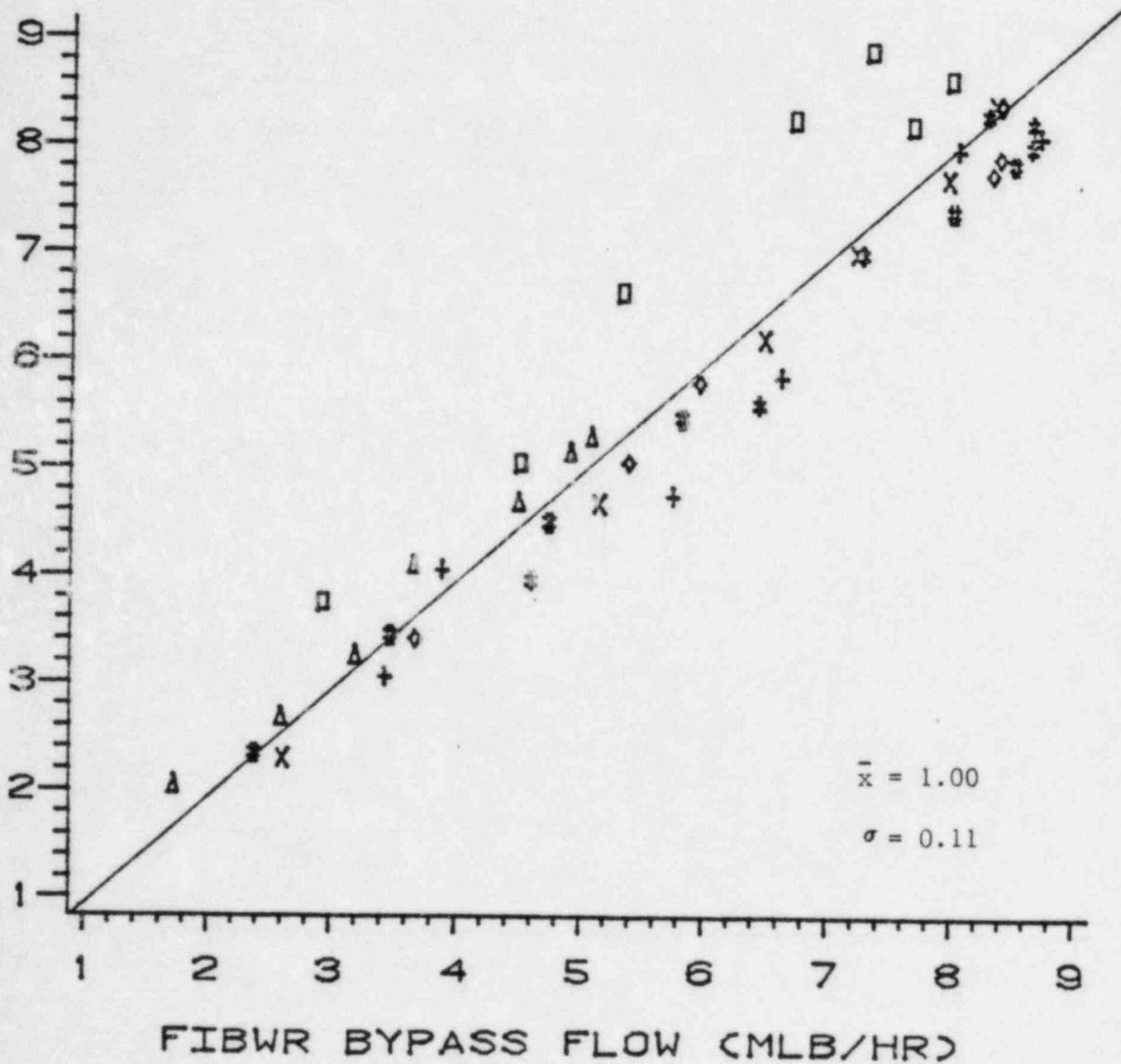
$$\bar{x} = \frac{\text{BYPASS FLOW (pc)}}{\text{BYPASS FLOW (FIBWR)}}$$
