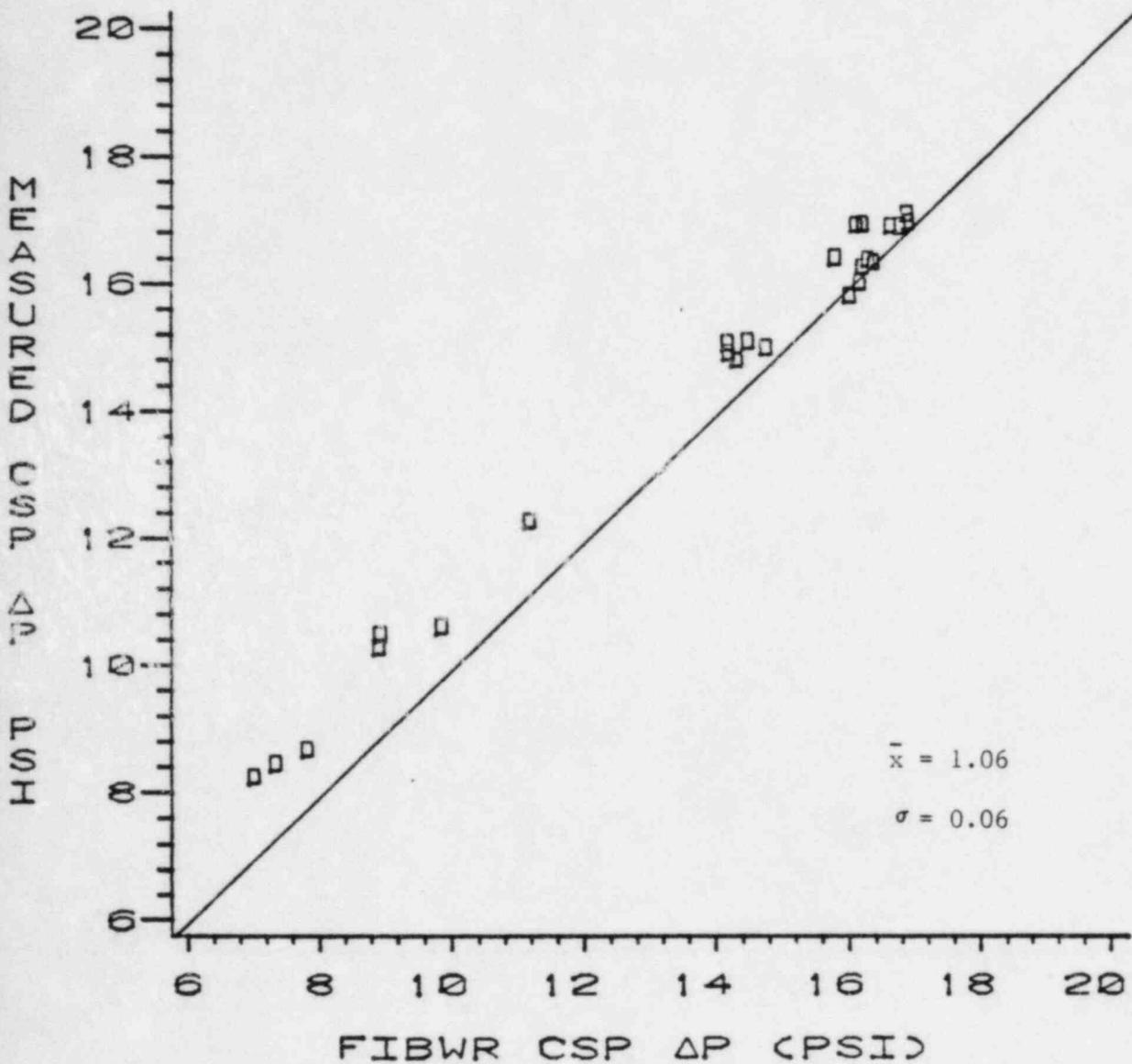
$$\bar{x} = \frac{\Delta P \text{ measured}}{\Delta P \text{ FIBWR}}$$
