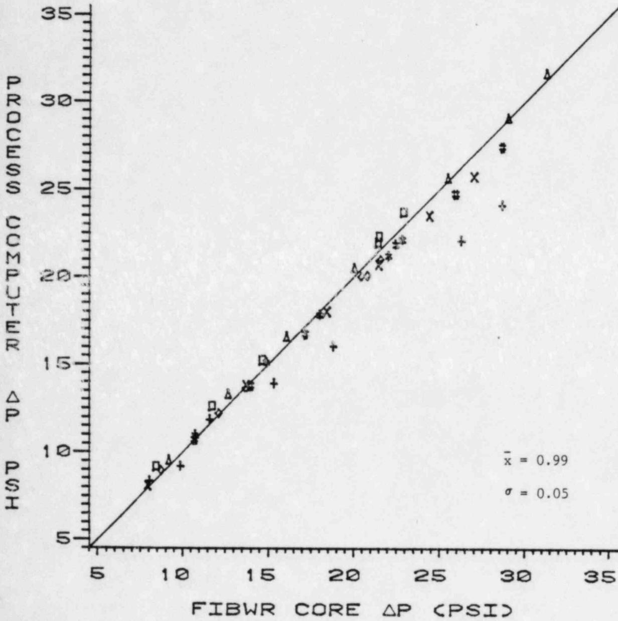
$$\bar{x} = \frac{\Delta P \text{ process computer}}{\Delta P \text{ FIBWR}}$$
