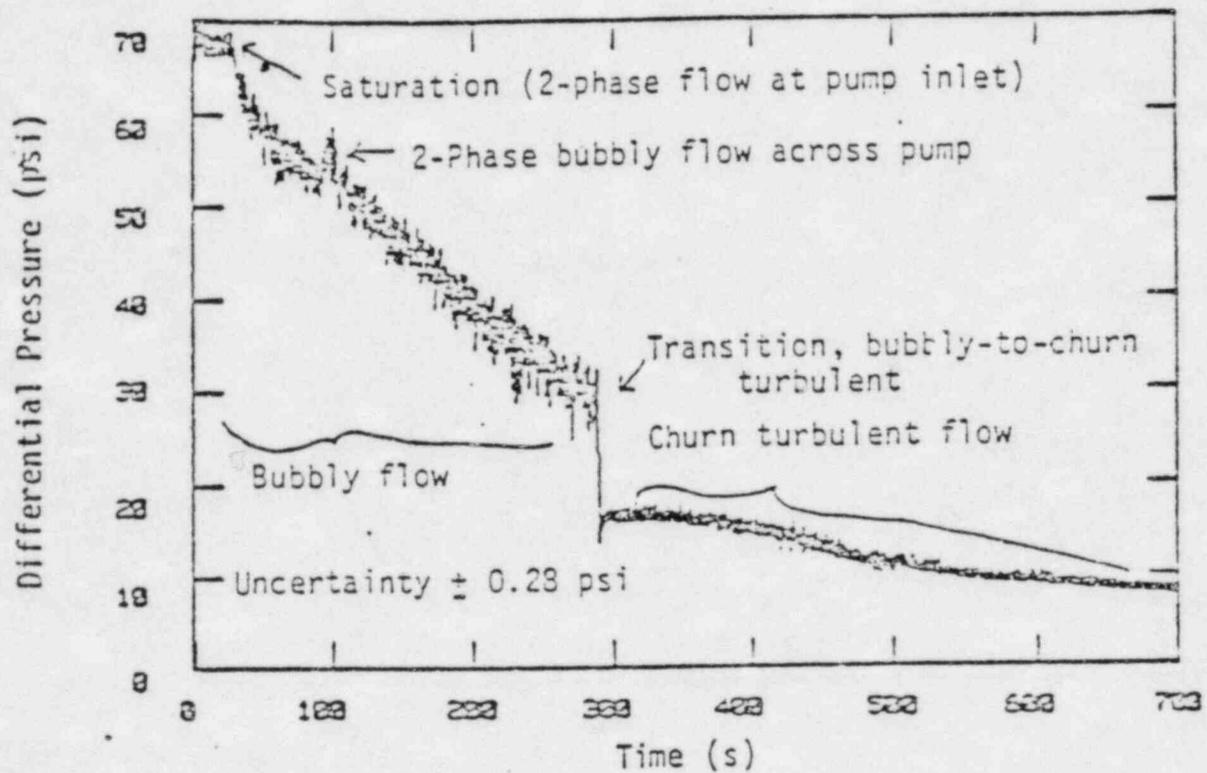
Figure 10: Differential Pressure Across Primary Coolant Pumps
