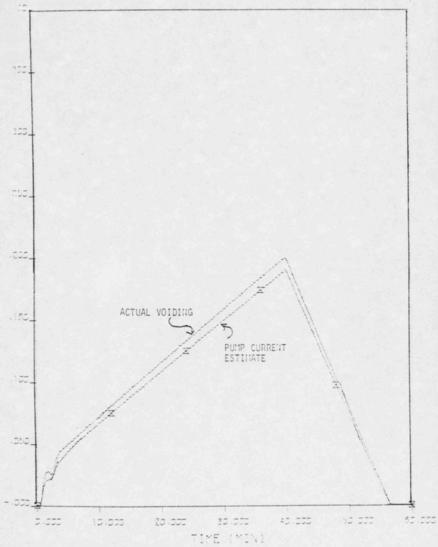
FIGURE 17: VOID FRACTION VS TIME (NON-DEGRADED)
