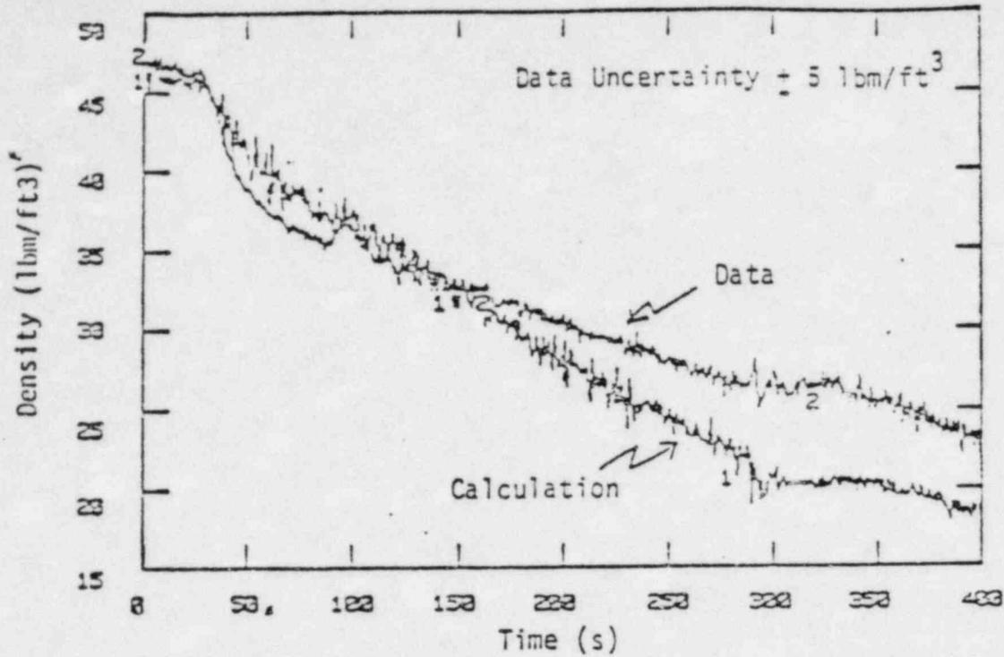
Figure 11. Measured Density Upstream of Pump Compared With Prediction Using Pump Motor Power Assuming Constant Volumetric Flow and Pump Head
