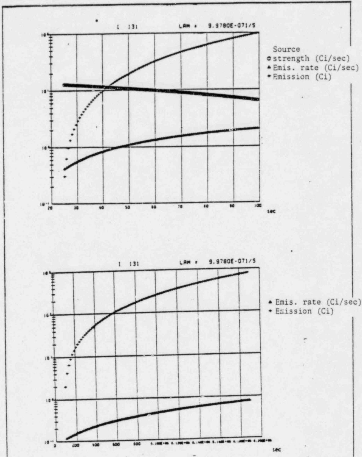
Figure 6.3.1. Emissions or Emission Rates of Accident According to Scenario 2. To the extent given, the source strength is the product of time-dependent primary concentration and time-dependent leak rate.
