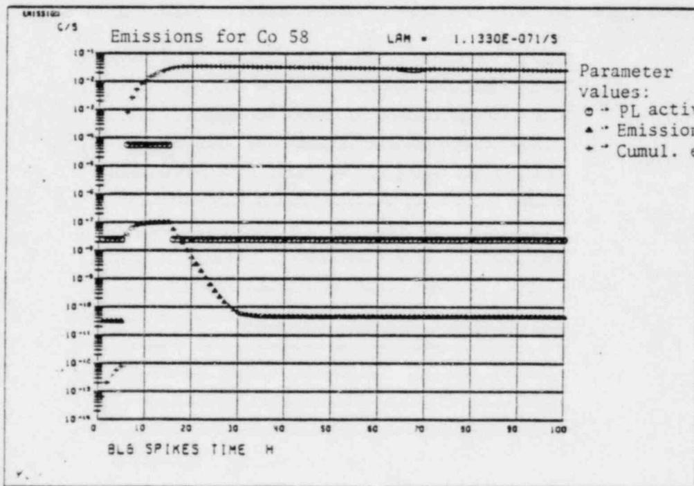
Figure 4.6.6./7. Block 6 - Spike Computation and Load Change Emission Computations for Co-58 with Medium Spike Factor ( $2.2 \cdot 10^3$ , Upper Figure) and Maximum Spike Factor ( $10^4$ , Lower Figure) at a Load Change of 100% to 85% in 20 Hrs.
