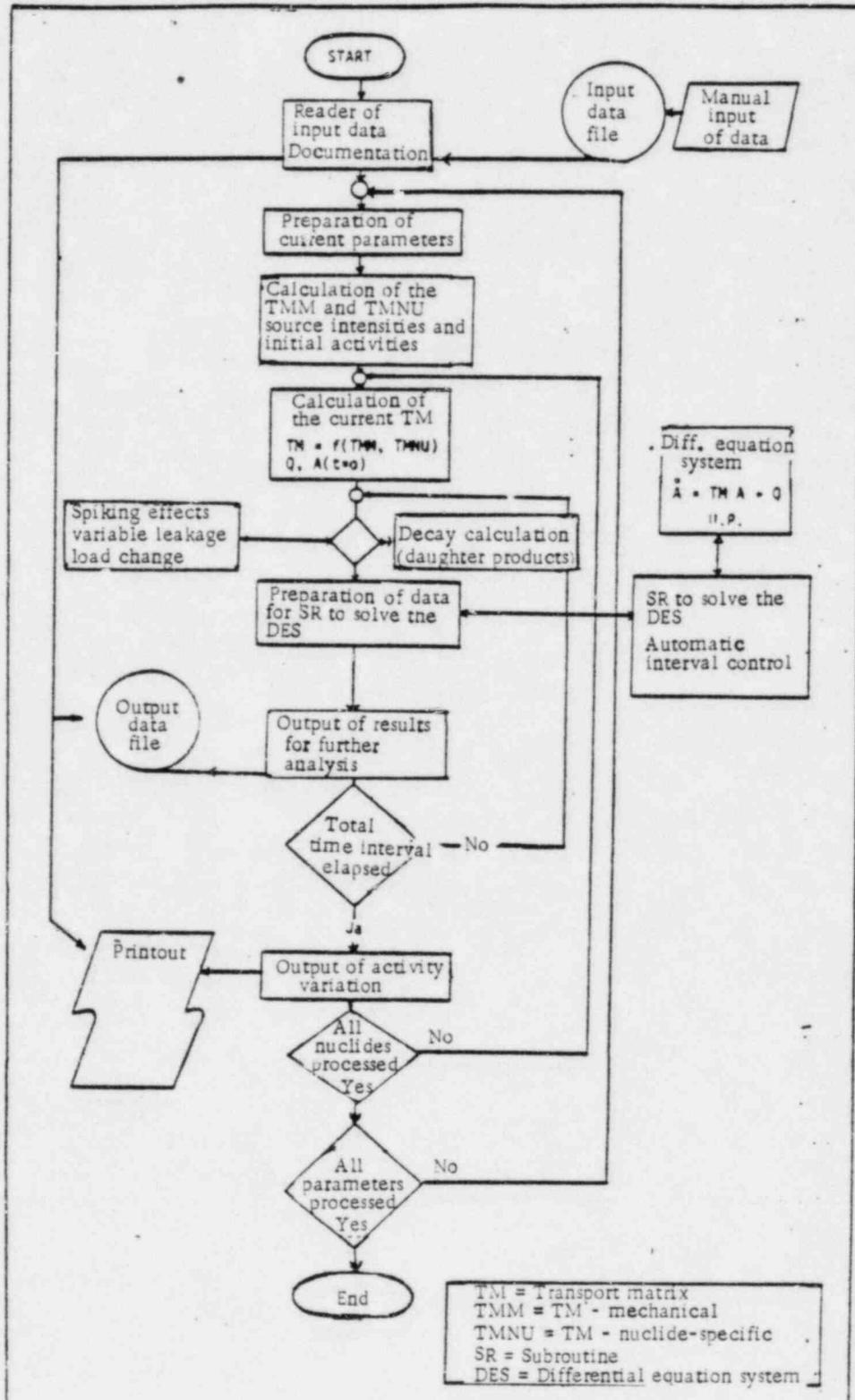
Figure 3.2. Schematic Block Diagram of the SEKEM4 Computer Program.
