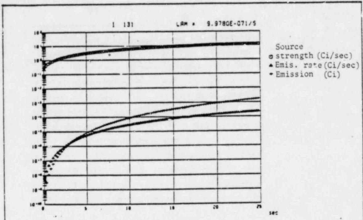
Figure 6.3.1. Emissions or Emission Rates of Accident According to Scenario 2. To the extent given, the source strength is the product of the time-dependent primary concentration and time-dependent leak rate.
