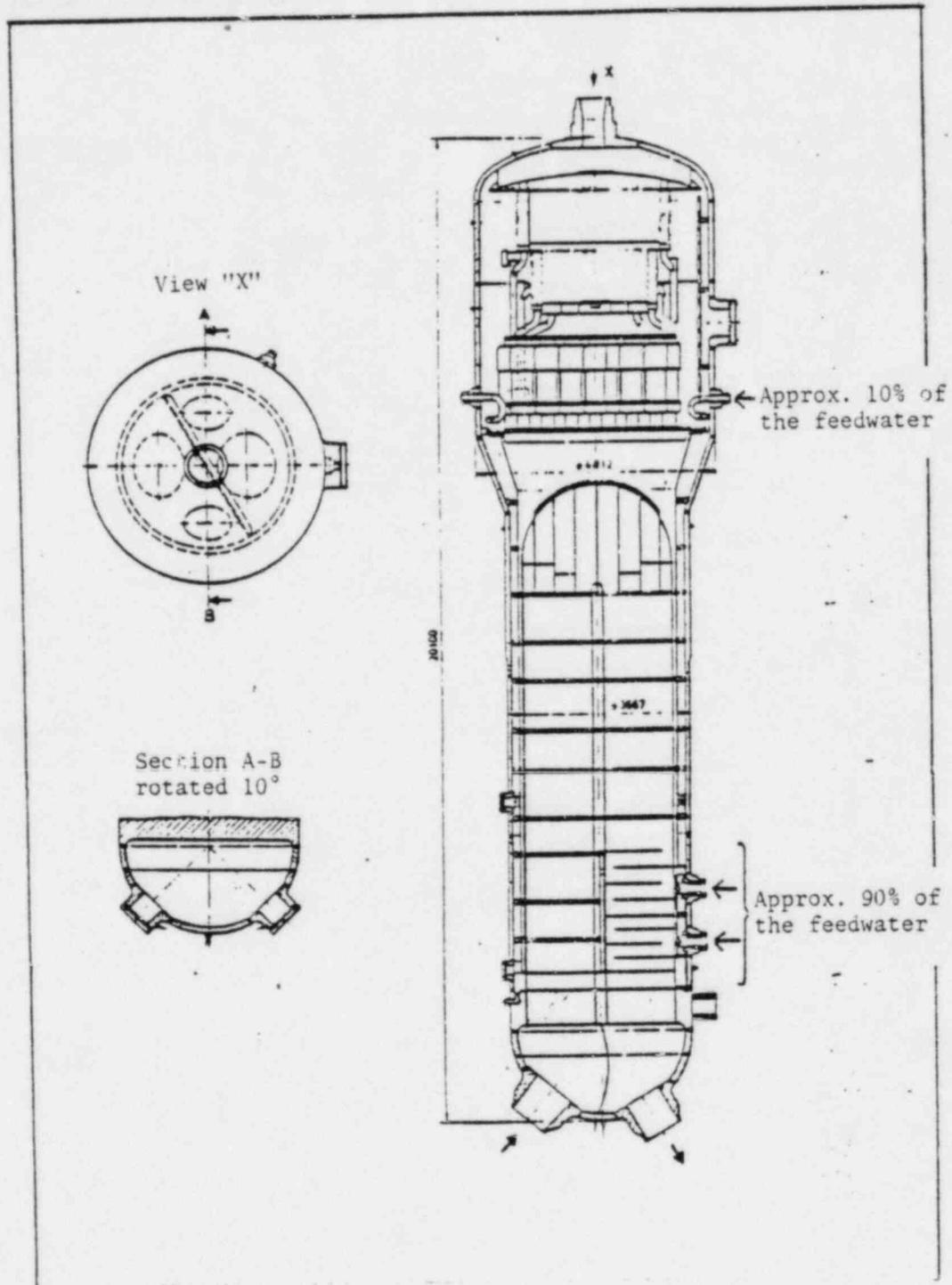
Figure 2.4.2. Standard Steam Generator 54 GS.
