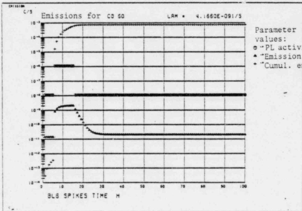
Figure 4.6.4./5. Block 6 - Spike Computation and Load Change Emission Computations for Co-60 with Medium Spike Factor (100, Upper Figure) and Maximum Spike Factor (500, Lower Figure) at a Load Change of 100% to 85% in 20 Hrs.
