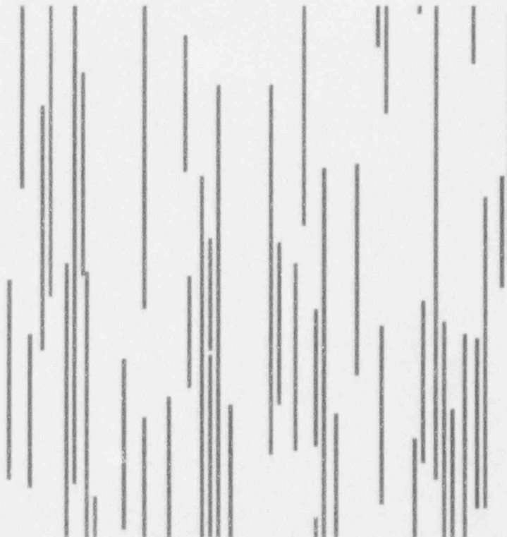
Figure 2-17. Set of vertical fractures used for network generator verification. Dimensions of the bounding box are 256 \times 256 length units.
