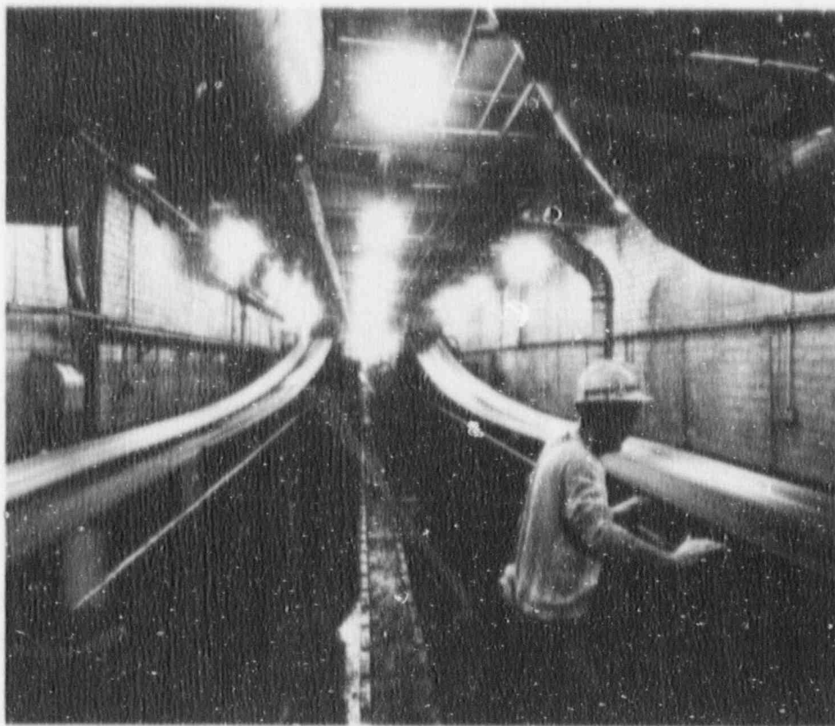
At North Omaha Station, coal is carried by conveyor belts to pulverizers that grind it down to the consistency of face powder. It is then mixed with preheated air and blown into the furnace, where it ignites and burns instantly in midair.
