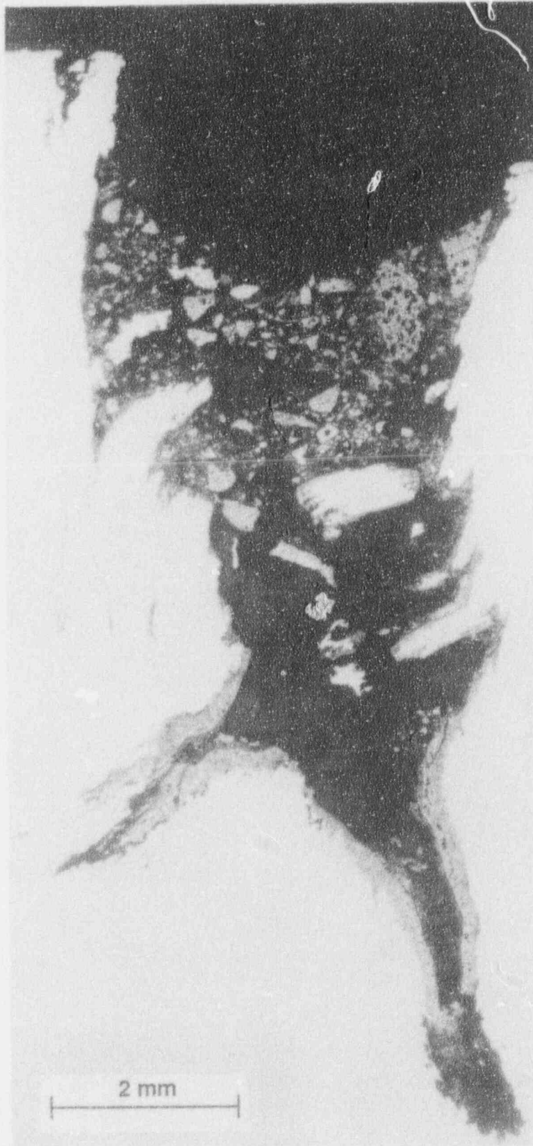
Fig. 9. "Bottom" end of large crack shown in Fig. 8, showing fuel debris in an Fe-oxide matrix.
