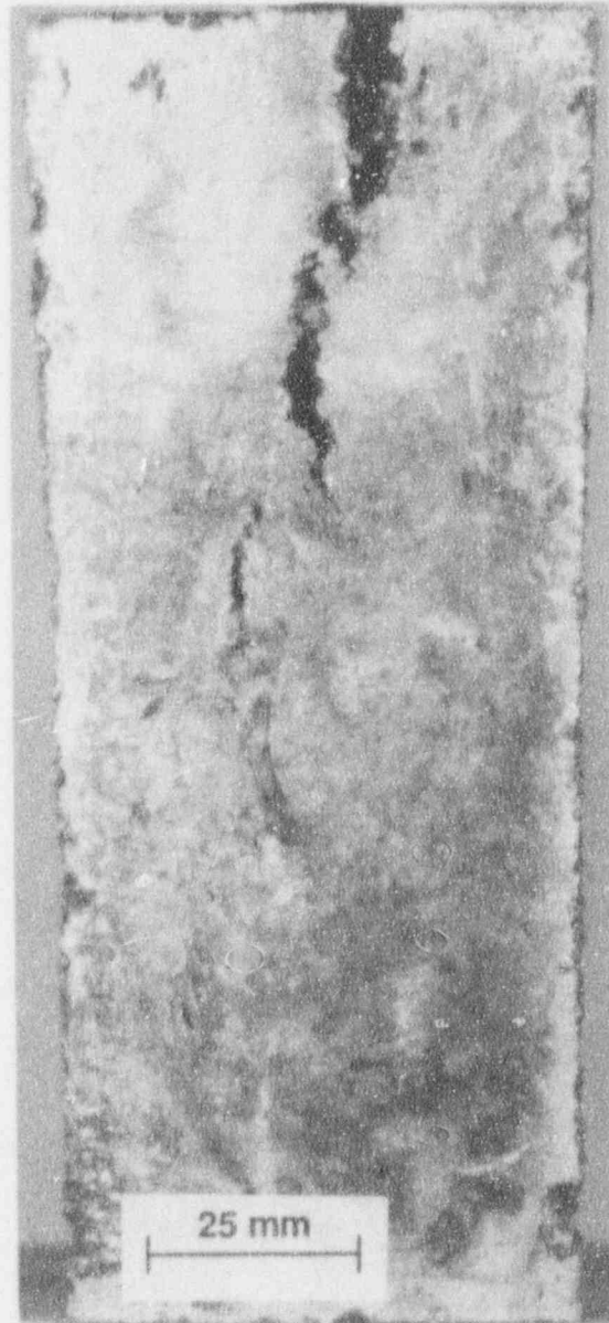
Fig. 5. Surface of Sample E-6 showing end of one leg of crack around Nozzle E-7. MCT 276674
