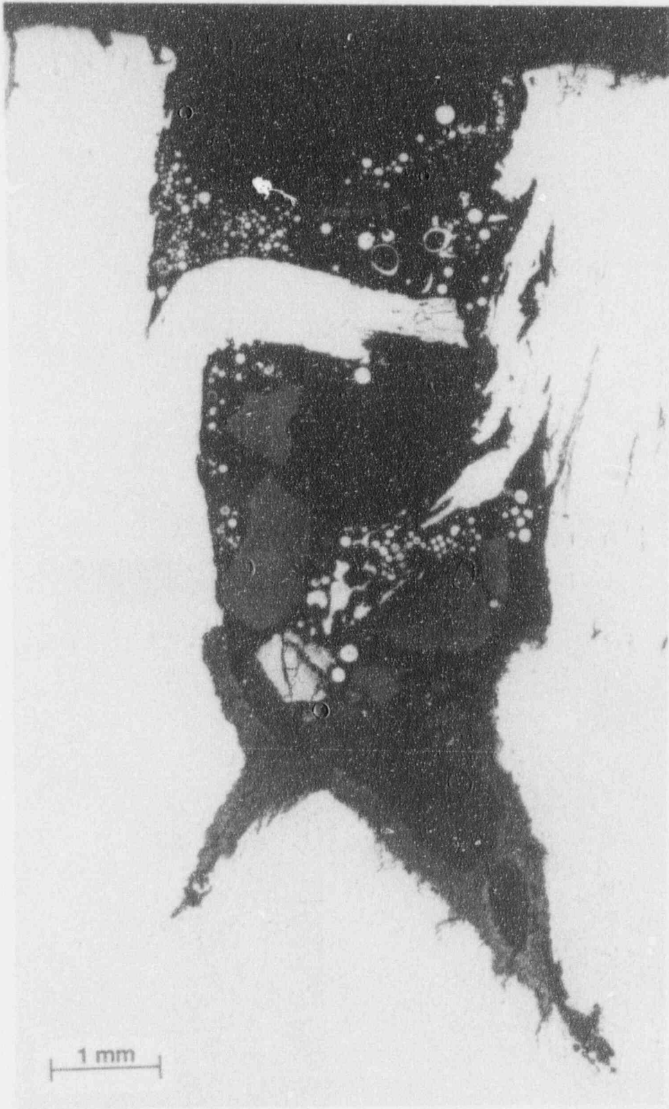
Fig. 10. Cross section through small crack in G-8. Gray masses are U-Zr "fuel;" white spheres are Fe from cutting operations.
