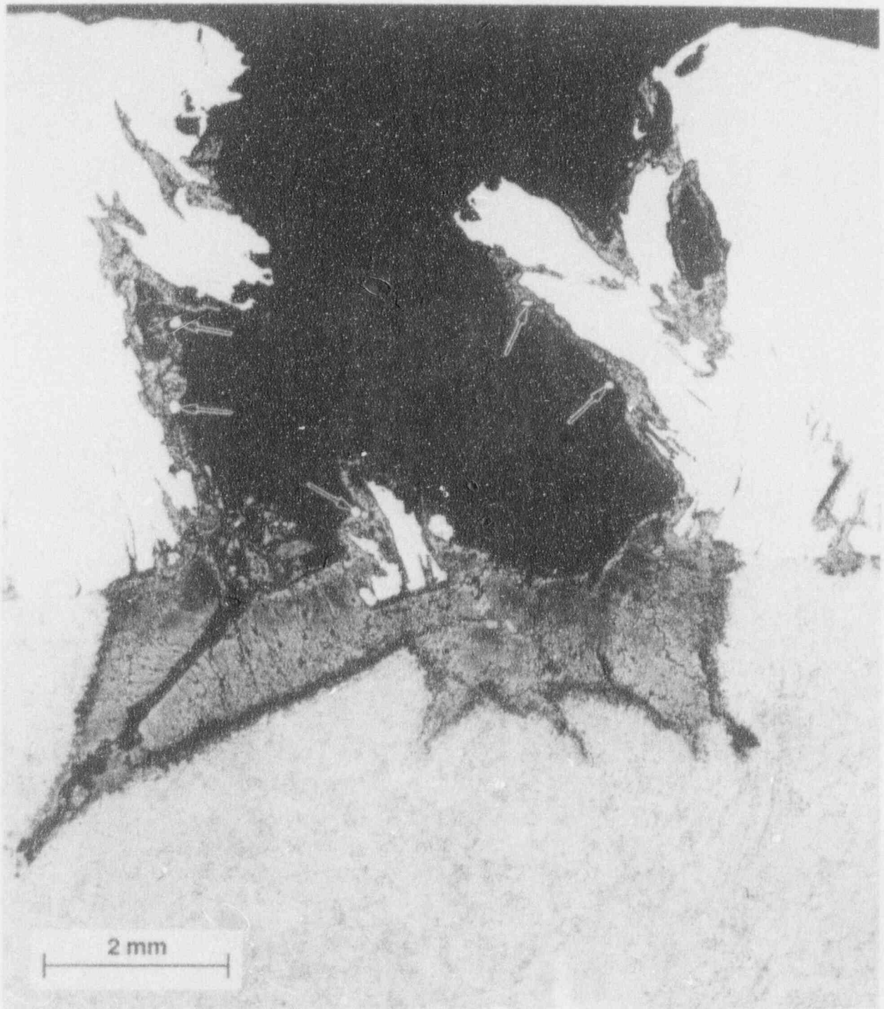
Fig. 6. Cross section through principal crack in Sample E-6. Arrows identify larger Ag-Cd nodules. Etched.
