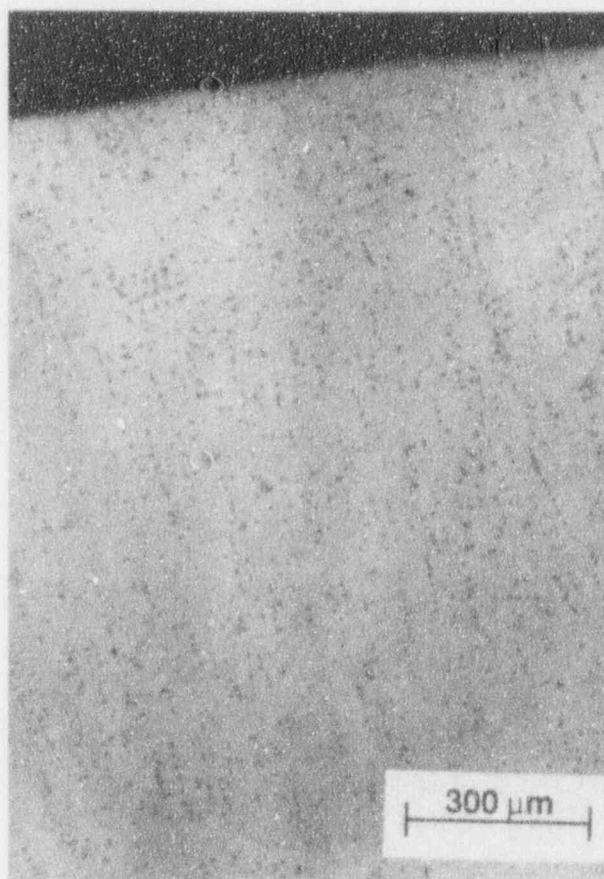
Fig. 17. Metallographic specimen from lower head Sample E-8 showing spheroidization of delta ferrite phase in cladding. (From Ref. 5)
