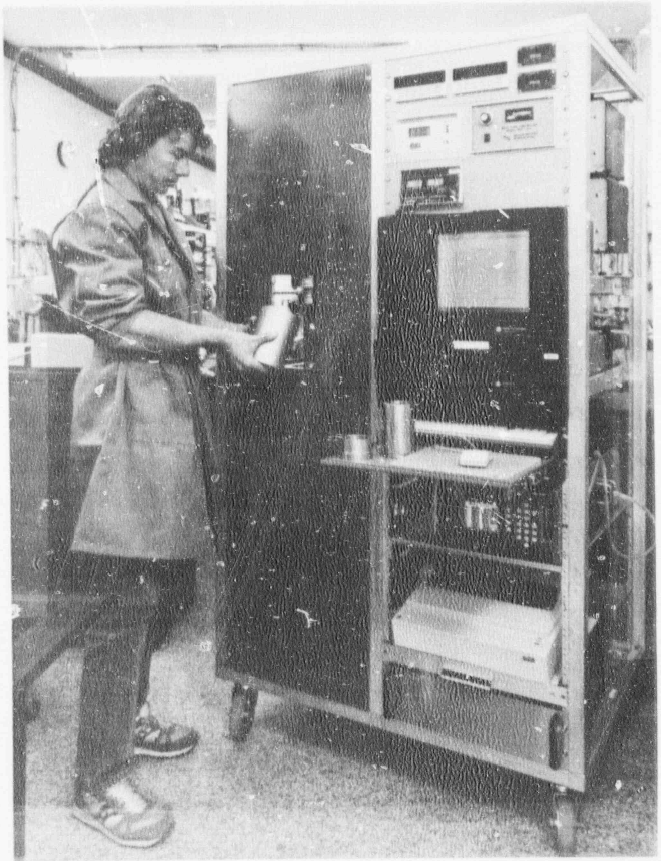
Figure 14 Operator installing prototype steel filter in LLNL automated filter tester.
