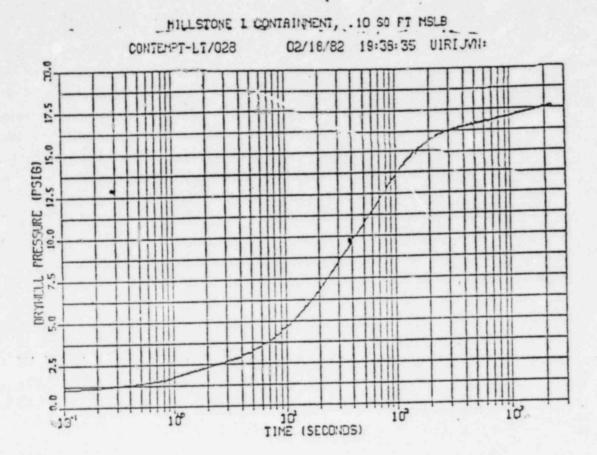
Figure 10. Drywell Pressure Response to a 0.10 ft<sup>2</sup> MSLB
