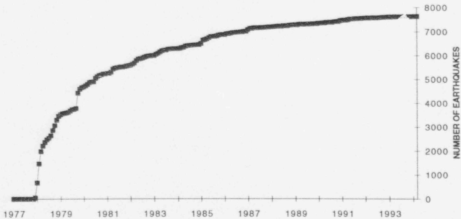
Figure 4. Cumulative seismicity near Monticello Reservoir since impoundment.
