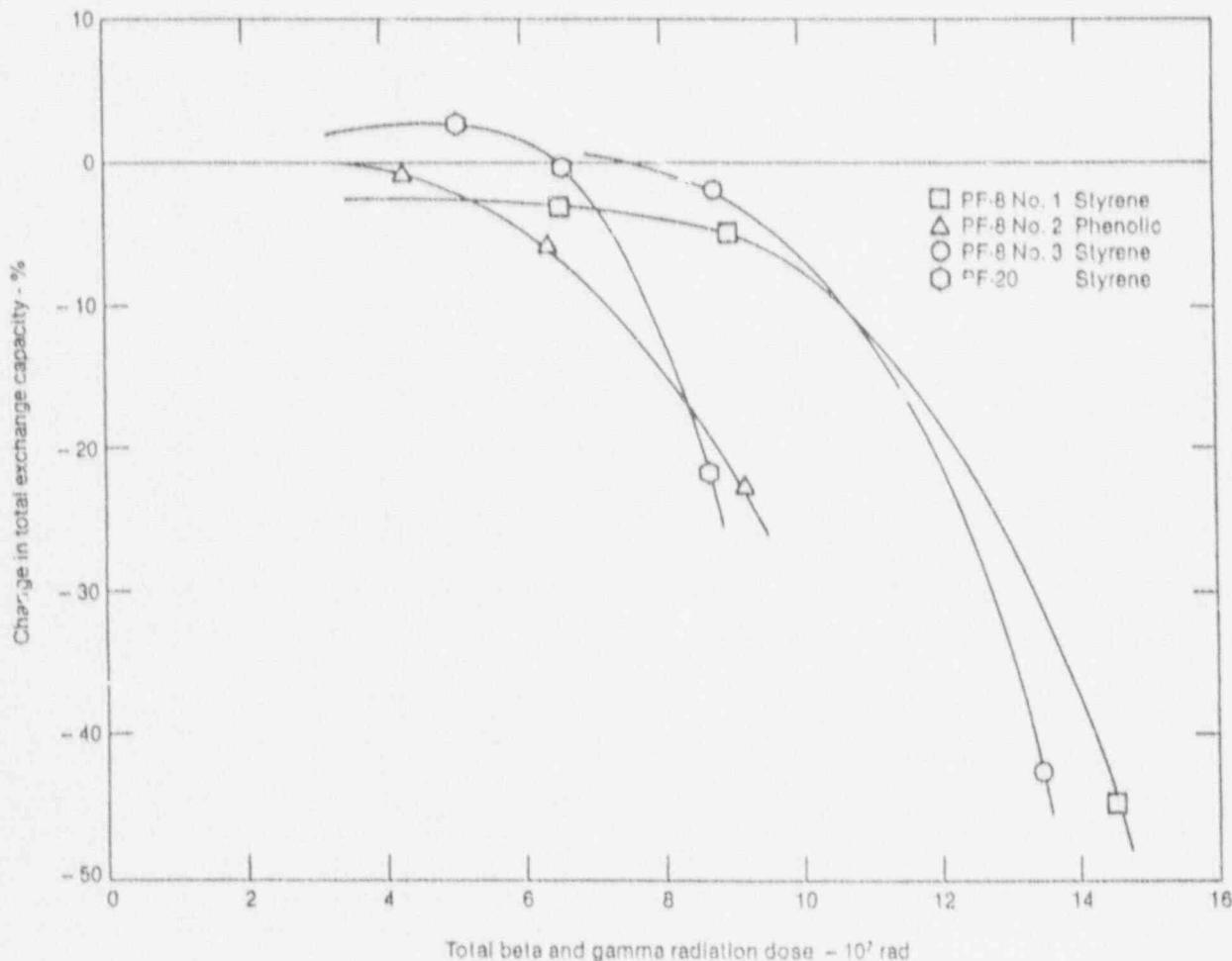
Figure 1. Change in total exchange capacity with increase in radiation dose.
