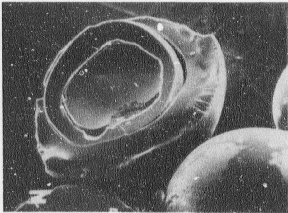
**Figure 2.** SEM photomicrograph of EPICOR-II strong acid cation resin sample from PF-8#1 showing a closeup of one unusually damaged bead (at 100 magnification).
