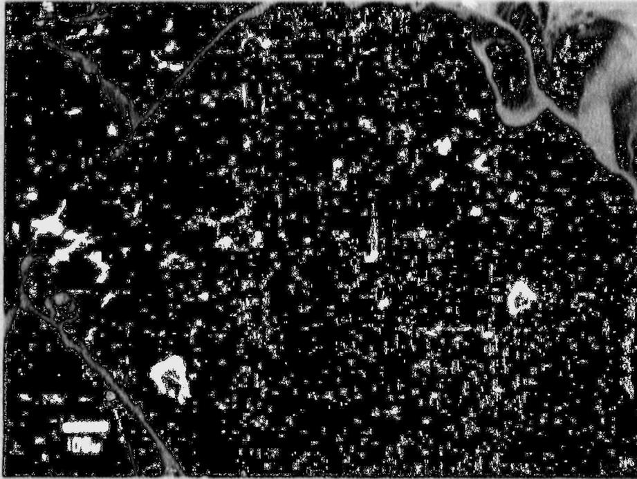
**Figure 5.** SEM photomicrograph of EPICOR-II phenolic cation resin sample PF-8#2 showing a closeup of one cracked resin particle (at 50 magnification).
