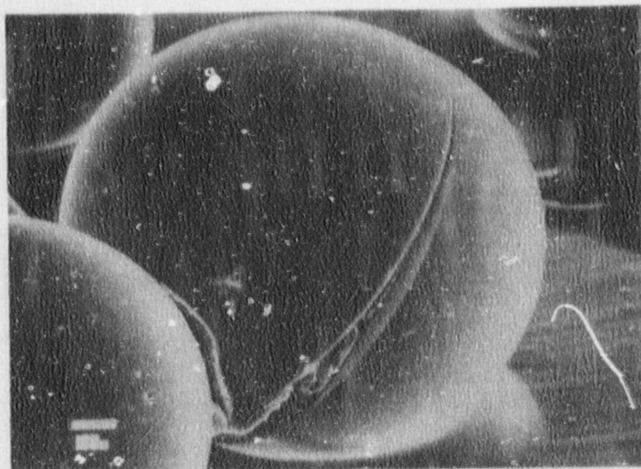
**Figure 4.** SEM photomicrograph of EPICOR-II strong acid cation resin sample PF-20 showing a closeup of a damaged resin bead (at 100 magnification).
