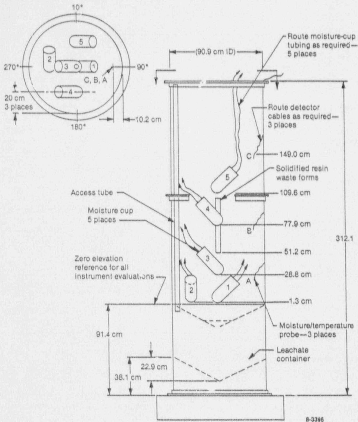
Figure 11. EPICCR-II lysimeter vessel component locations.
