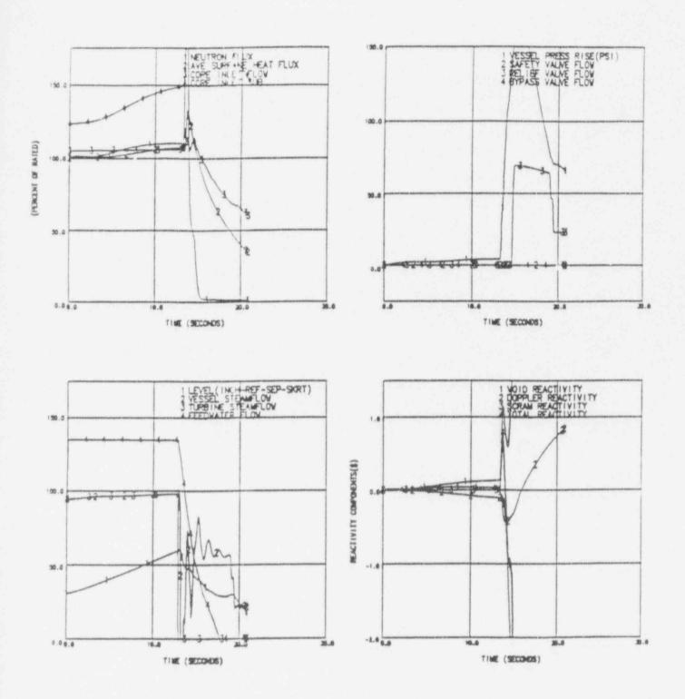
Figure 4. Plant Responses to Feedwater Controller Failure, Maximum Demand, 100P/105F, FWTR, TBP-OOS
