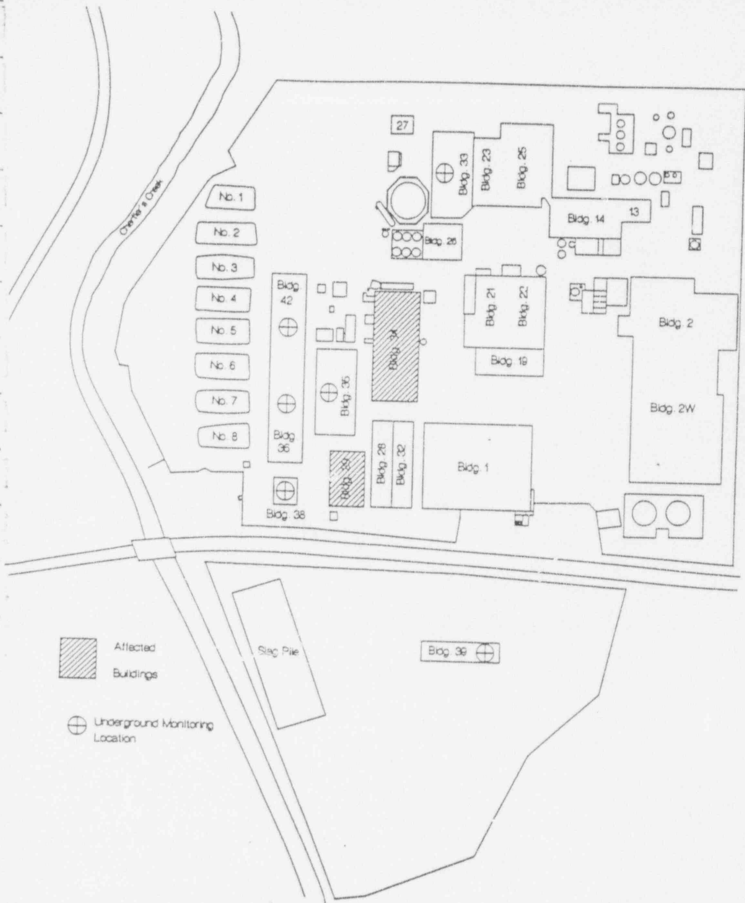
Figure 5-3: Buildings at MolyCorp, Washington Pa Plant Site which, Due to Historic Usage Patterns, May Be Classified as 'Affected Buildings'
