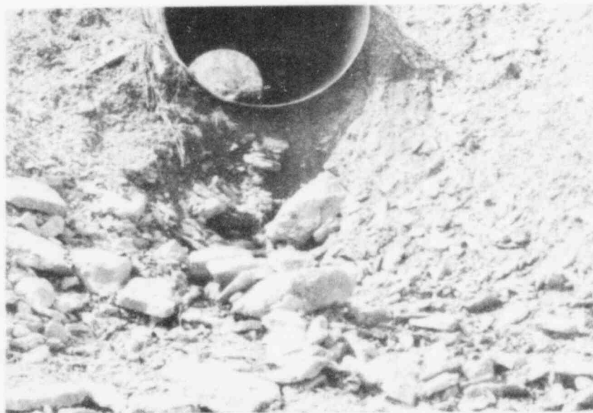
Figure A-30. Downstream sedimentation study rod at Station 8, 12 November 1981. No noticeable sediment accumulation.
