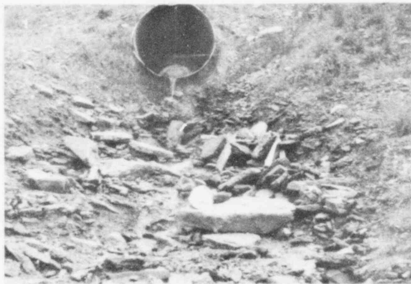
Figure A-28. Downstream sedimentation study site at Station 8, 25 May 1981. No noticeable accumulations.
