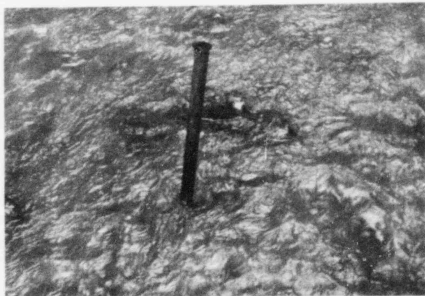
Figure A-36. Downstream sedimentation study rod at Station 6, 25 May 1981. No measureable sediment accumulation since March, but there was evidence along the banks that sediment had once been deposited. Rocks were scoured and algae had disappeared.
