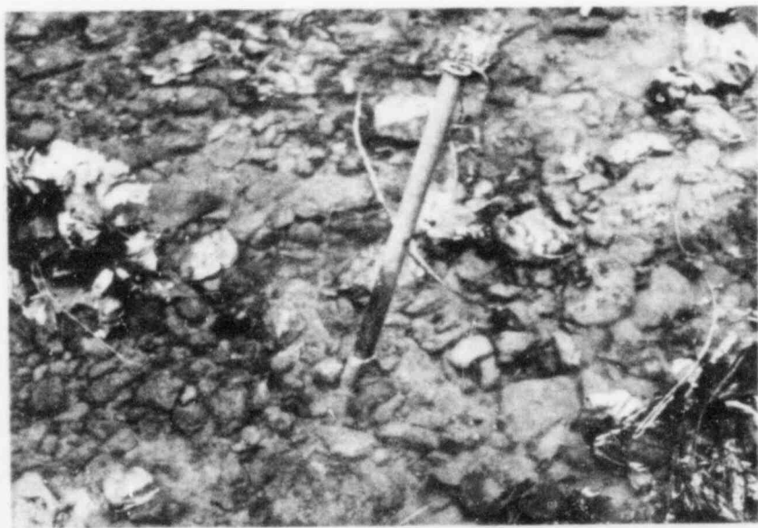
Figure A-37. Downstream sedimentation study rod at Station 6, 10 August 1981. Approximately 1 cm of sediment had accumulated since May. Note spaces between rocks filled in with sediment.
