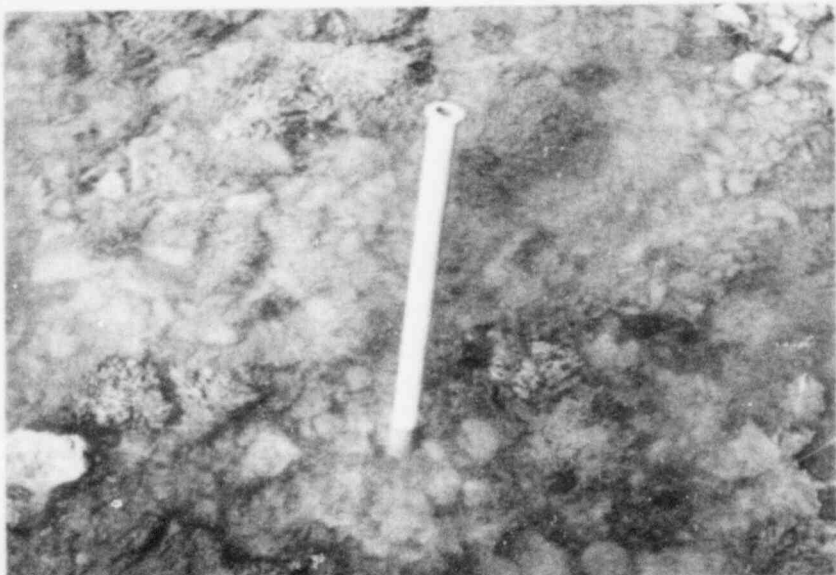
Figure A-35. Downstream sedimentation study rod at Station 6, 23 March 1981. No measureable sediment accumulation since November 1980. Note extensive algal growth.
