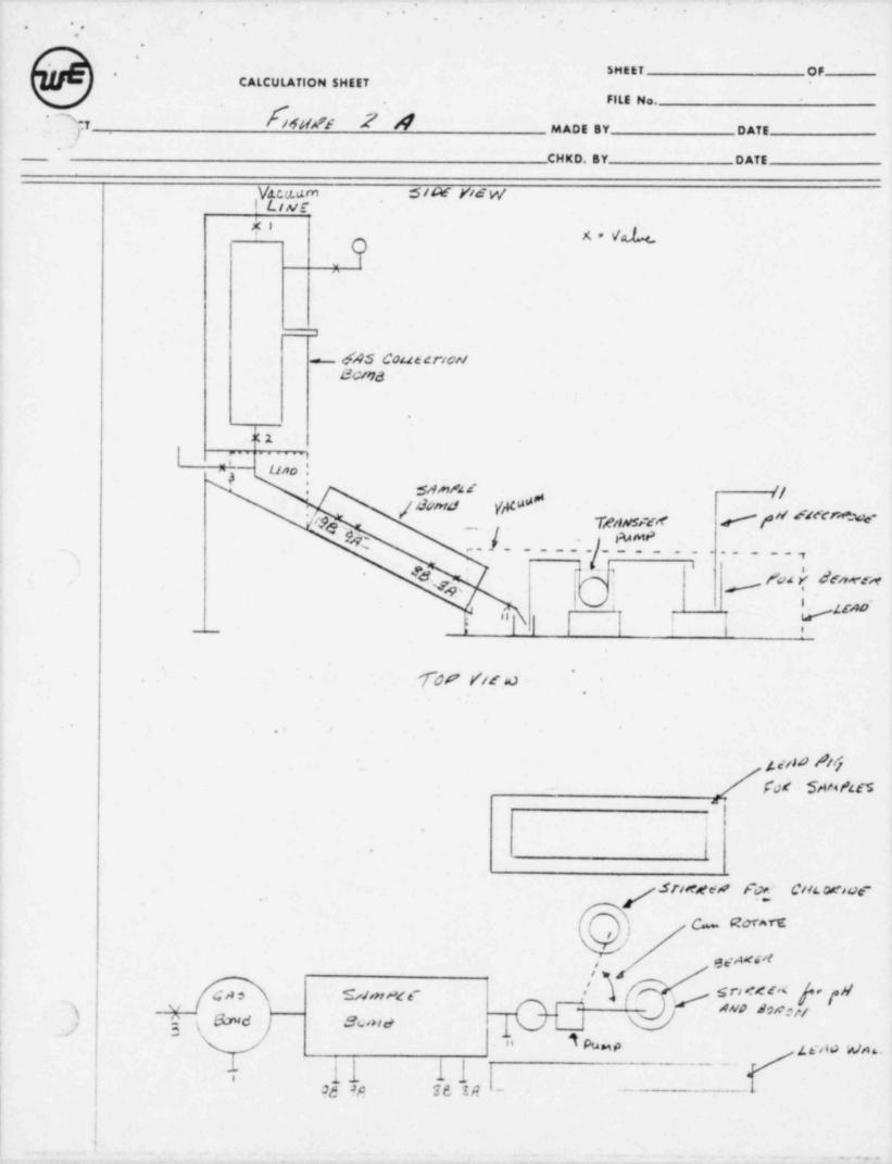
Chemical Transfer Plump n the aveas between Note : All value handle are L to plane of the gare : Lend briek should should 0 am h be placed the shiel mond aren Sample bomb 37 sot. Pressure Sample Gas Collection bomb \$7 Vent line est. Por Support 0  $\otimes$ Vacuum П m 200-Support -1 dn 06/8/1 25th 31AG HHO CHKD. BA 08/8/1 tray ving San 31AQ 519 Y8 JOAM EILE No. CALCULATION SHEET 10 SHEET 8 2 ranky
