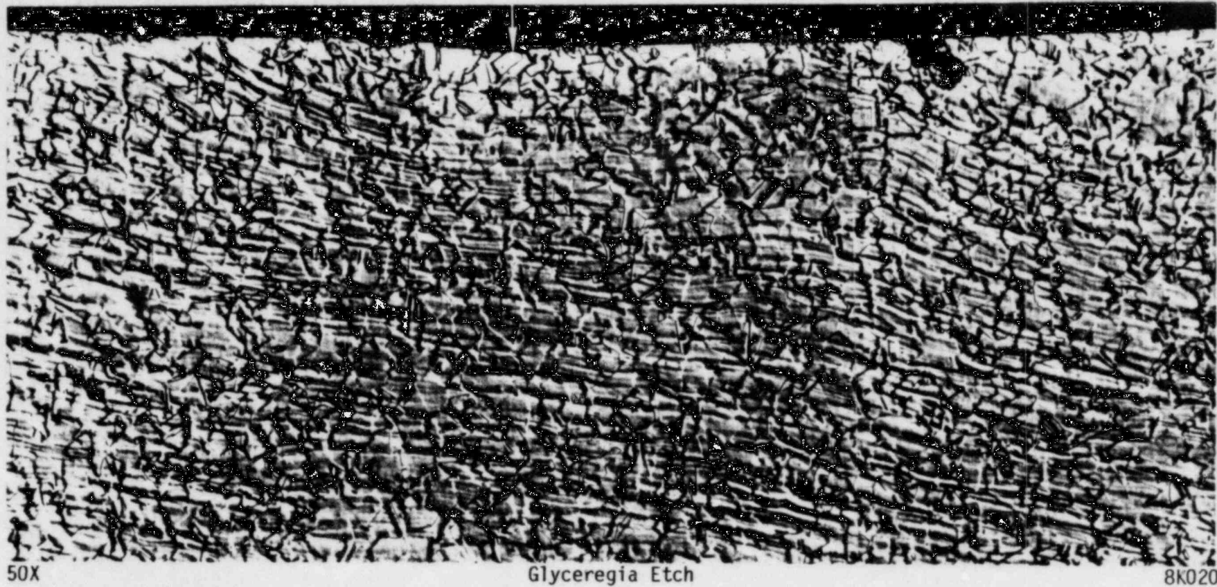
FIGURE 8. THE FLOW PATTERN OF METAL AROUND SURFACE FLAW NO. 2 OBSERVED IN SPECIMEN 2-P-P
