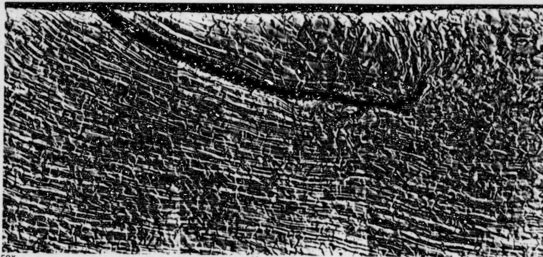
FIGURE 9. THE FLOW PATTERN OF METAL AROUND SURFACE FLAW NO. 2 IN SPECIMEN 2-N-N
