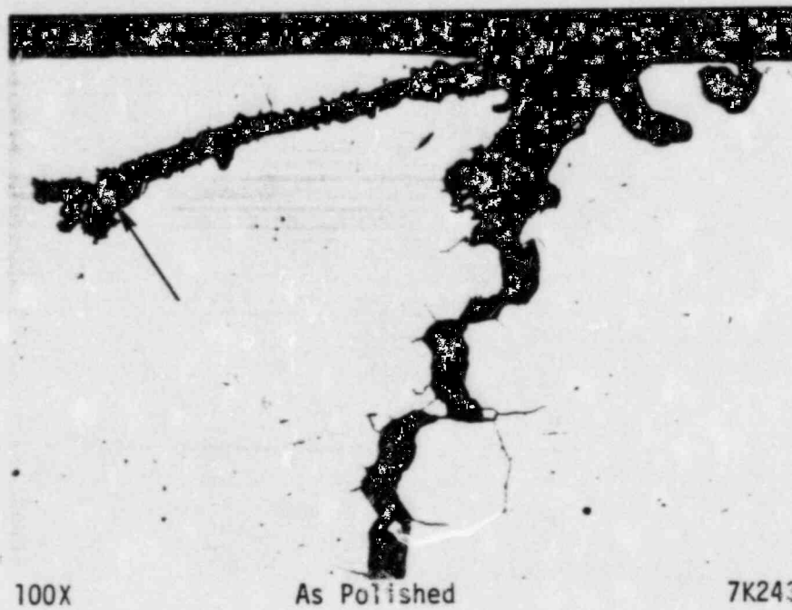
100X As Polished 7K243 FIGURE 13. CROSS SECTION OF FLAW NO. 1 IN SECTION 1-S-S The arrow identifies the corrosion products in Flaw No. 1 (Area 3 in Table 4) that were subjected to EDAX analyses.
