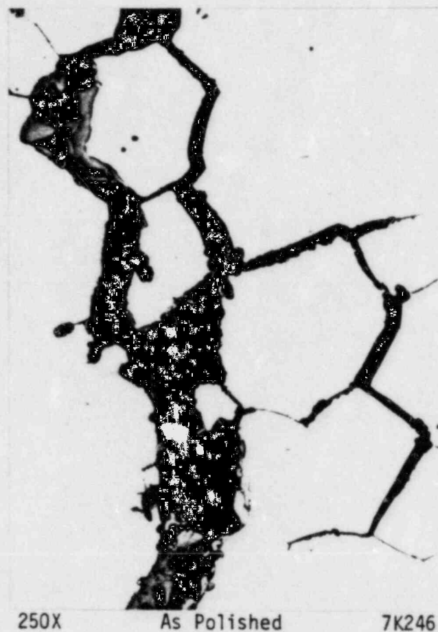
FIGURE 7. TYPICAL REGION OF THE INTERGRANULAR CRACK THAT WAS LOCATED WITHIN CIRCLED AREA 3 IN FIGURE 5a
