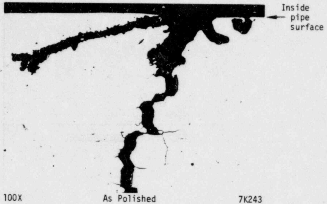
FIGURE 6. CROSS SECTION OF THE LINEAR DEFECT WITHIN CIRCLED AREA 2 IN FIGURE 5a
