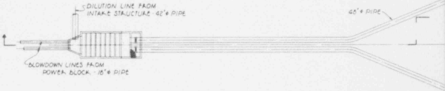
PLAN - OUTFALL STRUCTURE
