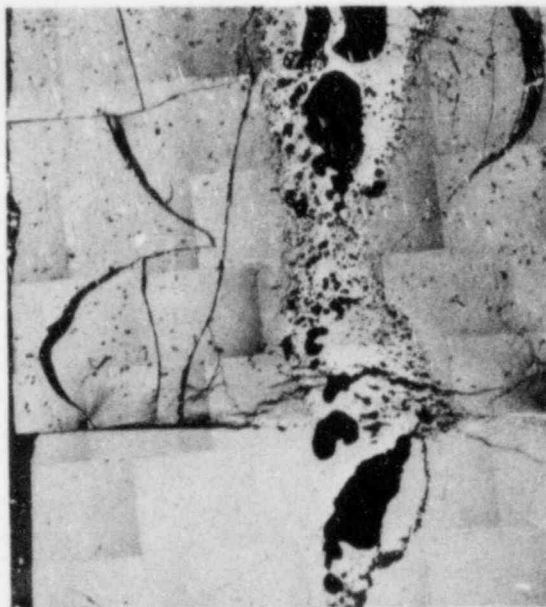
Fig. 25. Longitudinal Section through the Test 21 Specimen Showing Microcracking in the High-burnup Fuel (Top) and the Absence of Microcracking in the Depleted- \text{UO}_2 Spacer Pellet. Neg. No. MSD-188347.
