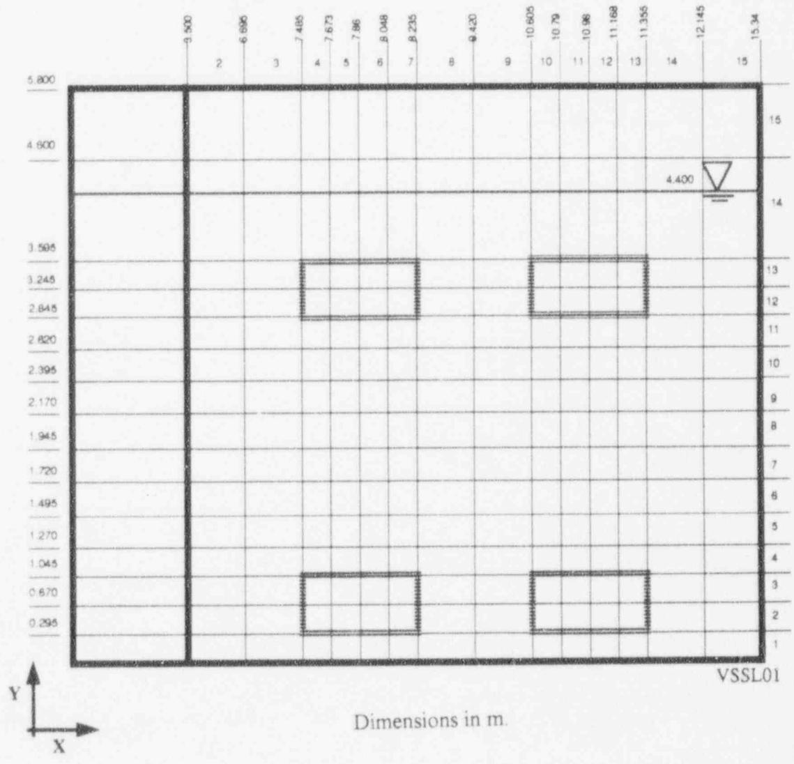
Figure 3-2 Nodalization of Condenser Pool
