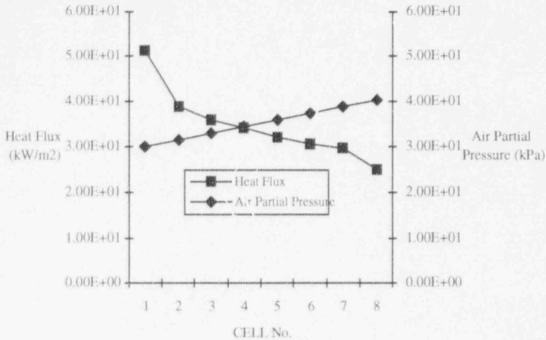
Figure 4-4 Heat Flux and Air Partial Pressure in PIPE 97 - Case 5
