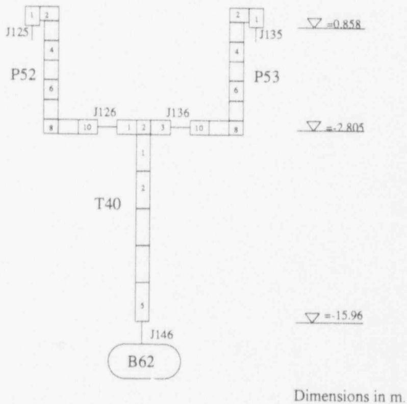
Figure 3-7 Nodalization of Vent Line
