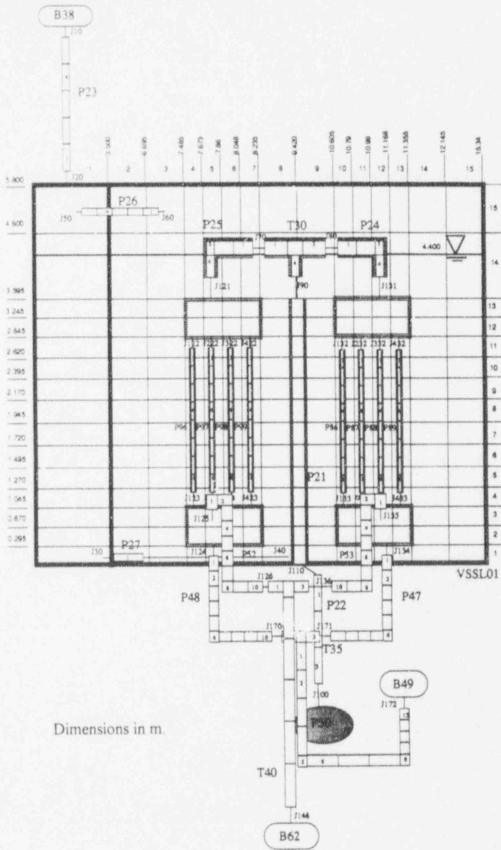
Figure 3-1 Composite Nodalization for PANTHERS TRACG Model
