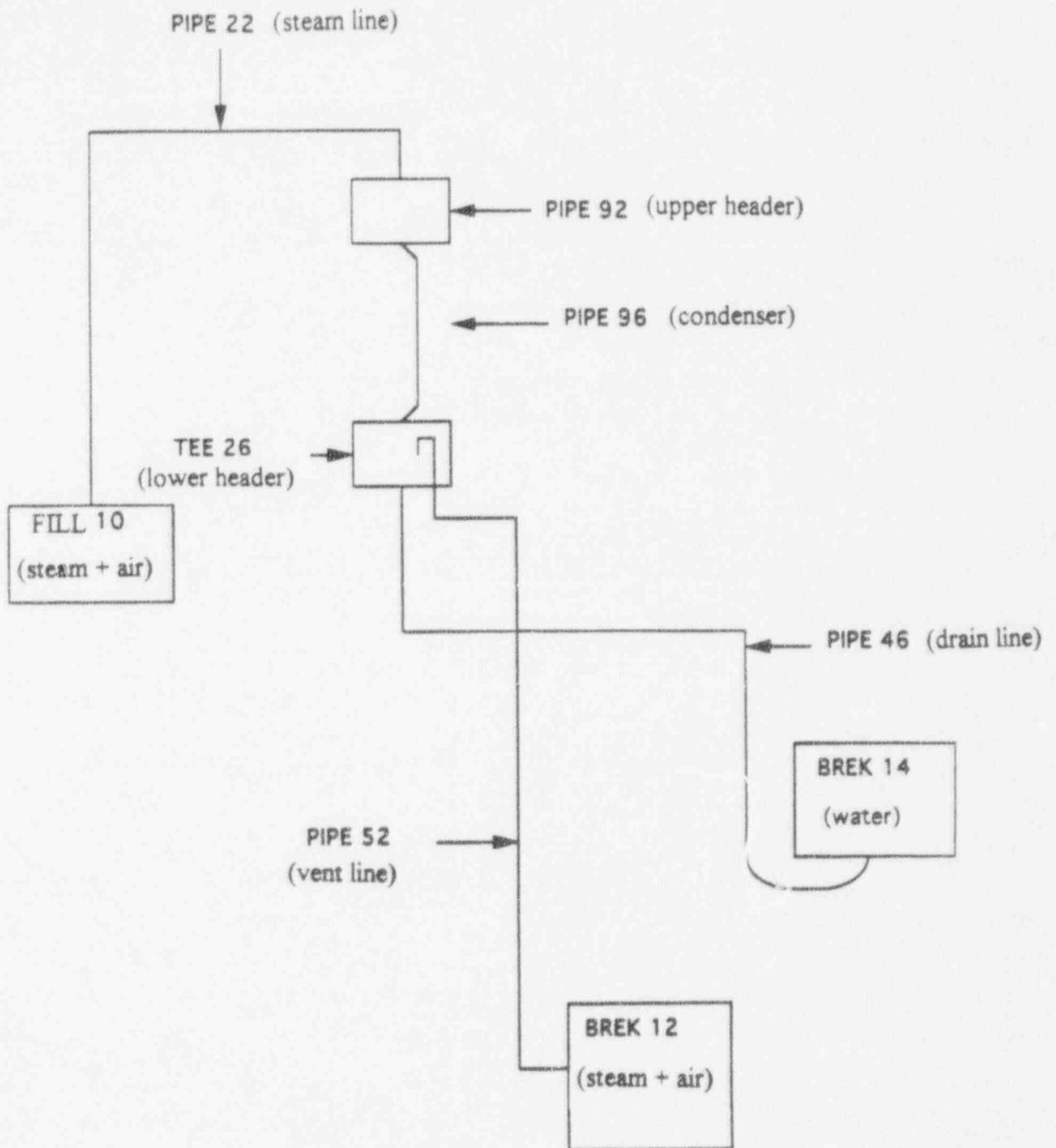
Figure 3-8 Schematic of SBWR Containment PCC Model
