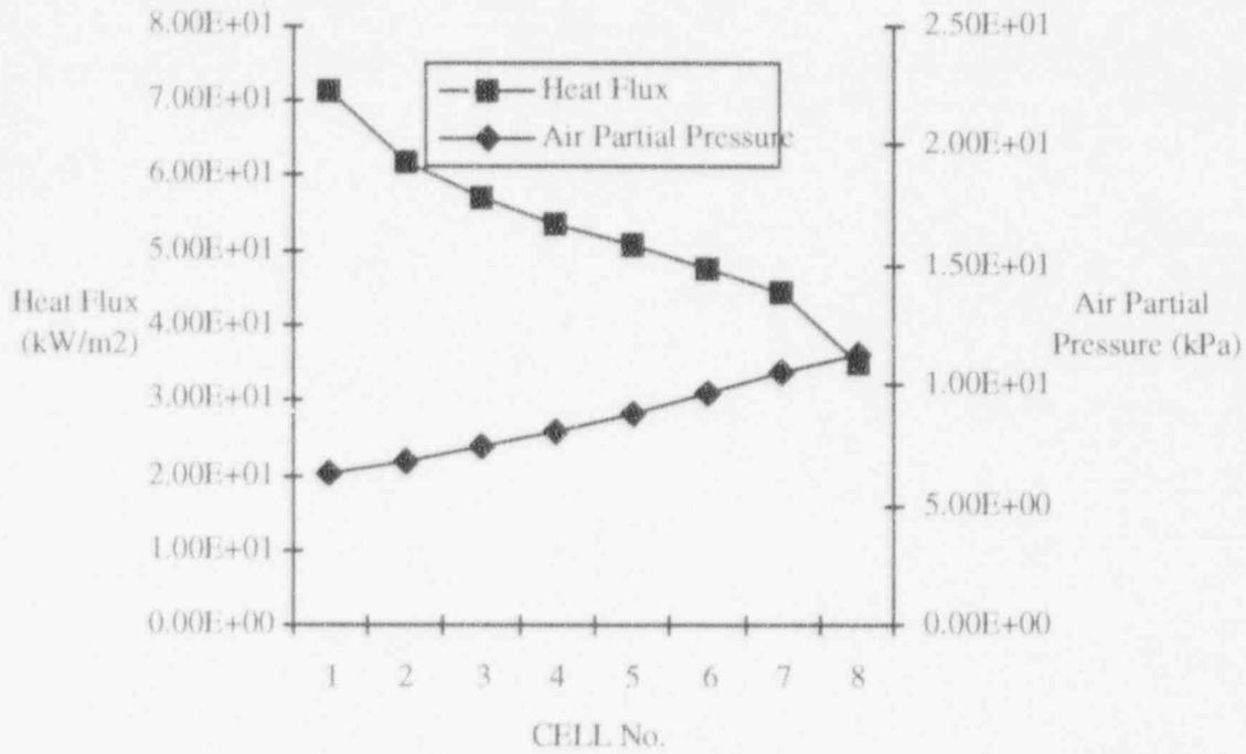
Figure 4-2 Heat Flux and Air Partial Pressure in PIPE 97 - Case 3
