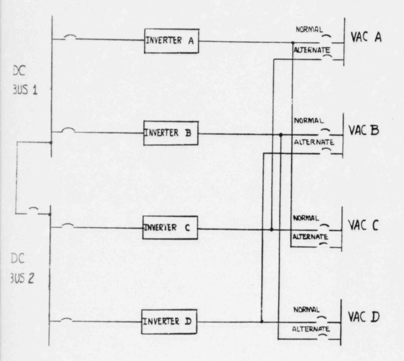
CONNECTICUT YANKEE PROPOSED DC BUS / VITAL AC BUS ARRANGEMENT
