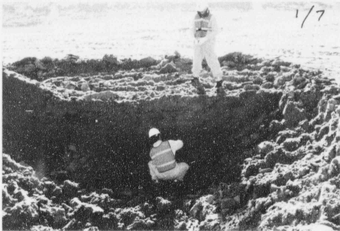
TP M-CF-04. The top five feet of the test pit is in tailings. Personnel are collecting tailings samples for radiological analysis.
