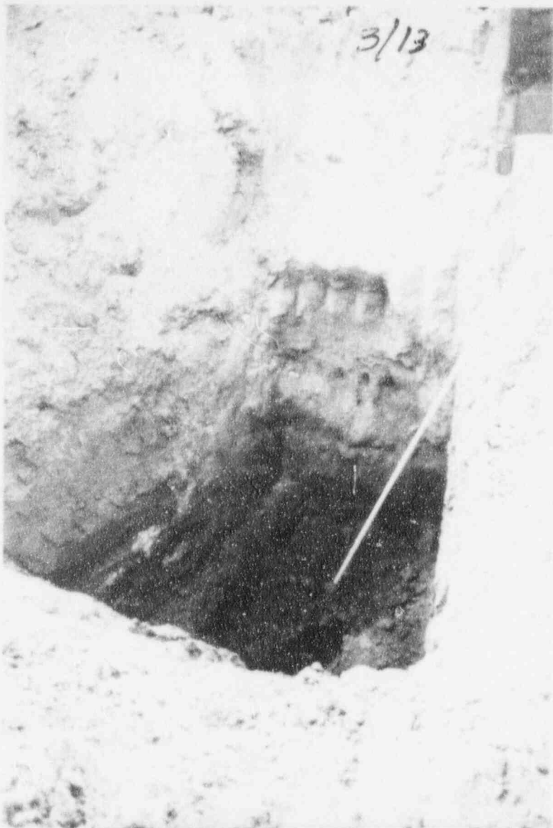
TP M-CF-03. Very dry soil overlying gravels. Note black carbonaceous coating on gravels.
