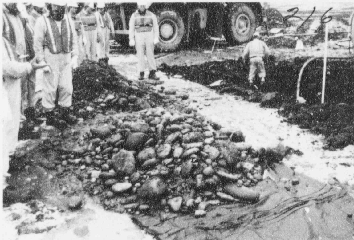
TP M-CF-25. Sample obtained from below the water table (Note how fines have been removed by the flushing action of the water when the water drains out of the sample).
