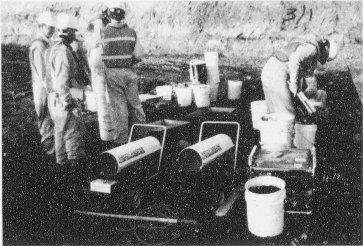
Drying and screening gravel (Cobbles and Fines) samples.
