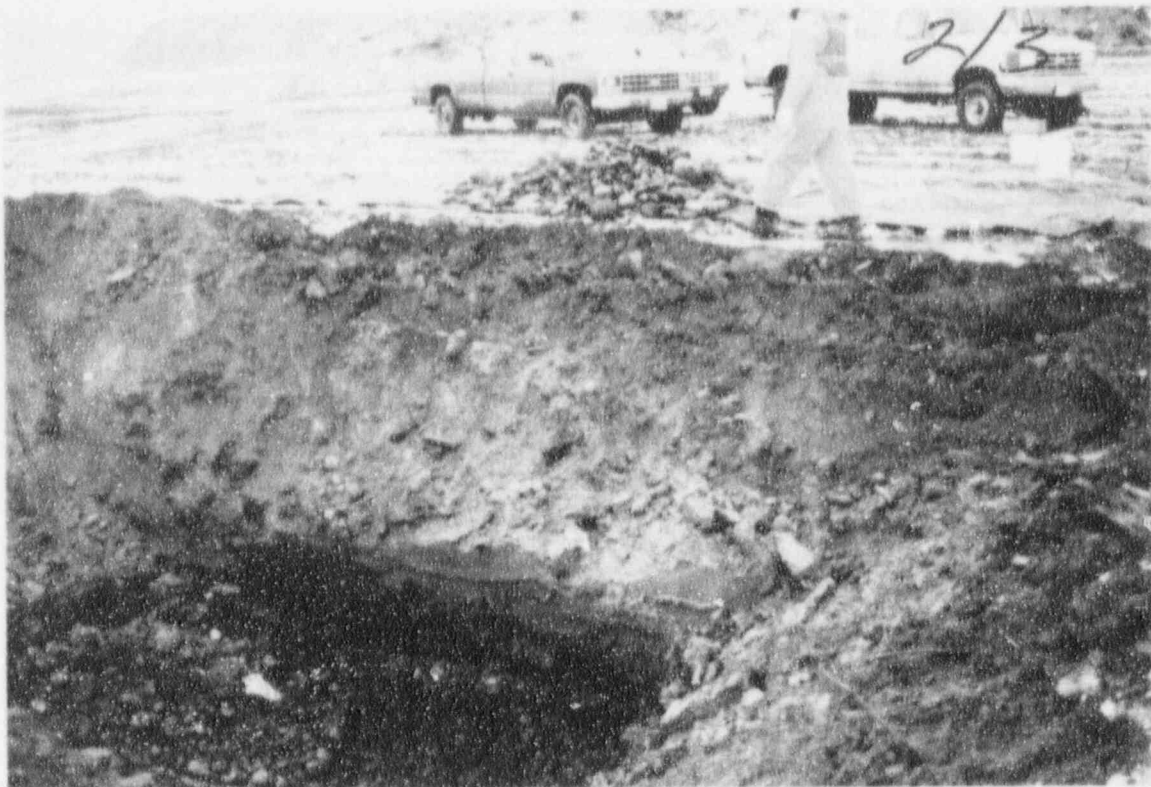
TP M-CF-27. About 4 feet of fill and wood trash overlying tailings. Bottom of the test pit is in gravels and cobbles.
