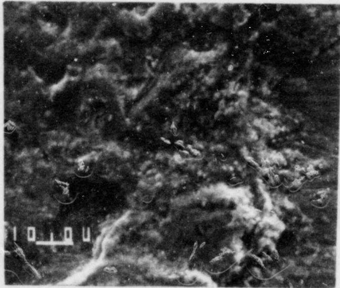
1000x Figure 24. SEM photograph of second "smeared" area on bolt.
