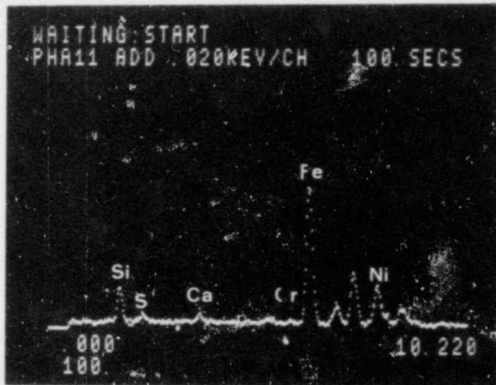
Figure 17. EDS scan of fibrous particle.
