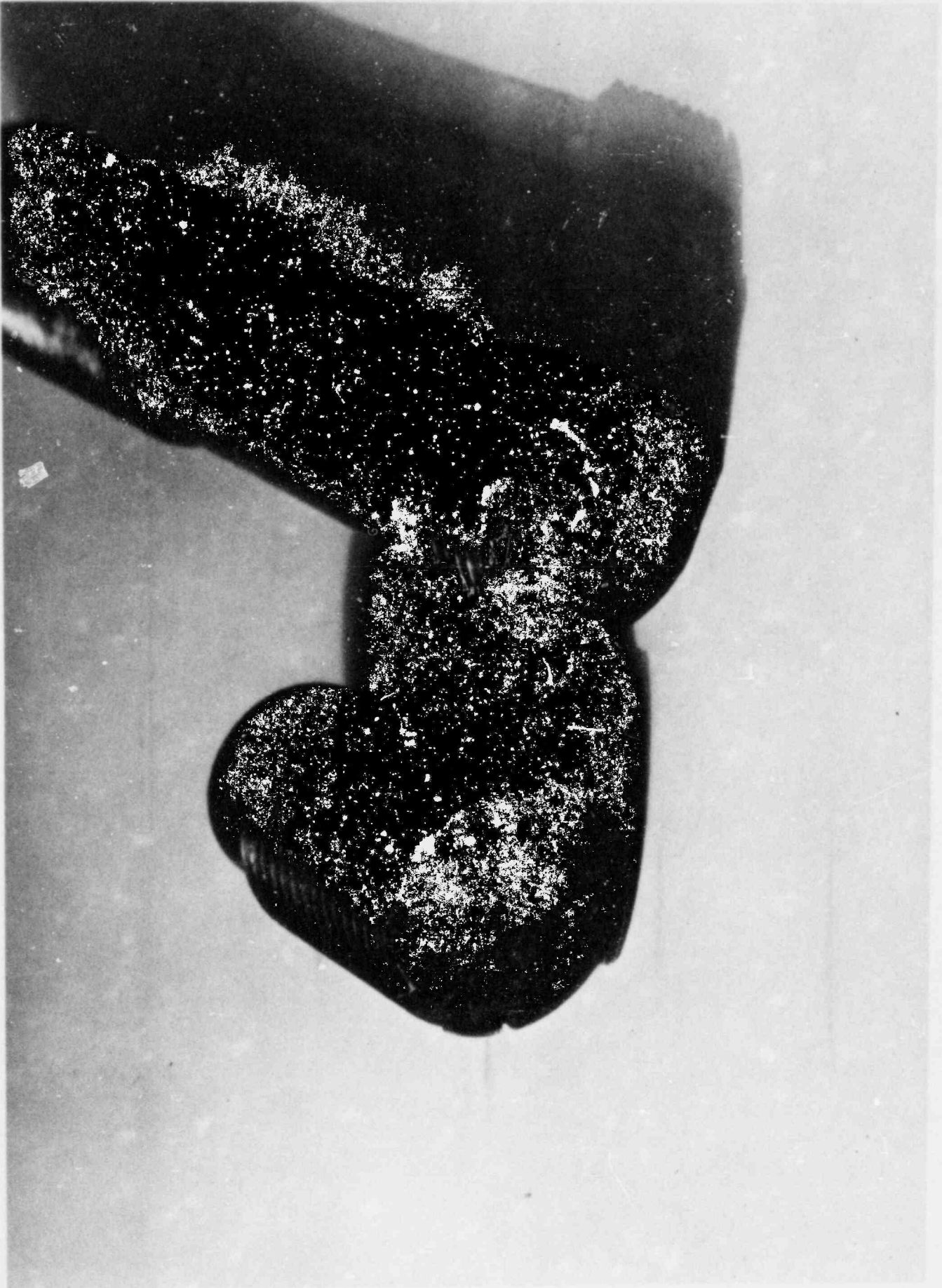
Figure 4. Frontal photograph of the fracture faces of the cracked bolt.
