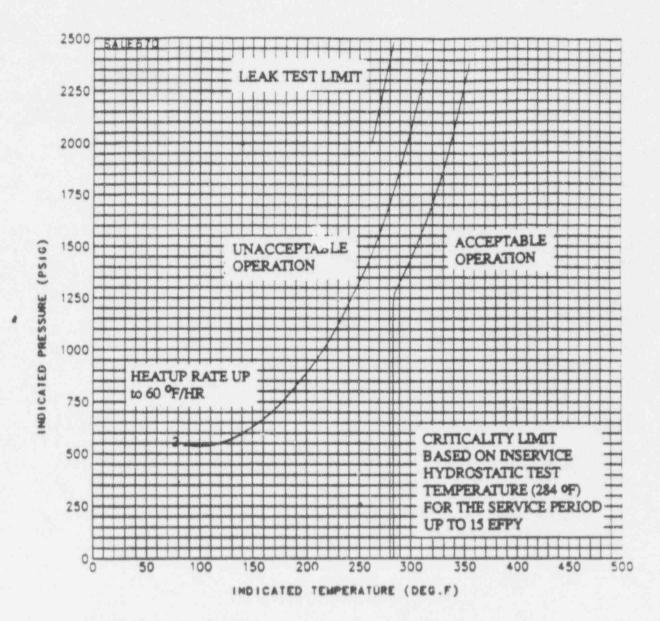
SALEM UNIT 2 REACTOR COOLANT SYSTEM HEATUP LIMITATIONS APPLICABLE FOR THE FIRST 15 EFPY WITH MAXIMUM HEATUP RATE OF 60 F/HR. CURVE CONTAINS NO MARGIN FOR INSTRUMENT ERROPS.
