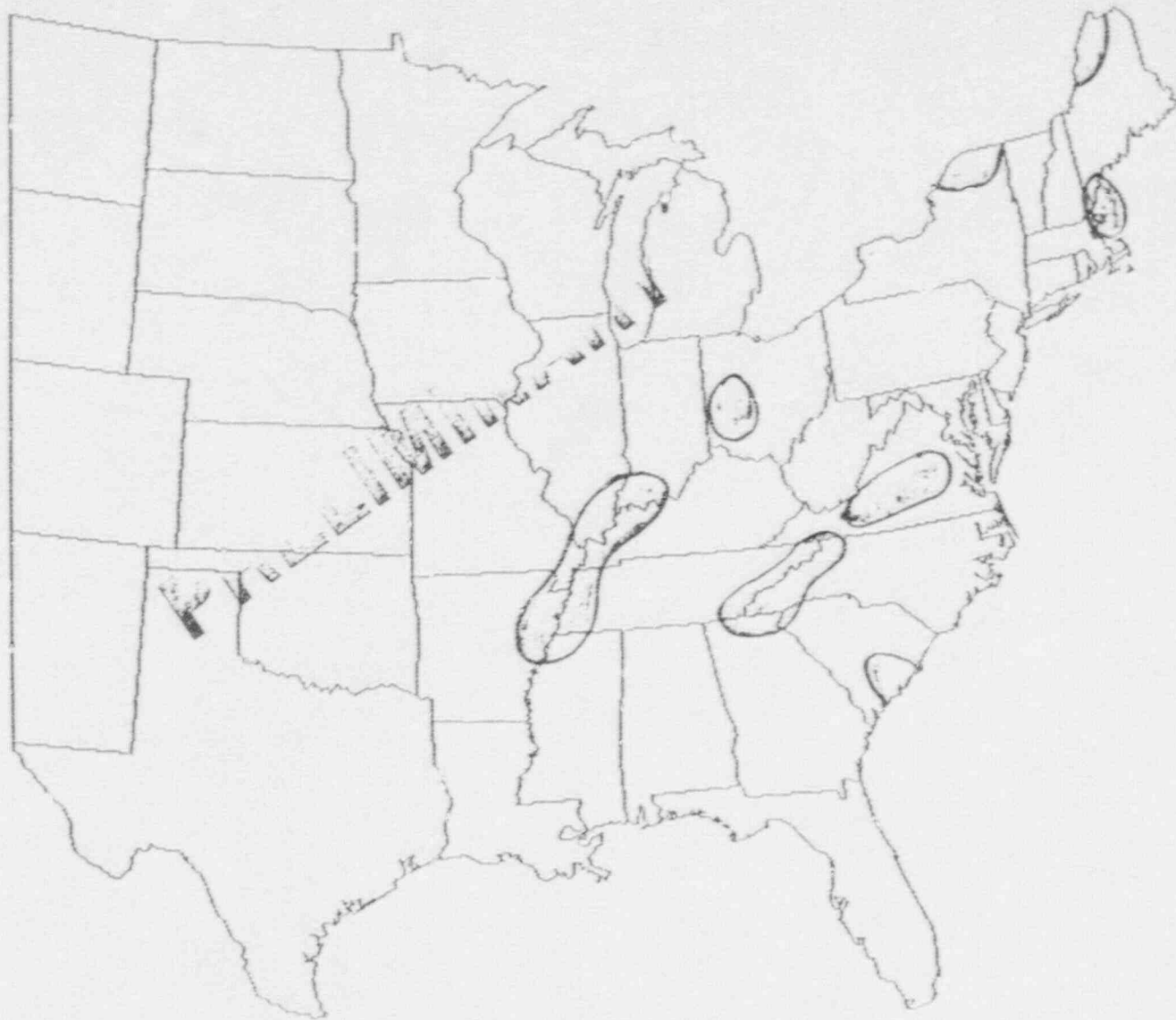
Figure 8-6 Areas in the EUS where the ALWR seismic risk may be greater than 10^{-6} per year for soil category S4 sites. Site-specific hazard assessments may be required for plants located in these areas.
