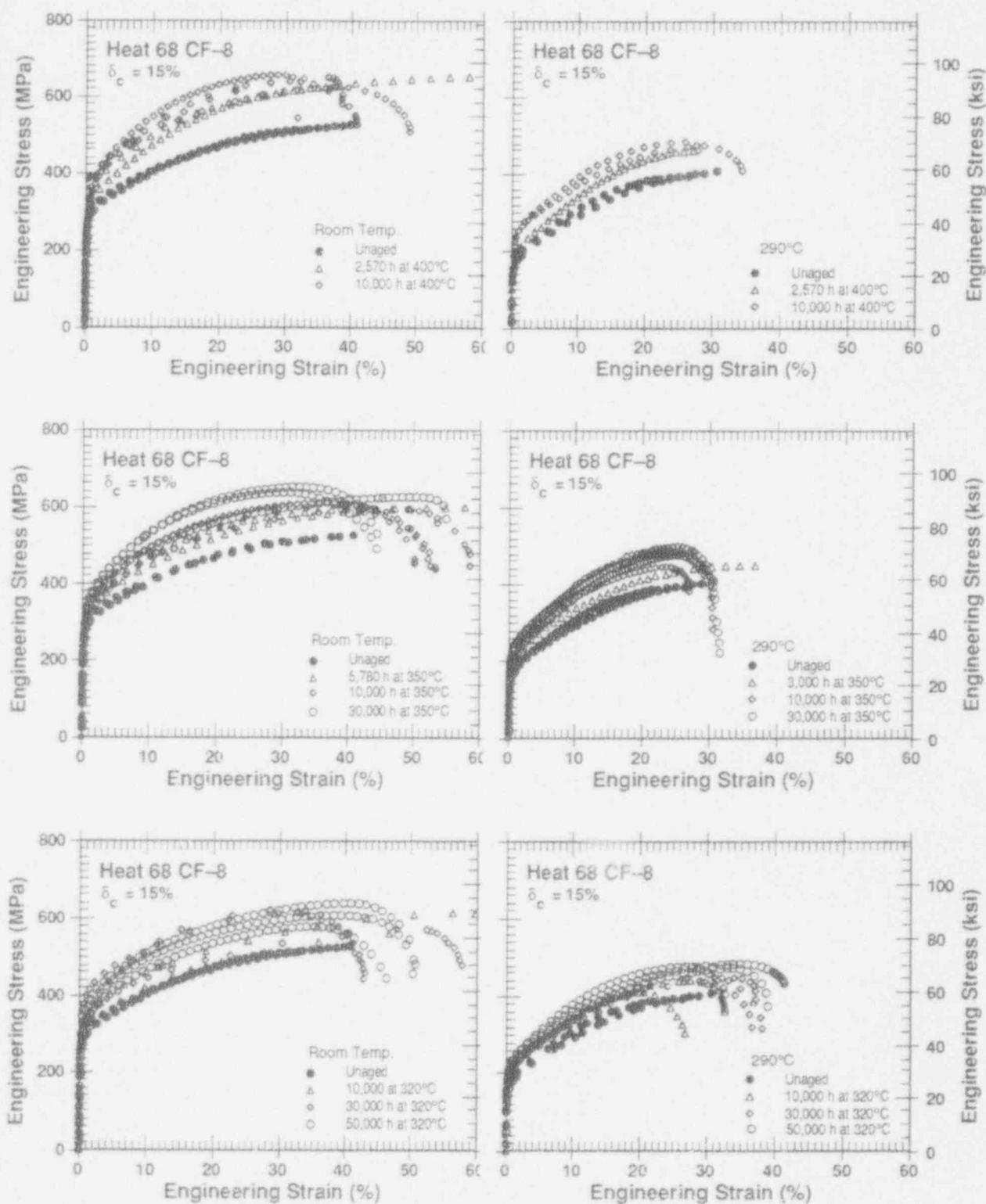
Figure 11. Effect of thermal aging on engineering stress vs. strain curves for Heat 68
