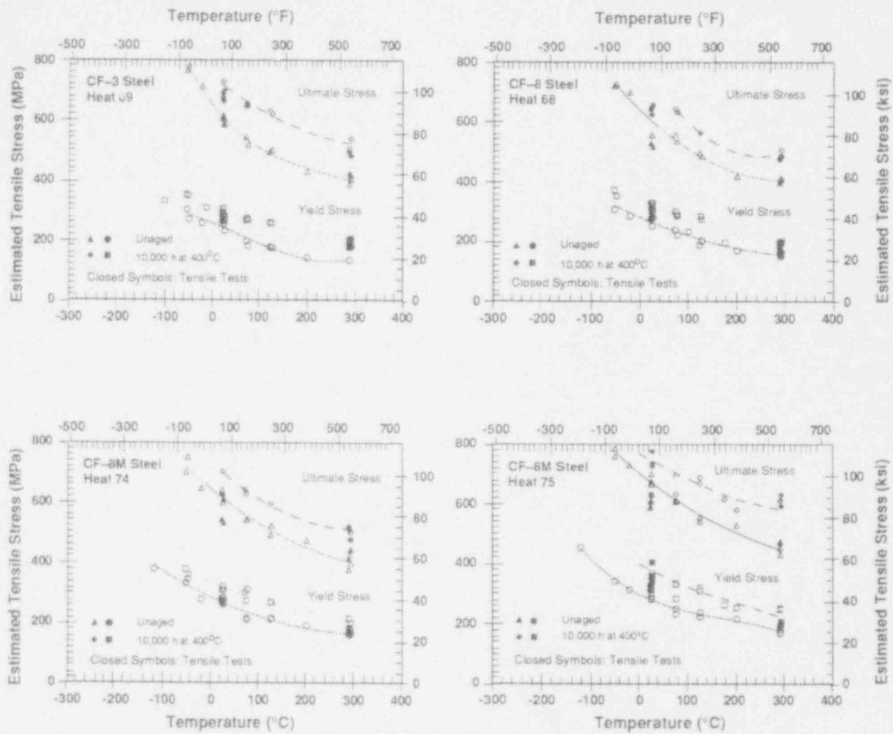
Figure 19. Values of yield and ultimate stress estimated from Charpy-impact data and those obtained from tensile tests for Heats 69, 68, 74, and 75
