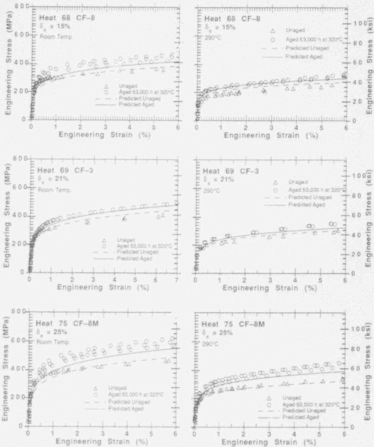
Figure 25. Engineering stress-vs.-strain curve at RT and 290°C, estimated from the chemical composition and initial tensile strength and determined experimentally for thermally aged CF-3, CF-8, and CF-8M steels
