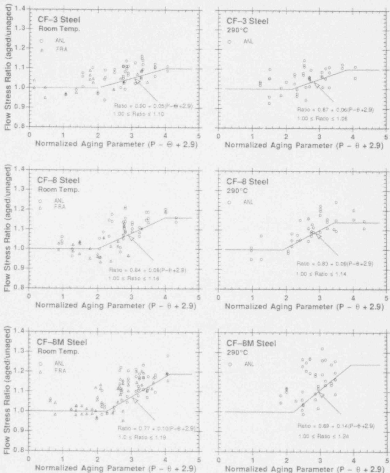
Figure 21. Flow stress ratio of aged cast stainless steels at RT and 290°C as a function of the normalized aging parameter. The solid lines represent correlations obtained by subtracting  $\sigma$  from the best fit curve.
