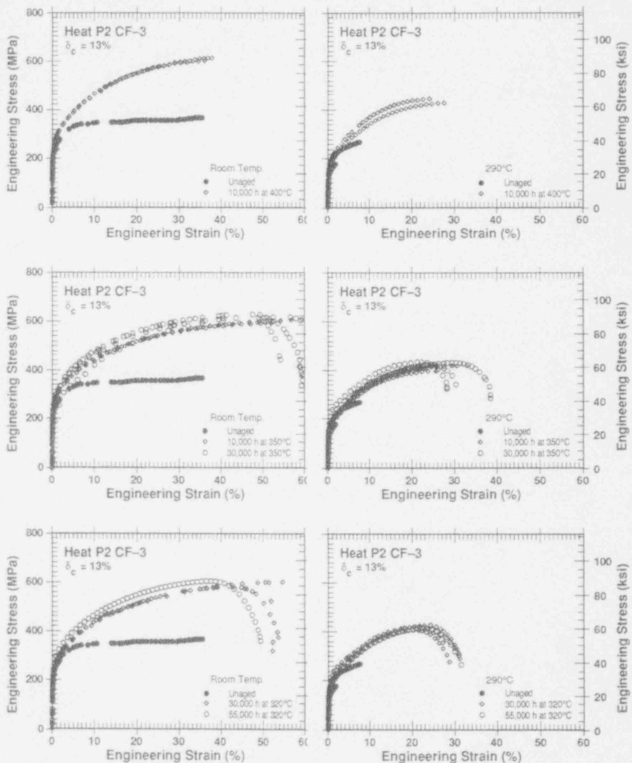
Figure 10. Effect of thermal aging on engineering stress vs. strain curves for Heat P2
