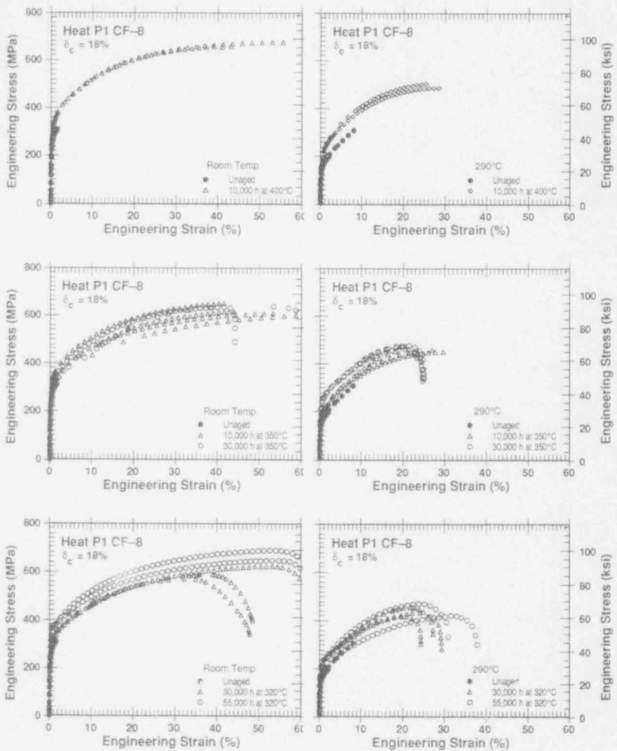
Figure 12. Effect of thermal aging on engineering stress vs. strain curves for Heat P1
