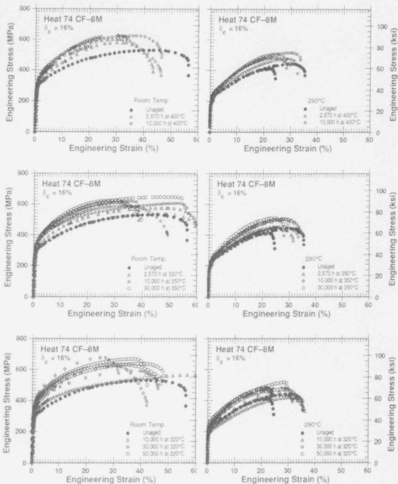
Figure 13. Effect of thermal aging on engineering stress vs. strain curves for Heat 74
