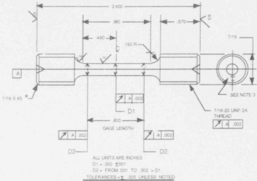
1. THE .800 INCH GAGE LENGTH TO HAVE UNIFORM SLOPE FROM MAX. DIA. D2 TO MIN. DIA. D1. UNIFORM SLOPE MUST NOT EXCEED .004 CHANGE IN DIA. PER 1 INCH CHANGE IN LENGTH.
