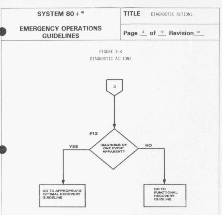
When the Diagnostic Actions are complete, a preliminary diagnosis should be apparent with an appropriate ORG available to be implemented (Reactor Trip Recovery is an ORG), or a preliminary diagnosis of one event is not possible and the FRG must be implemented.
