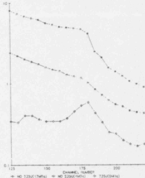
Fig 4 Interference in the 235 U 185.72 keV gamma-ray channels (163-192) due to 88 keV gamma-ray "double peaks" from 109 Cd sources with different activities
