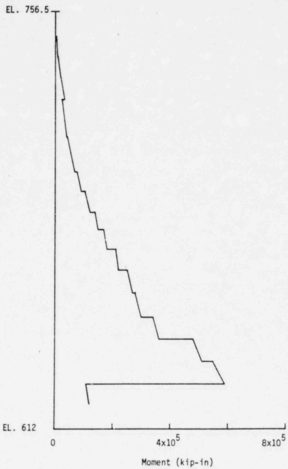
FIGURE 5-31. MOMENT IN STEEL CONTAINMENT IN X DIRECTION USING UPPER BOUND ESTIMATE OF SOIL SHEAR MODULUS
