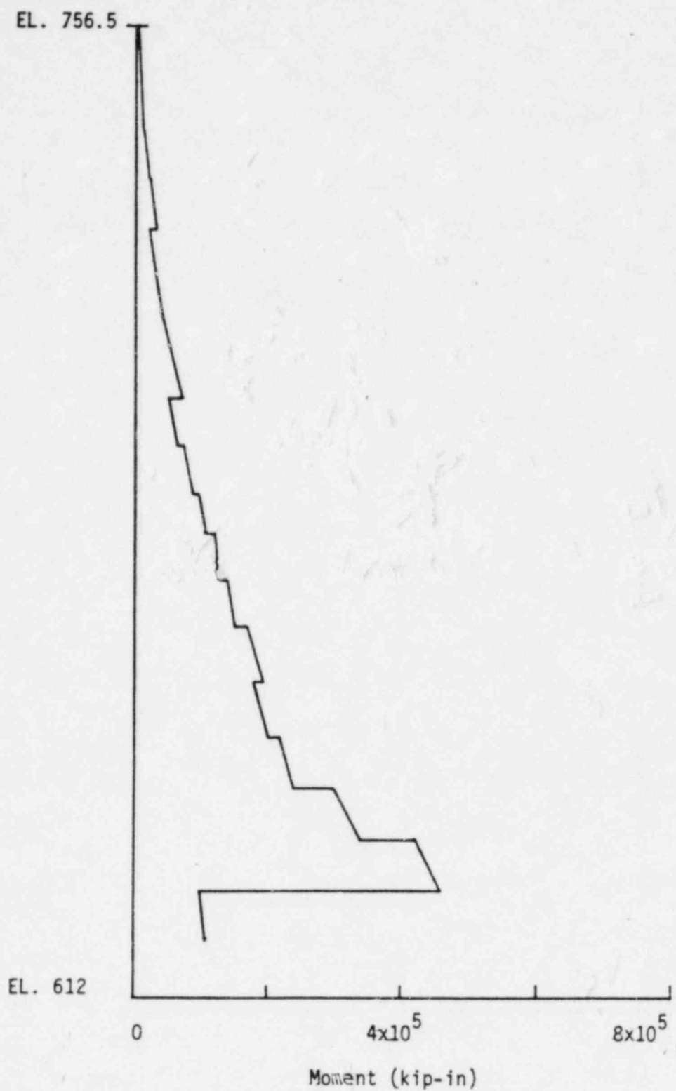
FIGURE 5-28. MOMENT IN STEEL CONTAINMENT IN Y DIRECTION USING BEST ESTIMATE OF SOIL SHEAR MODULUS
