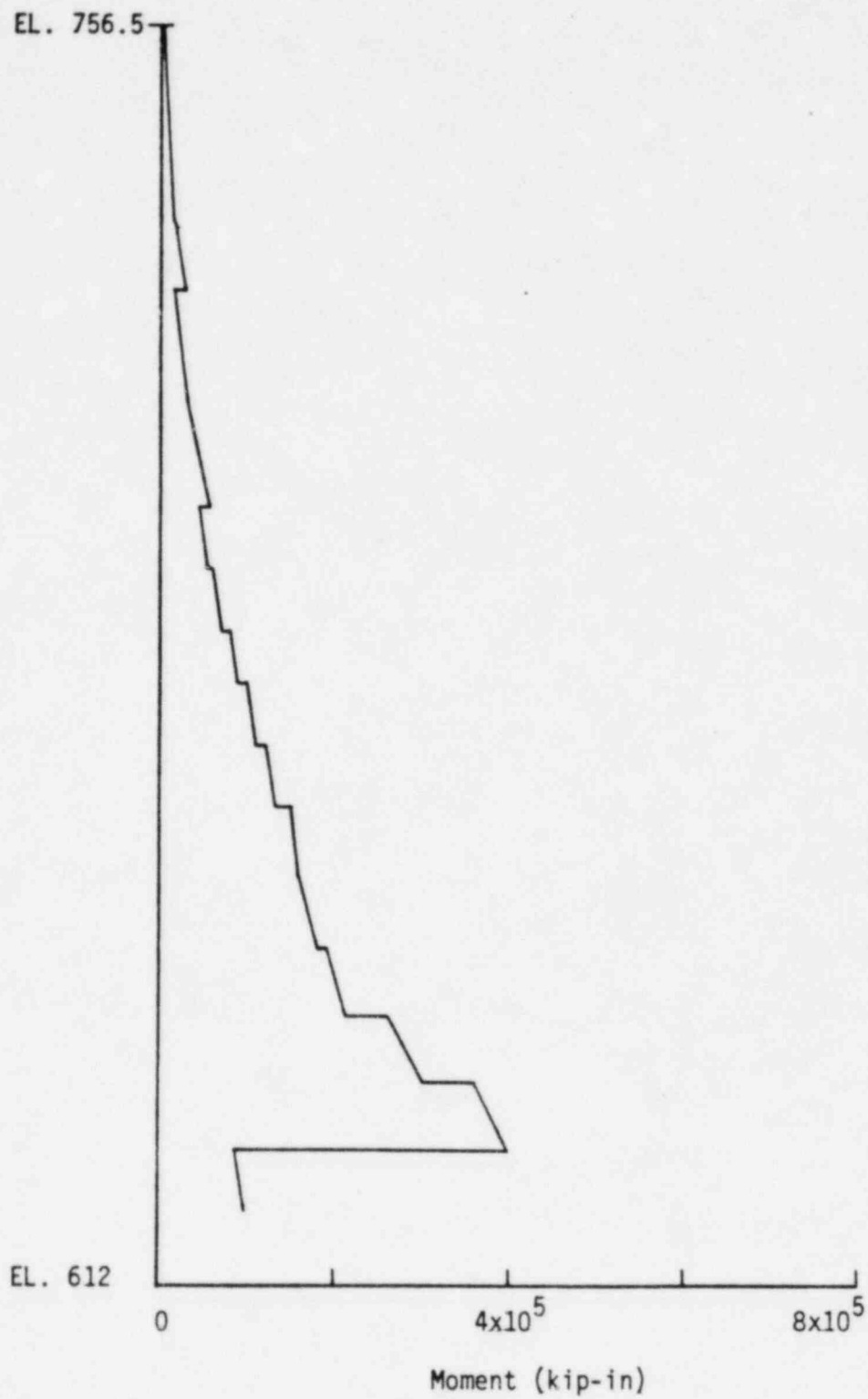
FIGURE 5-40. MOMENT IN STEEL CONTAINMENT IN Y DIRECTION USING LOWER BOUND ESTIMATE OF SOIL SHEAR MODULUS
